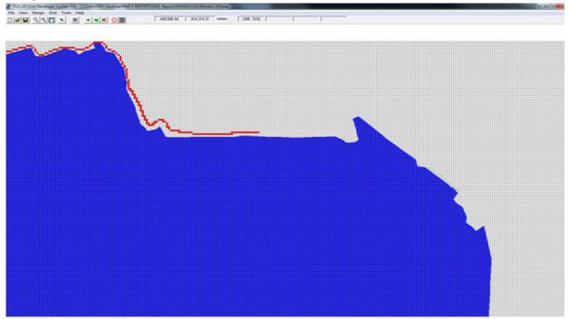
Figure 22. Screenshot showing how boundary grid elements are defined by line Elevation data was imported in the form of the DEM gathered through LiDAR. These elevation points in PTS format were extrapolated into the model, providing an elevation value for each grid element.
