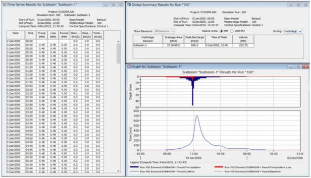
Figure 21. HEC-HMS simulation discharge results using Dr. Horritt's Method
