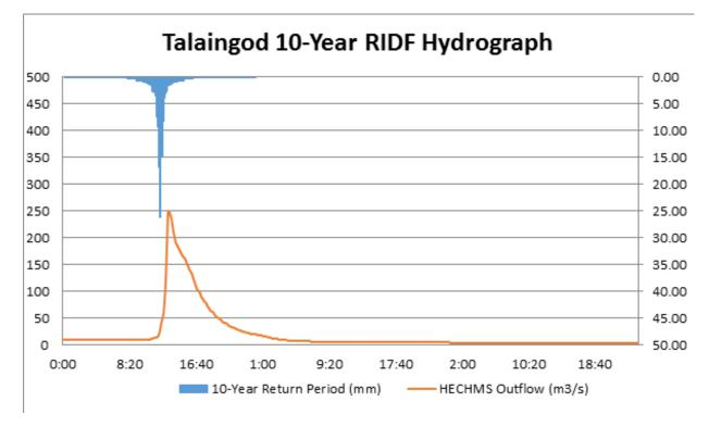
Figure 39. Outflow hydrograph generated using the Davao 10-Year RIDF inputted in HEC-HMS
