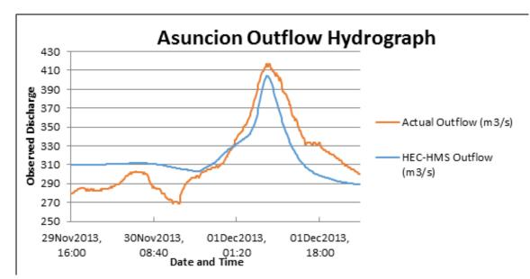
Figure 30. Outflow Hydrograph produced by the HEC-HMS model compared with observed outflow at Asuncion Bridge
