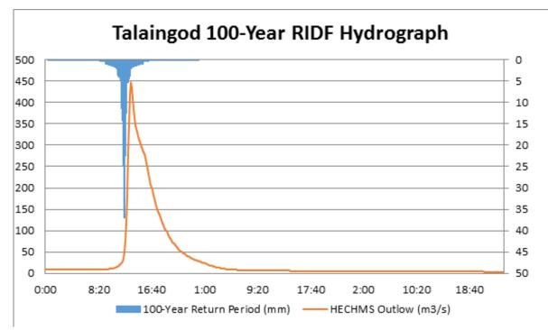
Figure 42. Outflow hydrograph generated using the Davao 100-Year RIDF inputted in HEC-  ${\rm HMS}$
