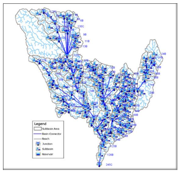
Figure 17. Tagum HEC-HMS Model domain generated by WMS
