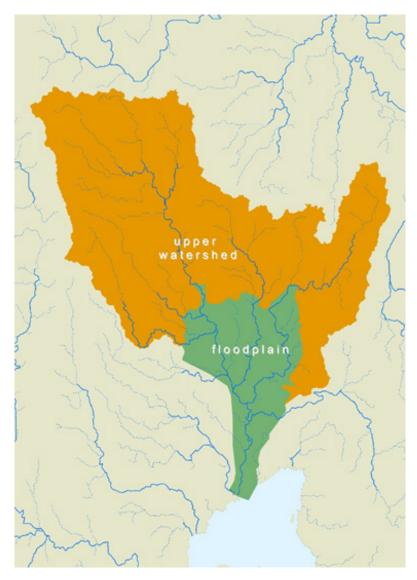
Figure 20. Delineation upper watershed for Tagum floodplain discharge computation
