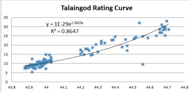
Figure 15. Water level vs. Discharge Curve for Nanaga Bridge, Talaingod, Davao del Norte
