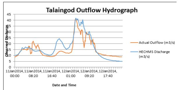
Figure 31. Outflow Hydrograph produced by the HEC-HMS model compared with observed outflow at Nanaga Bridge
