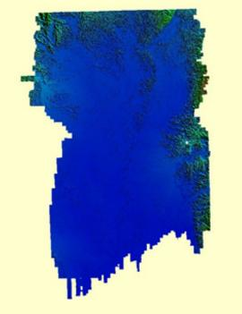
Figure 7. Digital Elevation Model (DEM) of the Tagum River Basin using Light Detection and Ranging (LiDAR) technology
