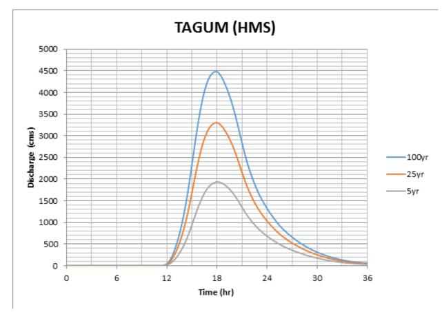
Figure 43. Outflow hydrograph generated for Tagum using the Malaybalay and Davao Stations' 5-, 25-, and 100-year Rainfall Intensity Duration Frequency (RIDF) in HEC-HMS
