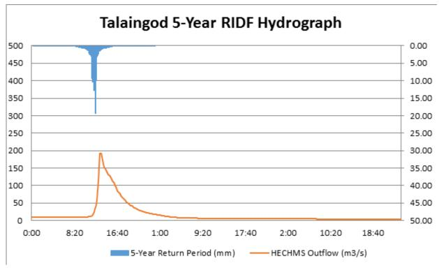
Figure 38. Outflow hydrograph generated using the Davao 5-Year RIDF inputted in HEC-HMS
