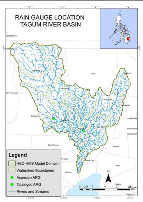
Figure 18. The location map of rain gauges used for the calibration of the Tagum HEC-HMS model
