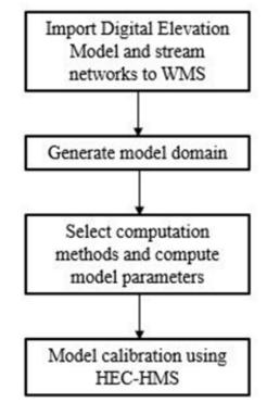
Figure 16. The Rainfall-Runoff Basin Model Development Scheme
