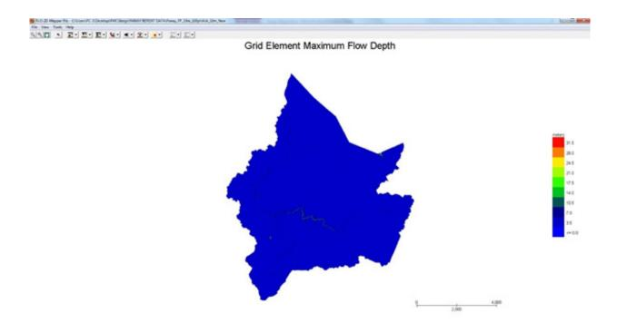
Figure 28. Tagum floodplain generated flow depth map using FLO-2D Mapper
