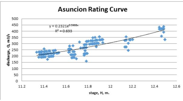
Figure 14. Water level vs. Discharge Curve for Mahayahay Bridge, Asuncion, Davao del Norte
