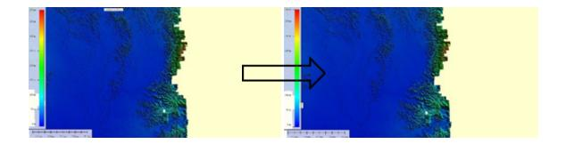
Figure 8. The 1-meter resolution LiDAR data resampled to a 10-meter raster grid in GIS software to ensure that values are properly adjusted.
