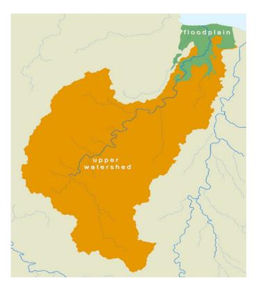
Figure 18. Delineation of upper watershed for Iponan floodplain discharge computation
