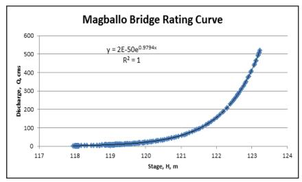
Figure 16. Water level vs. Discharge Curve for Magballo Bridge
