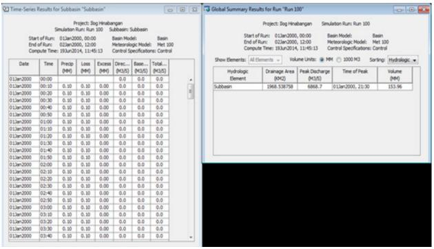
Figure 22. HEC-HMS simulation discharge results using Dr. Horritt's Method
