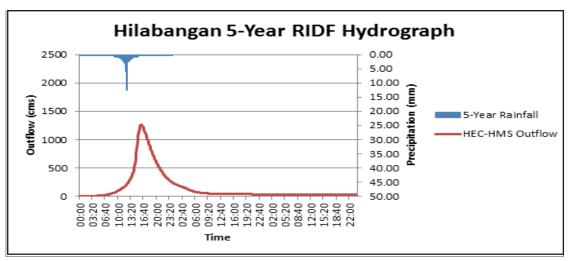
Figure 34. Hilabangan Bridge outflow hydrograph generated using the Negros 5-Year RIDF inputted in WMS and HEC-HMS Basin Model.
