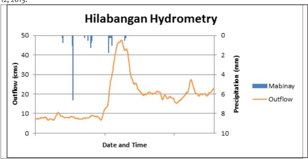
Figure 10. Hilabangan Bridge rainfall and outflow data used for modeling.
