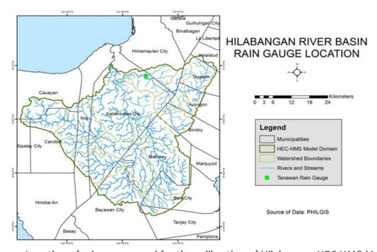
Figure 19. Location of rain gauge used for the calibration of Hilabangan HEC-HMS Model.
