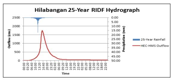
Figure 36. Hilabangan Bridge outflow hydrograph generated using the Negros 25-Year RIDF inputted in WMS and HEC-HMS Basin Model.
