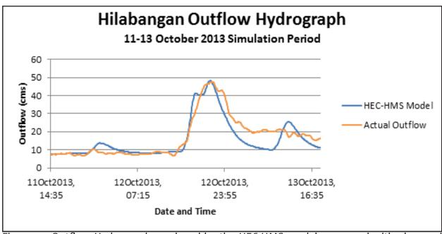
Figure 31. Outflow Hydrograph produced by the HEC-HMS model compared with observed outflow.
