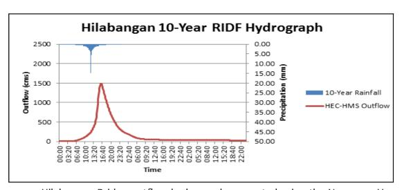
Figure 35. Hilabangan Bridge outflow hydrograph generated using the Negros 10-Year RIDF inputted in WMS and HEC-HMS Basin Model.
