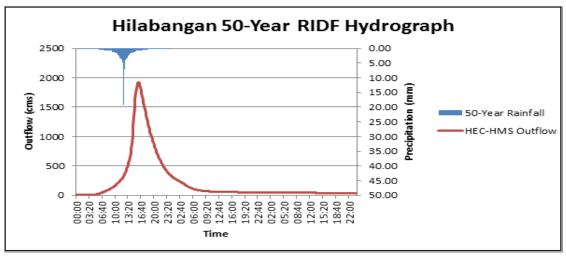
Figure 37. Hilabangan Bridge outflow hydrograph generated using the Negros 50-Year RIDF inputted in WMS and HEC-HMS Basin Model.
