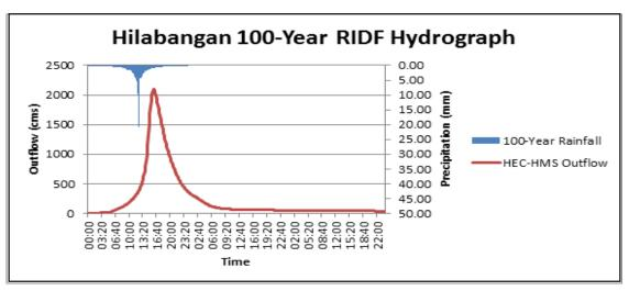
Figure 38. Hilabangan Bridge outflow hydrograph generated using the Negros 50-Year RIDF inputted in WMS and HEC-HMS Basin Model.
