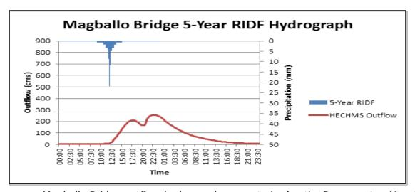
Figure 39. Magballo Bridge outflow hydrograph generated using the Dumaguete 5-Year RIDF inputted in WMS and HEC-HMS Basin Model.
