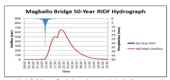
Figure 42. Magballo Bridge outflow hydrograph generated using the Dumaguete 50-Year RIDF inputted in WMS and HEC-HMS Basin Model.
