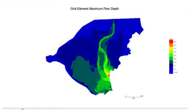
Figure 29. Hilabangan floodplain generated flow depth map using Flo-2D Mapper
