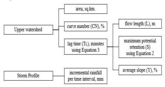
Figure 20. Different data needed as input for HEC-HMS discharge simulation using Dr. Horritt's recommended hydrology method.
