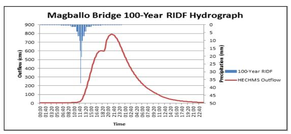
Figure 43. Magballo Bridge outflow hydrograph generated using the Dumaguete 100-Year RIDF inputted in WMS and HEC-HMS Basin Model
