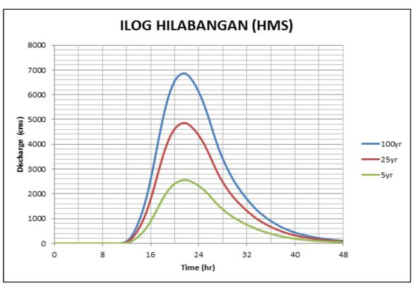
Figure 44. Outflow hydrograph generated for Ilog Hilabangan using the Iloilo Station 5-, 25-, 100-Year RIDF in HEC-HMS
