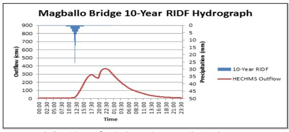
Figure 40. Magballo Bridge outflow hydrograph generated using the Dumaguete 10-Year RIDF inputted in WMS and HEC-HMS Basin Model.
