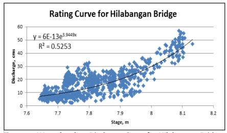
Figure 15. Water level vs. Discharge Curve for Hllabangan Bridge
