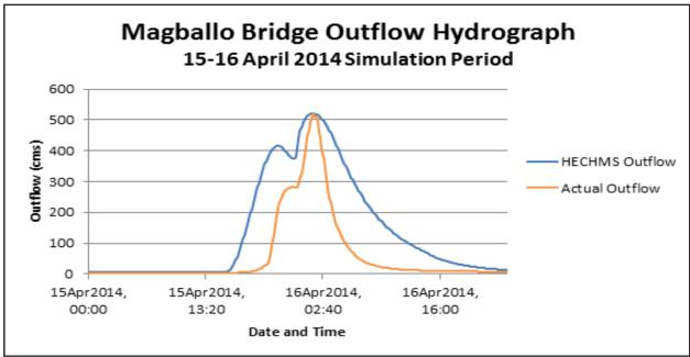
Figure 32. Outflow Hydrograph produced by the HEC-HMS model compared with observed outflow.
