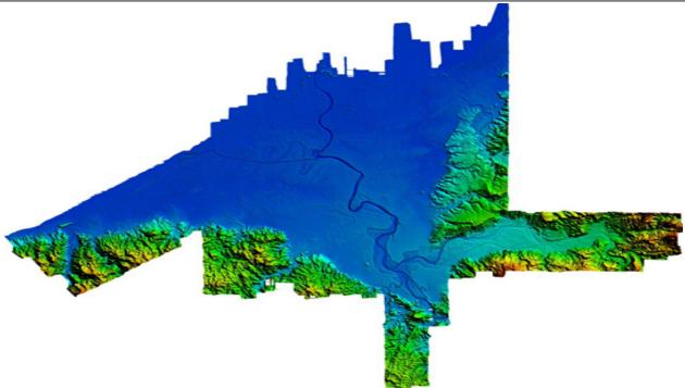
Figure 7. Digital Elevation Model (DEM) of the Hilabangan River Basin using Light Detection and Ranging (LiDAR) technology
