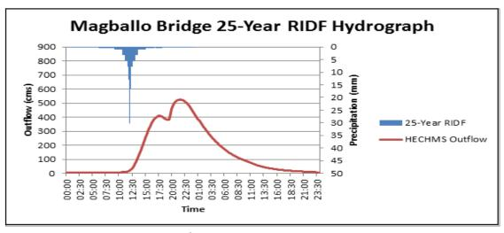
Figure 41. Magballo Bridge outflow hydrograph generated using the Dumaguete 25-Year RIDF inputted in WMS and HEC-HMS Basin Model.
