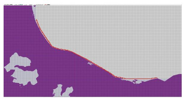
Figure 20. Screenshot showing how boundary grid elements are defined by line
