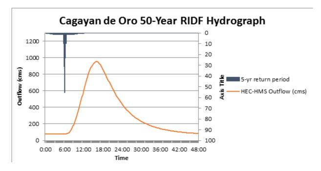
Figure 33. Outflow hydrograph generated using the Lumbia 50-Year RIDF inputted in HEC-  ${\rm HMS}$
