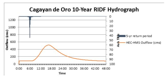
Figure 31. Outflow hydrograph generated using the Lumbia 10-Year RIDF inputted in HEC-HMS
