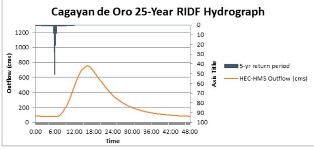
Figure 32. Outflow hydrograph generated using the Lumbia 25-Year RIDF inputted in HEC-HMS.
