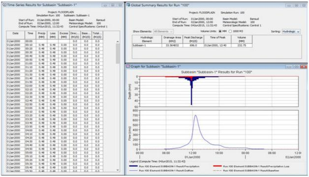
Figure 19. HEC-HMS simulation discharge results using Dr. Horritt's Method 3.3.2.3 Discharge validation against other estimates
