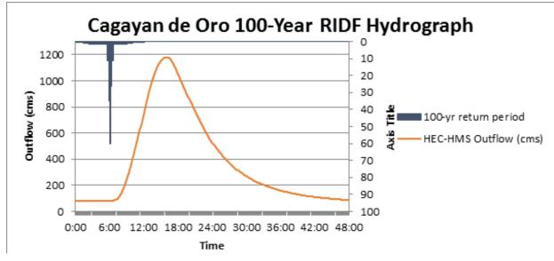
Figure 34. Outflow hydrograph generated using the Lumbia 100-Year RIDF inputted in HEC-HMS
