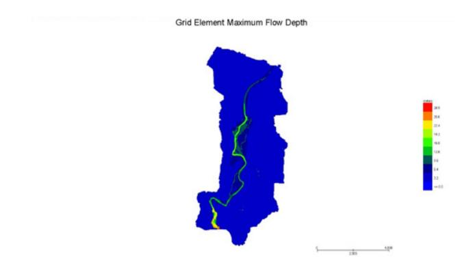
Figure 26. Cagayan de Oro floodplain generated flow depth map using FLO-2D Mapper
