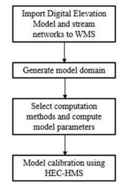
Figure 14. The Rainfall-Runoff Basin Model Development Scheme
