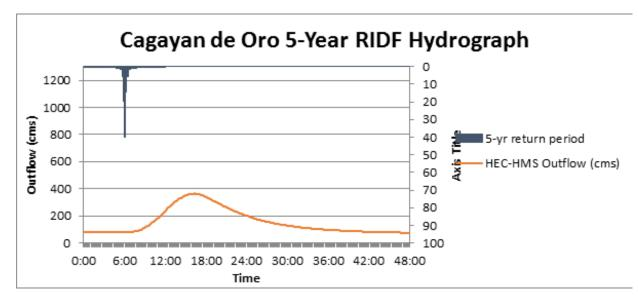
Figure 30. Outflow hydrograph generated using the Lumbia 5-Year RIDF inputted in HEC-HMS
