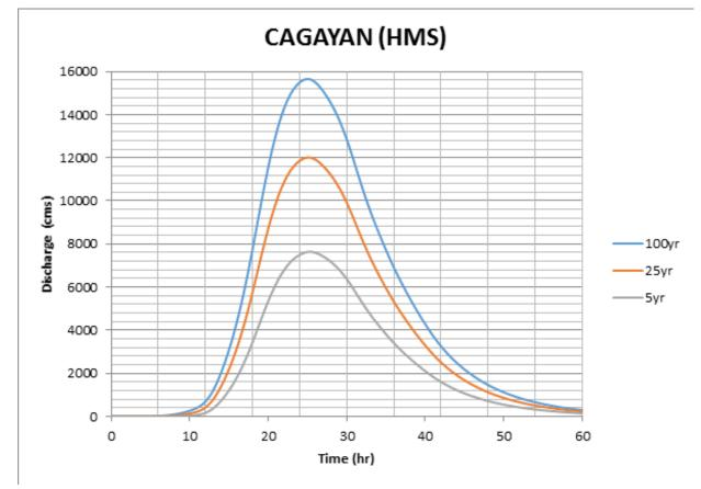
Figure 35. Outflow hydrograph generated for Cagayan de Oro using the Lumbia 5-, 25-, and
