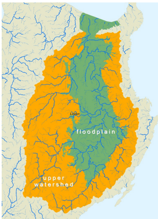
Figure 28. Delineation of upper watershed for Cagayan floodplain discharge computation
