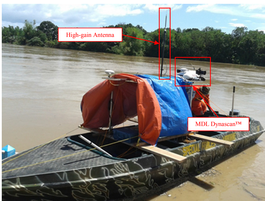
Figure 16. MDL Dynascan™ installed on one end of the boat for the river bank profile surveys of Pampanga River
