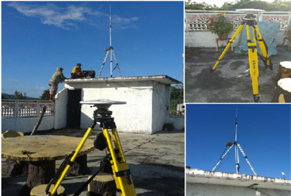
Figure 13. RTK Base set-up in Brgy. Cupang Arayat, Pampanga
