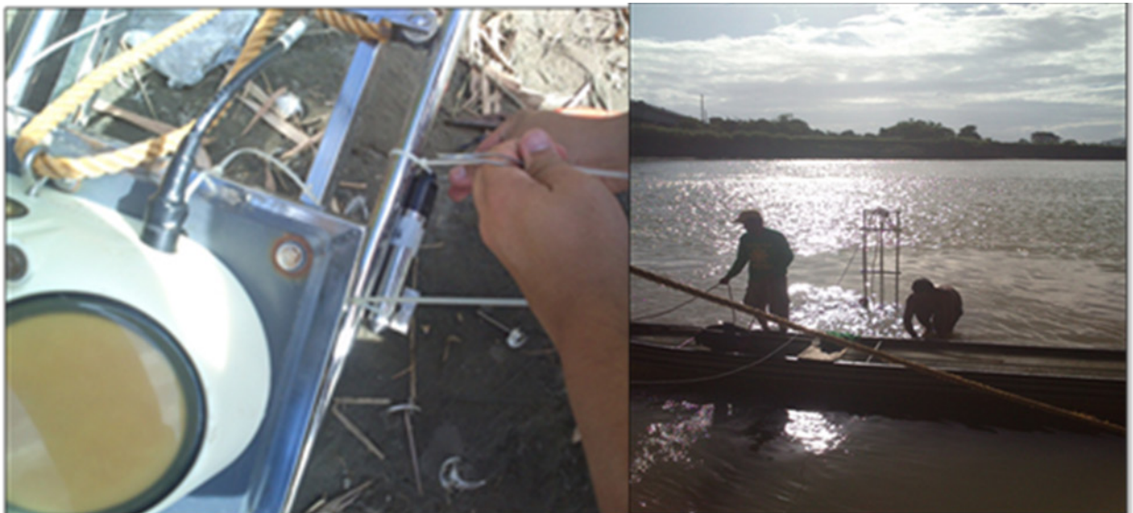
Figure 32. ADCP set up and deployment Site in Brgy. Camba, Arayat, Pampanga
