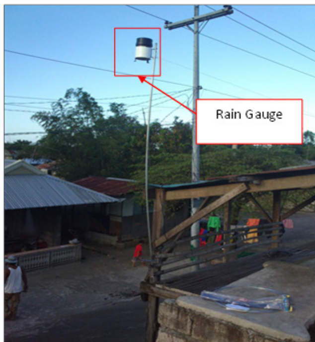
Figure 34. Rain Gauge deployed in Brgy. Camba, Arayat, Pampanga
