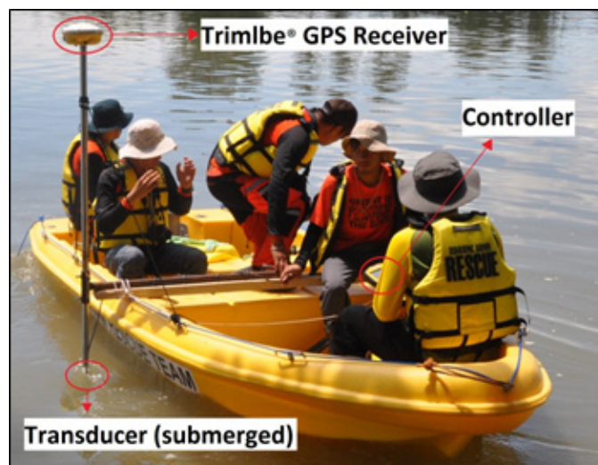
Figure 22. Bathymetric survey setup
