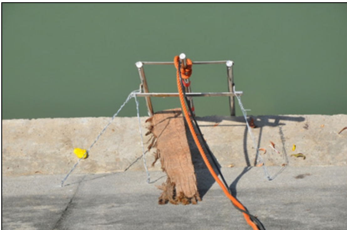
Figure 37. The Acoustic Doppler Current Profiler with depth gauge deployed along Dicalungan Bridge, Ampatuan, Maguindanao Cotabato
