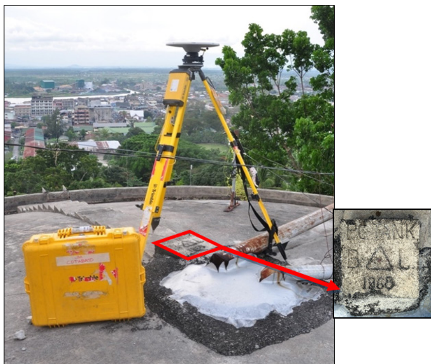
Figure 12. Static GNSS observation at MGD-2 on top of the PC Hill Compound water tank in Cotabato City
