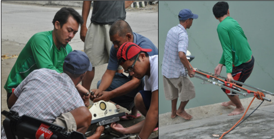
Figure 36. Deployment of ADCP with Depth Gauge on the bank of Mindoro River in Dicalungan Bridge, Ampatuan, Maguindanao Cotabato
