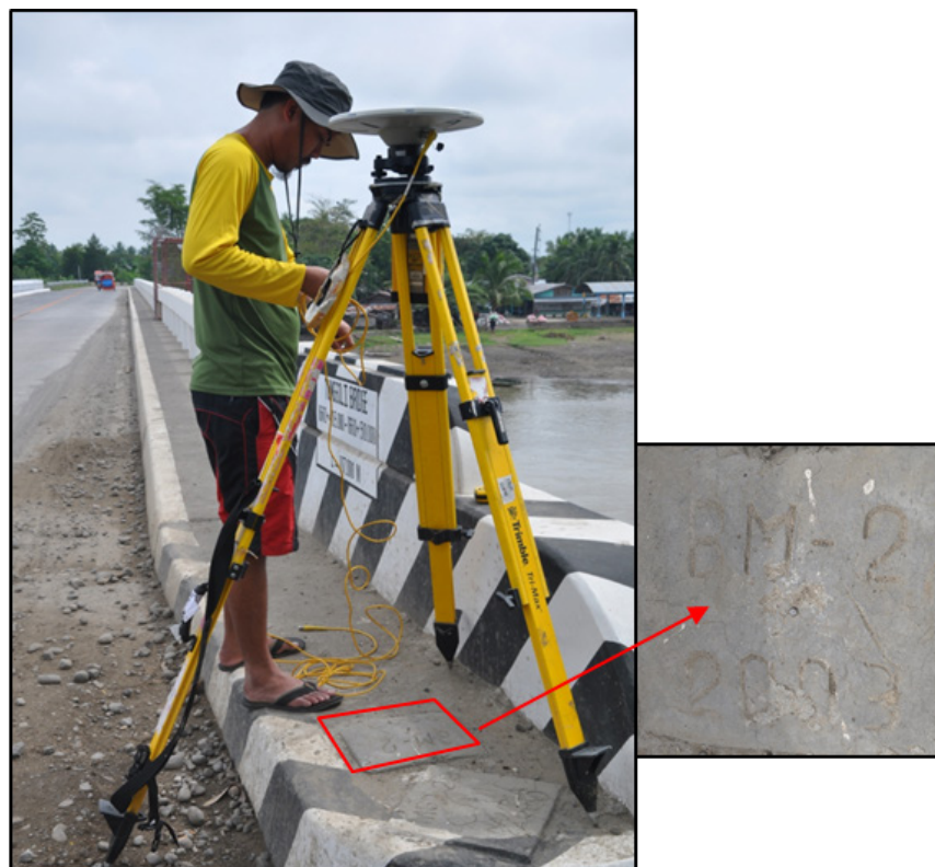
Figure 16. Static GNSS observation at BM-2 at Tunggol Bridge in Datu Montawal, Maguindanao
