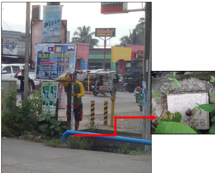
Figure 18. Differential levelling survey at IBM 58 in Brgy. Poblacion, Kabacan, Cotabato
