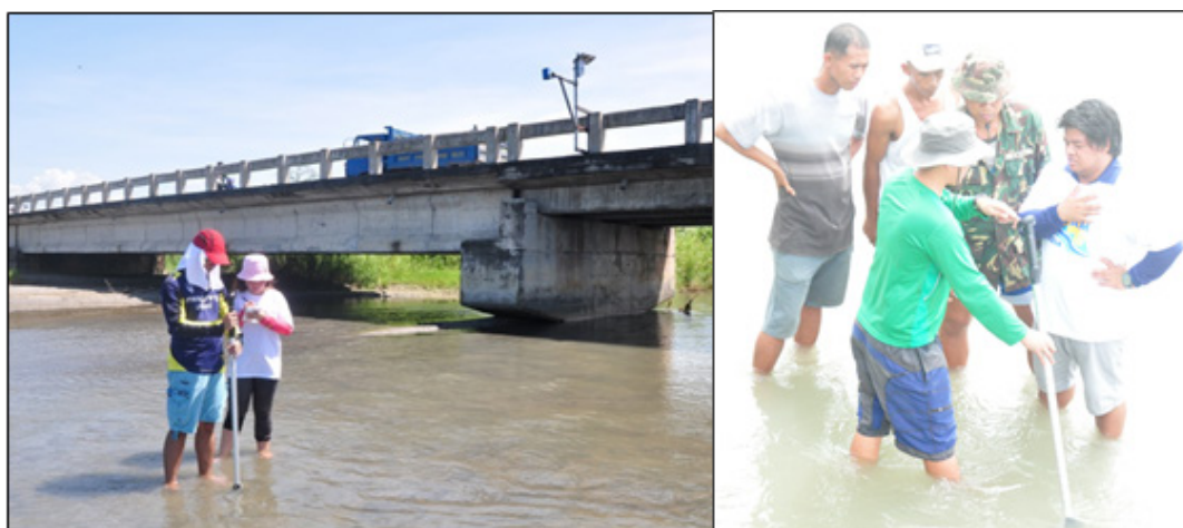
Figure 49. Flow measurement in Kalawag Bridge in Isulan, Sultan Kudarat on December 13-19, 2013 survey (A) and on July 1-15, 2014 survey (B) using digital flow meter.
