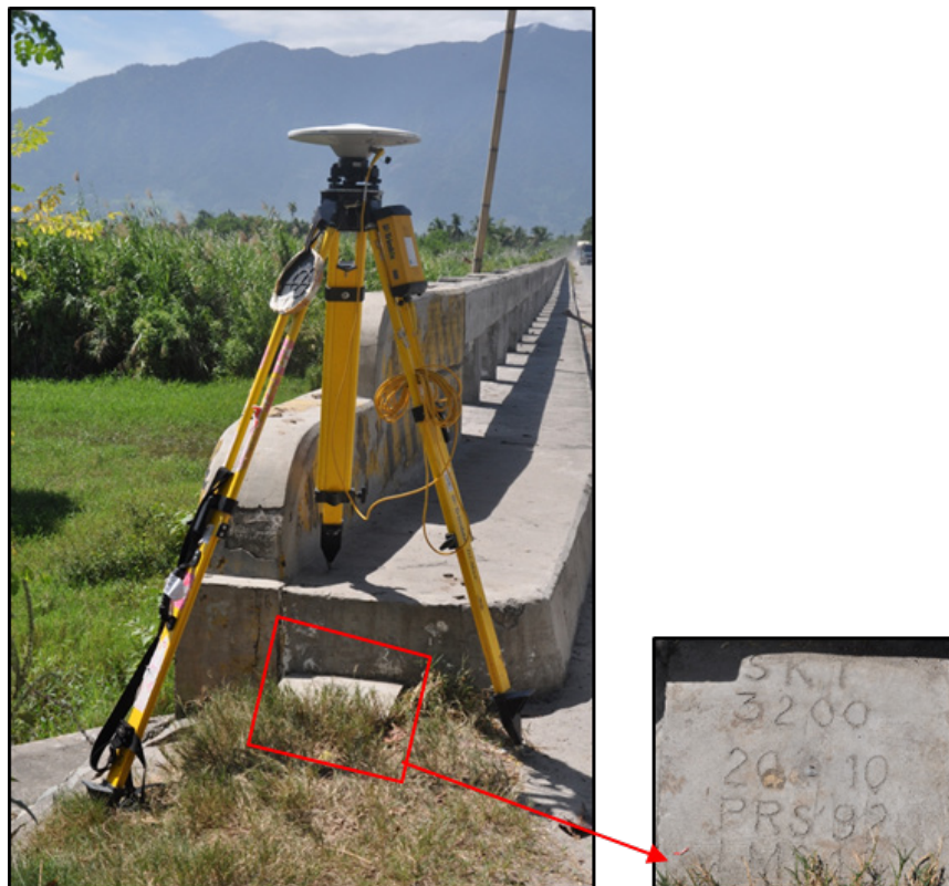
Figure 15. Static GNSS observation at SKT-3200 at Kalawag Bridge Isulan, Sultan Kudarat
