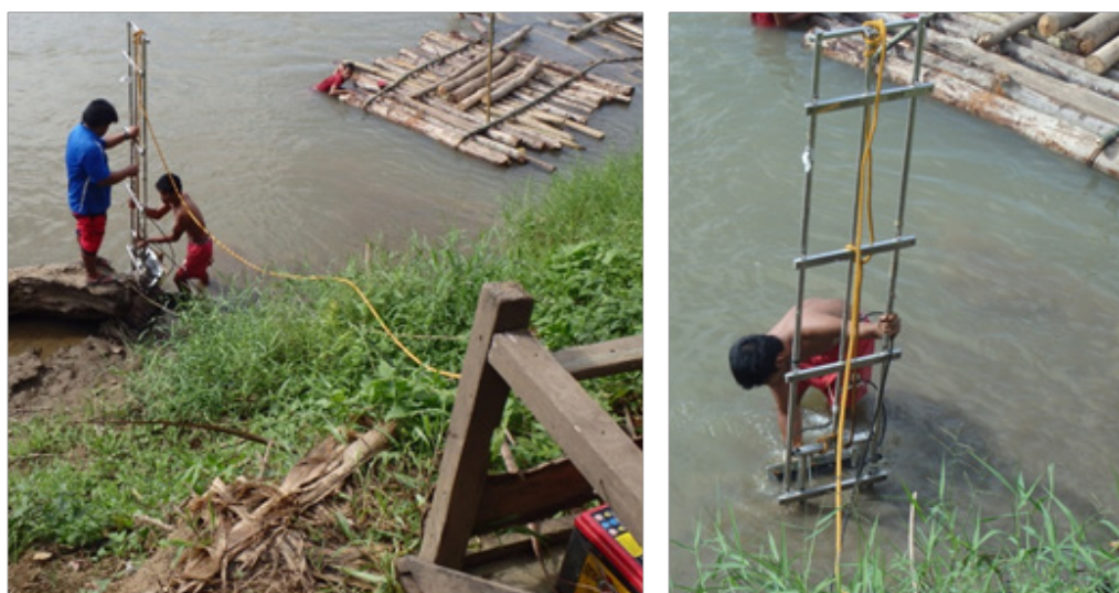
Figure 30. Deployment of ADCP with depth gauge in Lumayong (Carmen) Bridge, Brgy. Kaya, Kabacan, North Cotabato
