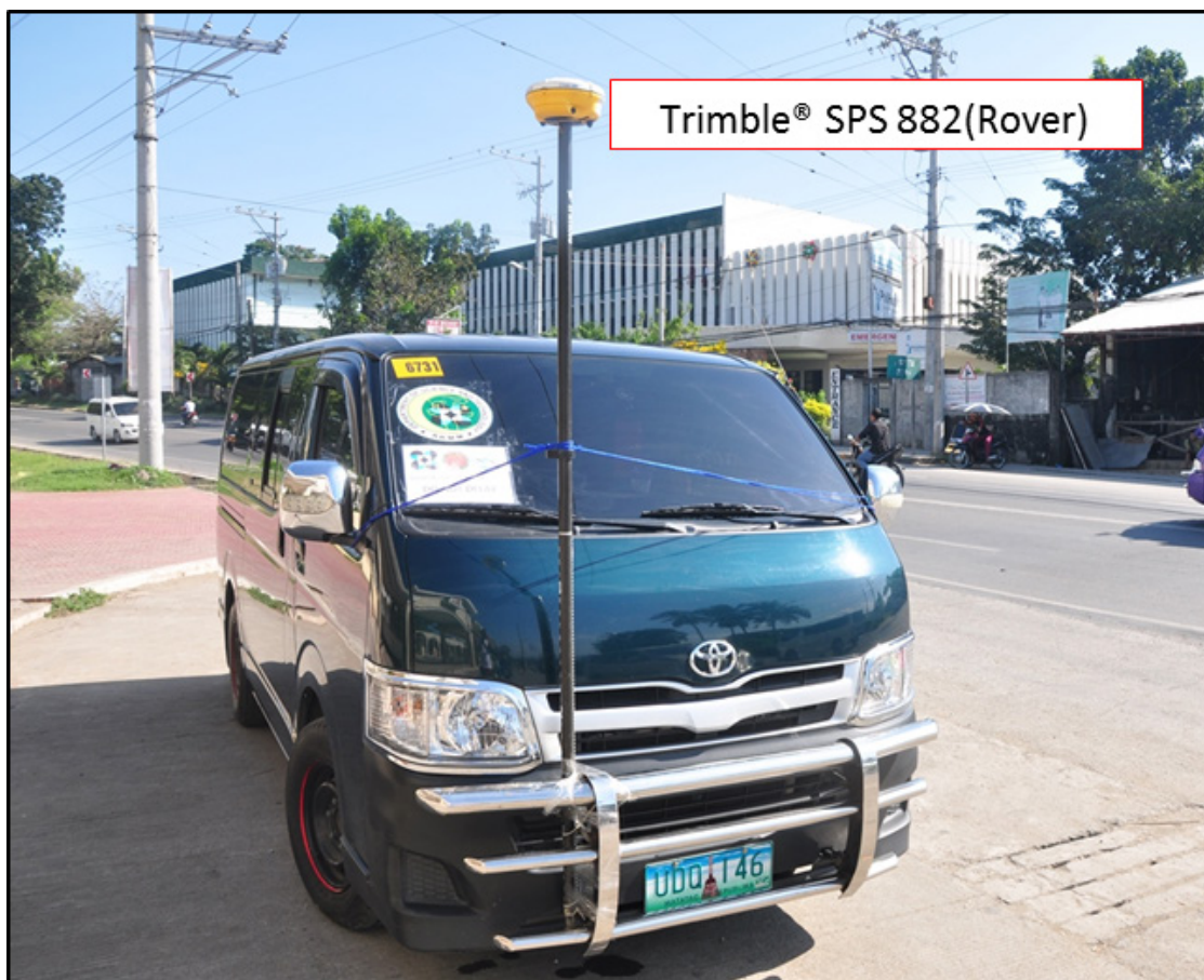
Figure 20. Validation Points Acquisition Survey
