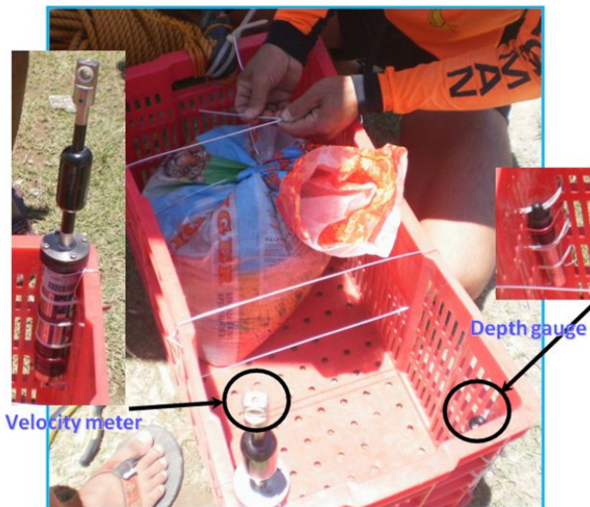
Figure 26. Setup of the sensors (velocity meter and depth gauge)
