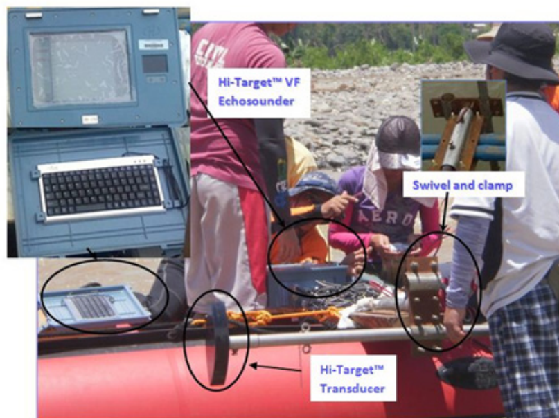
Figure 20. Setup of the bathymetric survey instrument on a rubber boat
