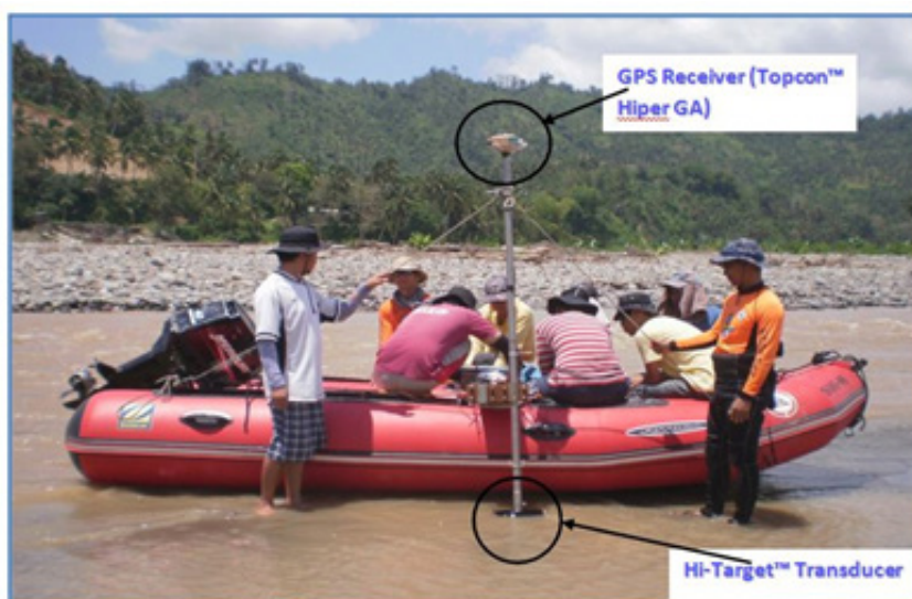
Figure 21. Another view of the single-beam echo sounder setup in PCG rubber boat with PCG personnel
