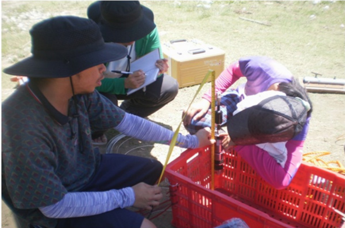
Figure 27. Measurement of the velocity meter offset prior deployment
