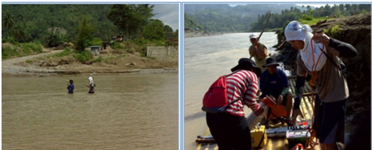
Figure 24. Alternative methods of acquiring bathymetric data in shallow areas (upstream of Mandulog River) using Topcon™ digital level and Nikon™ total station
