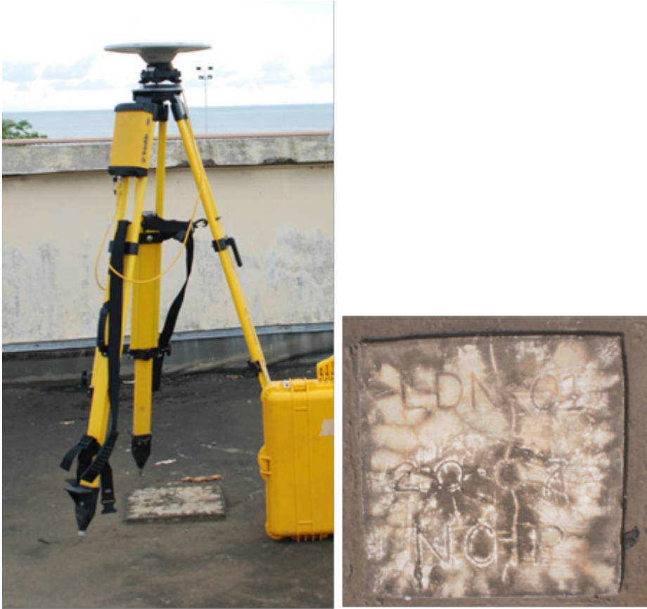
Figure 12. Recovered NAMRIA horizontal control point (LDN-01, see inset) at the PPA premises, Iligan City
