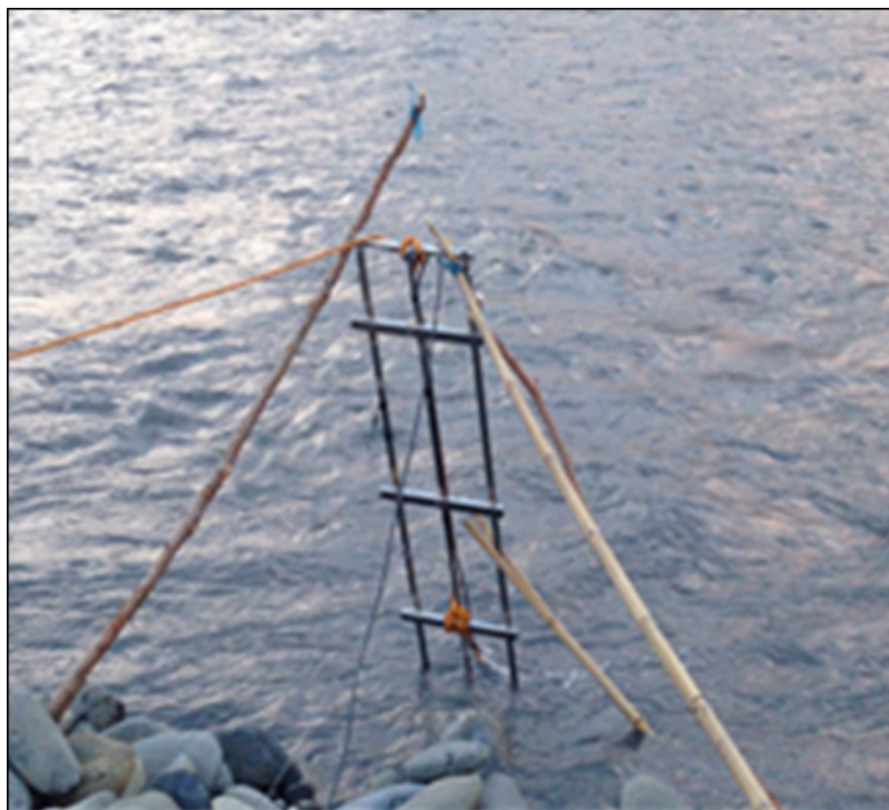
Figure 19. ADCP and Depth Gauge deployed in Brgy. Villa Cerveza
