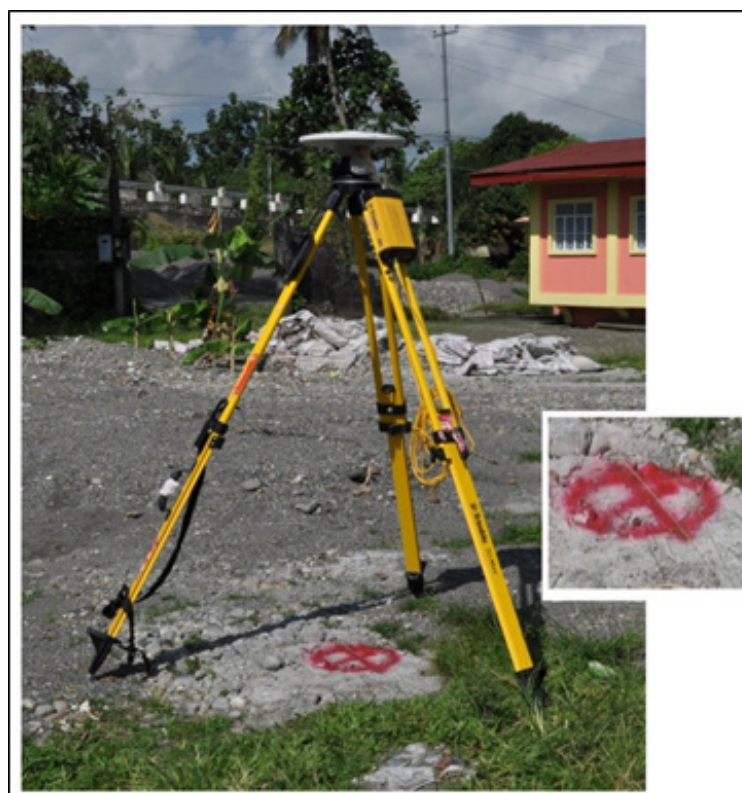
Figure 14. Base set-up at a control point at Brgy. Barcenaga, Naujan, Oriental Mindoro
