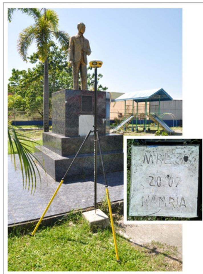
Figure 12. Static GNSS observation at MRE-32 at Victoria, Oriental Mindoro
