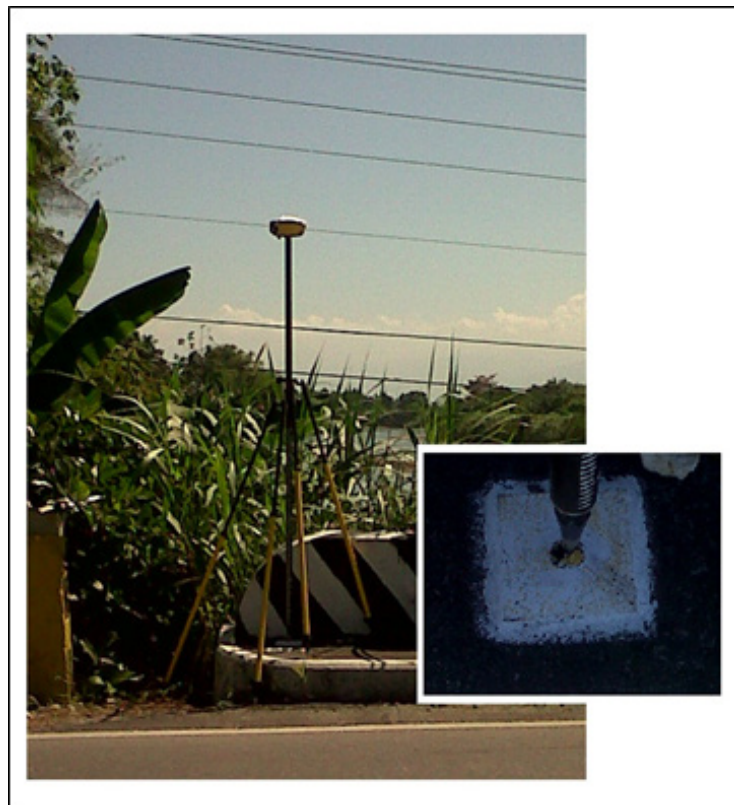
Figure 13. Static observation at MR-178 at Pangalaan Bridge, Oriental Mindoro
