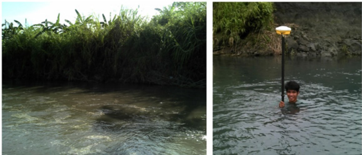
Figure 48. Tall cogon grass obstructs GNSS signals, some areas are too deep for manual bathymetry survey
