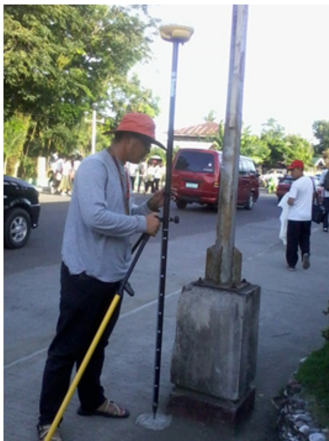
Figure 12. Static GNSS observation at control point IL-391A along the Anilao-Zarraga National Highway in Barotac Nuevo
