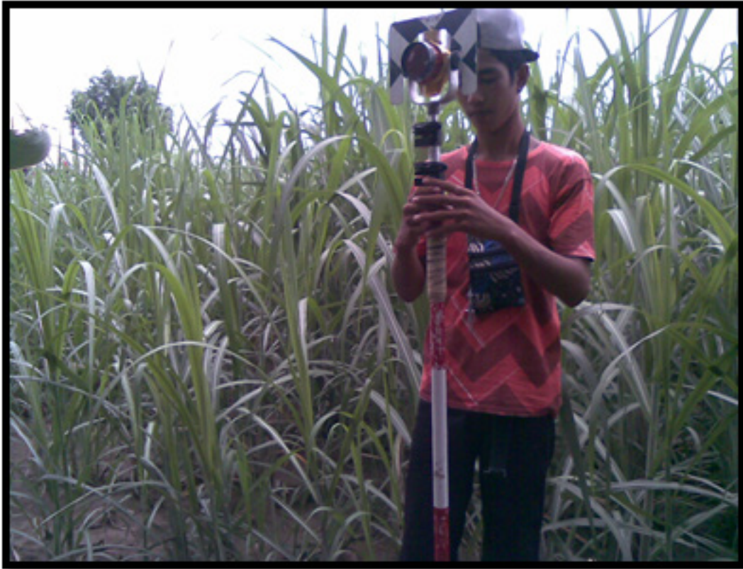
Figure 98: Conducting cross-section survey using Total Station at cross-section 2 at Brgy. Gemat-y, Passi City
