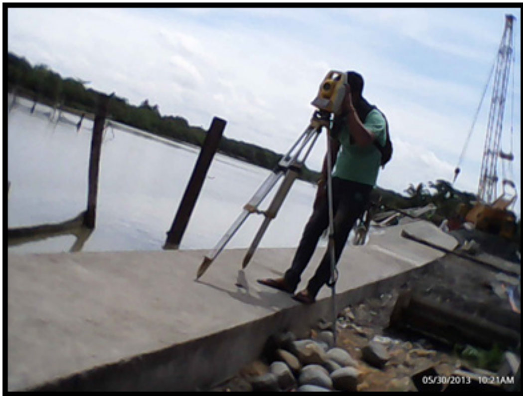
Figure 105: Conducting profile survey using Hi-Target Prismless at Brgy. Nabitasan, Leganes
