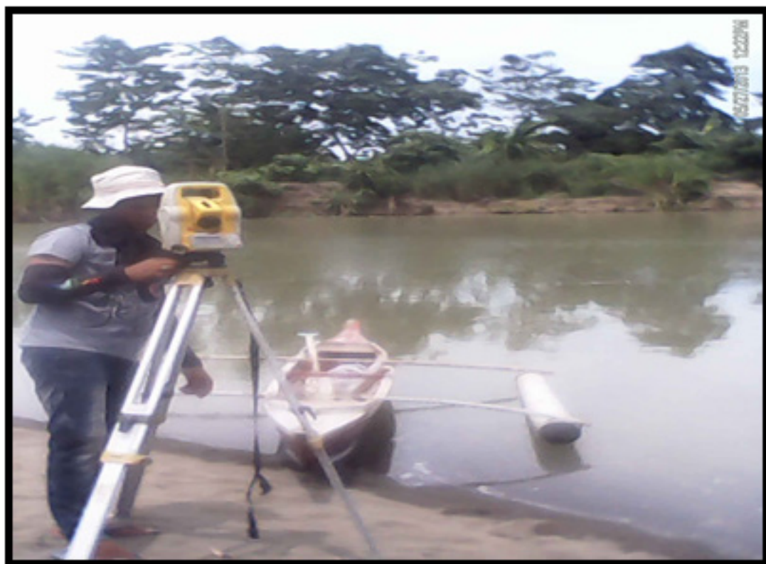
Figure 106: Conducting profile survey using Hi-Target Prismless at Brgy. Tubigan, Zarraga
