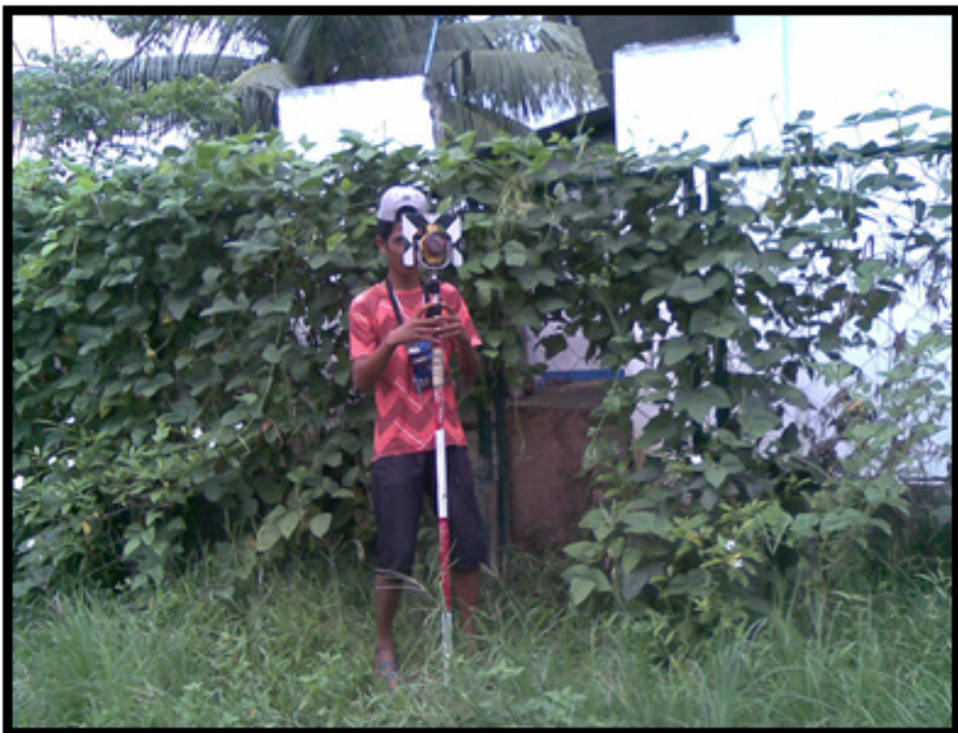
Figure 99: Conducting cross-section survey using Total Station at cross-section 4 at Brgy. Poblacion Ilaya, Passi City
