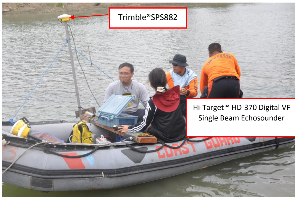
Figure 15. The setup of instruments for bathymetry survey with Trimble®SPS882 mounted on top of the Hi-Target™Transducer
