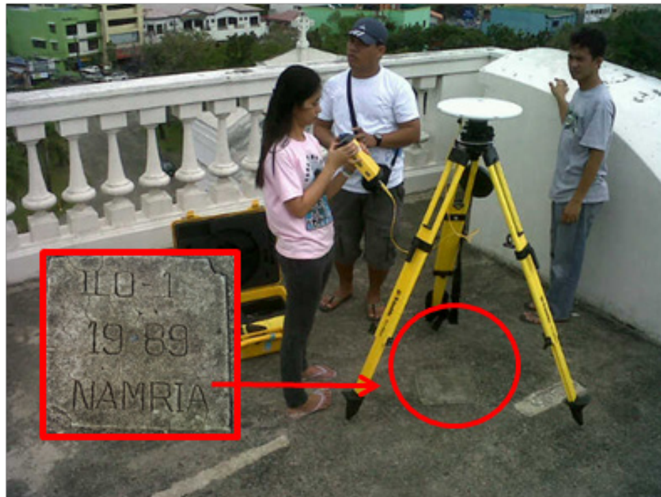
Figure 10. Static GNSS observation at ILO-1 on top of St. Clement's Bell Tower in Jaro District, Iloilo City
