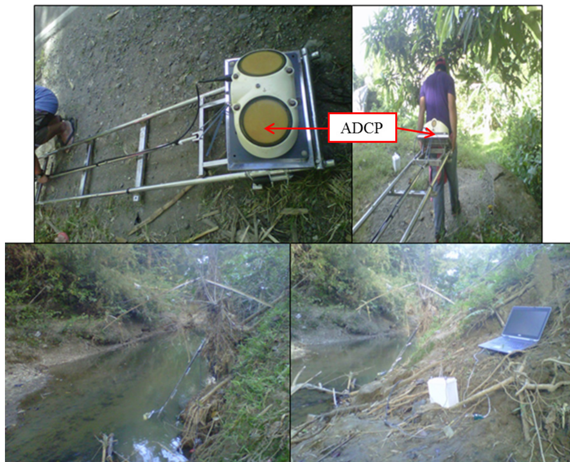
Figure 22. A series of pictures displaying the components and deployment of the ADCP in Maniniw River
