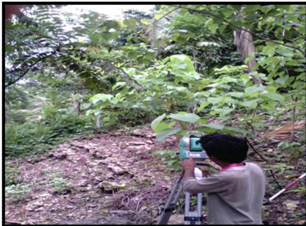
Figure 97: Conducting cross-section survey using Total Station at cross-section 7 at Brgy. Camiri, San Enrique
