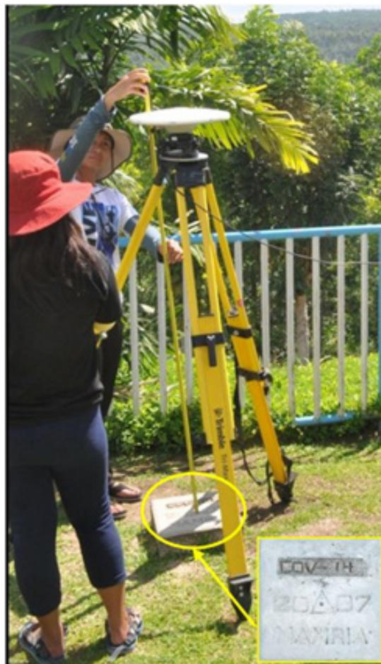
Figure 13. Static GNSS observation at COV-14 in front of Maco Municipal Hall in Barangay Poblacion, Maco, Compostela Valley
