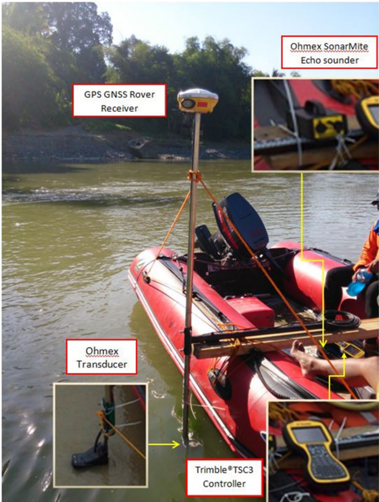
Figure 14. Bathymetric survey setup
