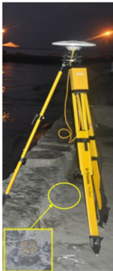
Figure 11. Static GNSS observation at DVS-1 in Port Area, Sta. Ana Wharf, Davao City
