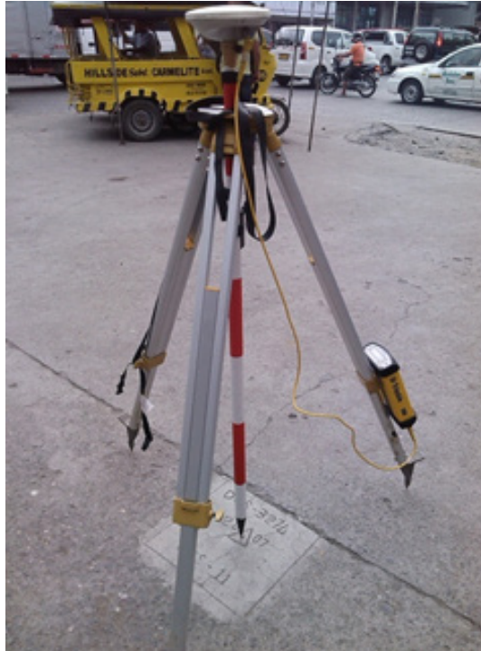
Figure 35. Static GNSS observation in DVS 3274 located at brgy Poblacion Davao City
