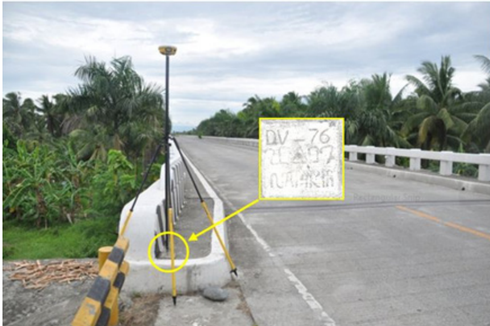
Figure 12. Static GNSS observation at DV-76 in Guadalupe Bridge, Tagum City
