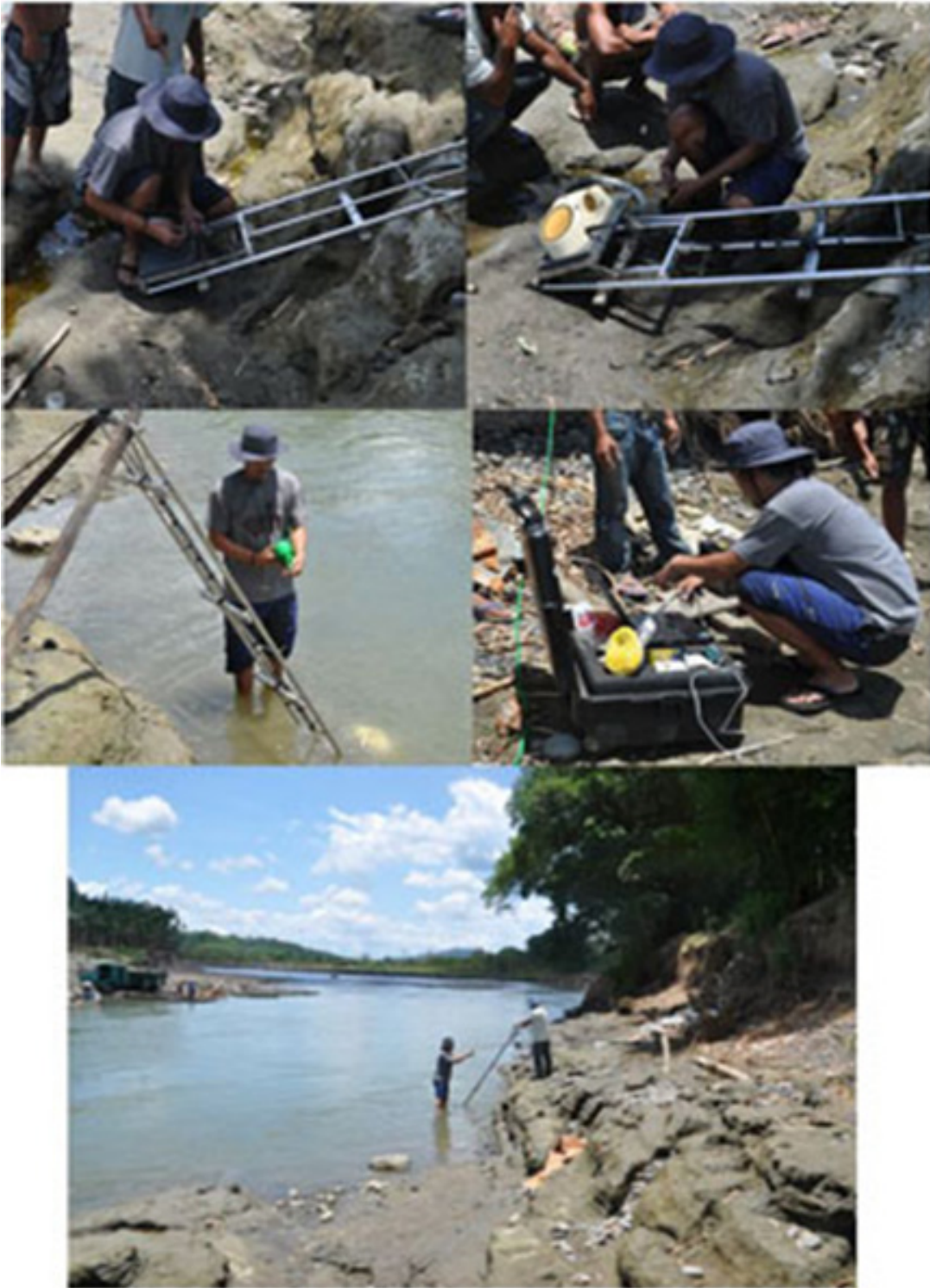
Figure 21. Deployment of ADCP with Depth Gauge on the bank of Davao River in Brgy. Waan, Davao City
