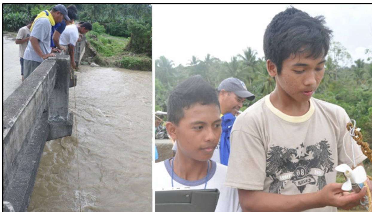
Figure 69. Flow measurements using a rotor-type flow meter
