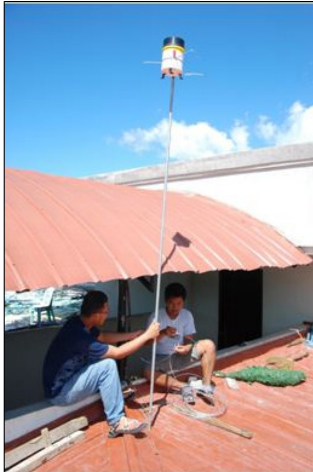
Figure 60. Rain Gauge deployment at the Roof top of New Bataan Town Hall
