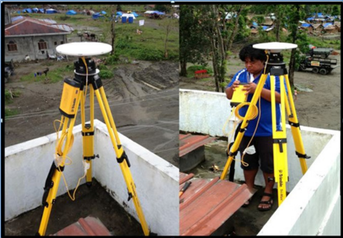
Figure 15. Static GNSS observation at UP-NB 1 at the roof top of New Bataan Town Hall in Brgy. Fatima, New Bataan, Compostela Valley
