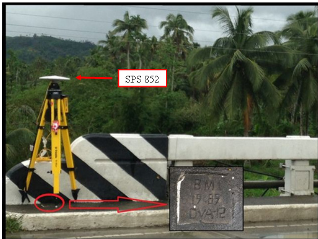
Figure 12. Static GNSS observation at DVA-12 at Mawab Bridge, Brgy. New Sibunga, Nabunturan, Davao del Norte
