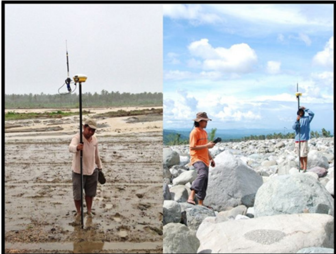
Figure 18. Cross-section using RTK surveying technique
