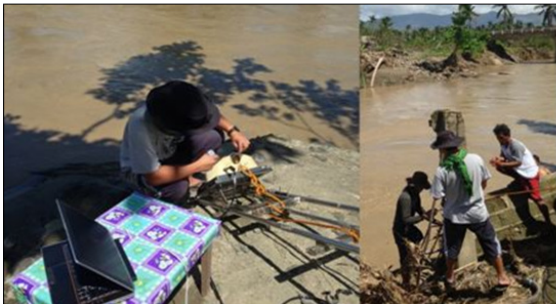
Figure 61. ADCP deployment with depth gauge in Brgy. Poblacion, Compostela
