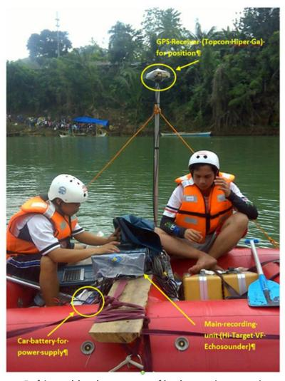
Figure 30. Rafting rubber boat setup of bathymetric survey instrument
