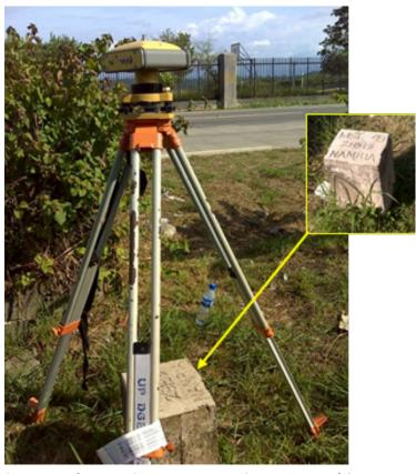
Figure 13. Static GNSS observation on MSE-49 in Brgy. Lumbia, Cagayan de Oro City
