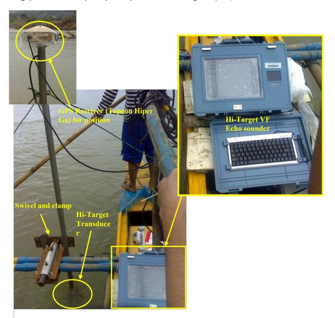
**Figure 29.** Bathymetric survey setup using Topcon® Hiper Gamounted on top of the Hi-Target™ Transducer
