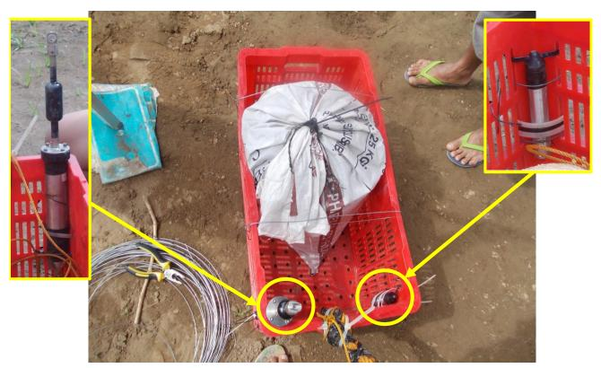
Figure 34. Sensors setup of velocity meter and depth gauge
