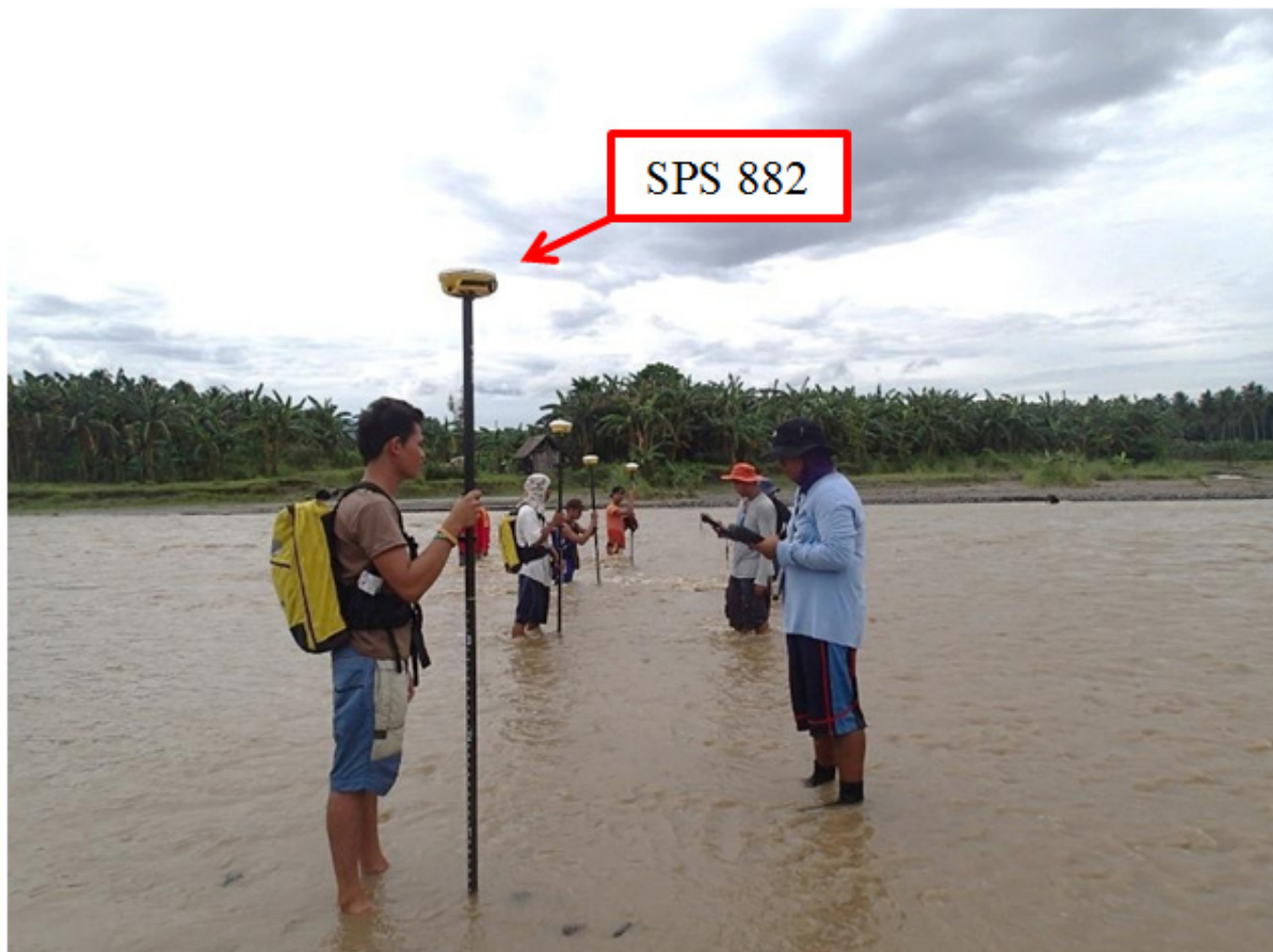
Figure 15. Manual bathymetric survey using PPK GNSS technique in Buayan-Malungon and Siluay Rivers
