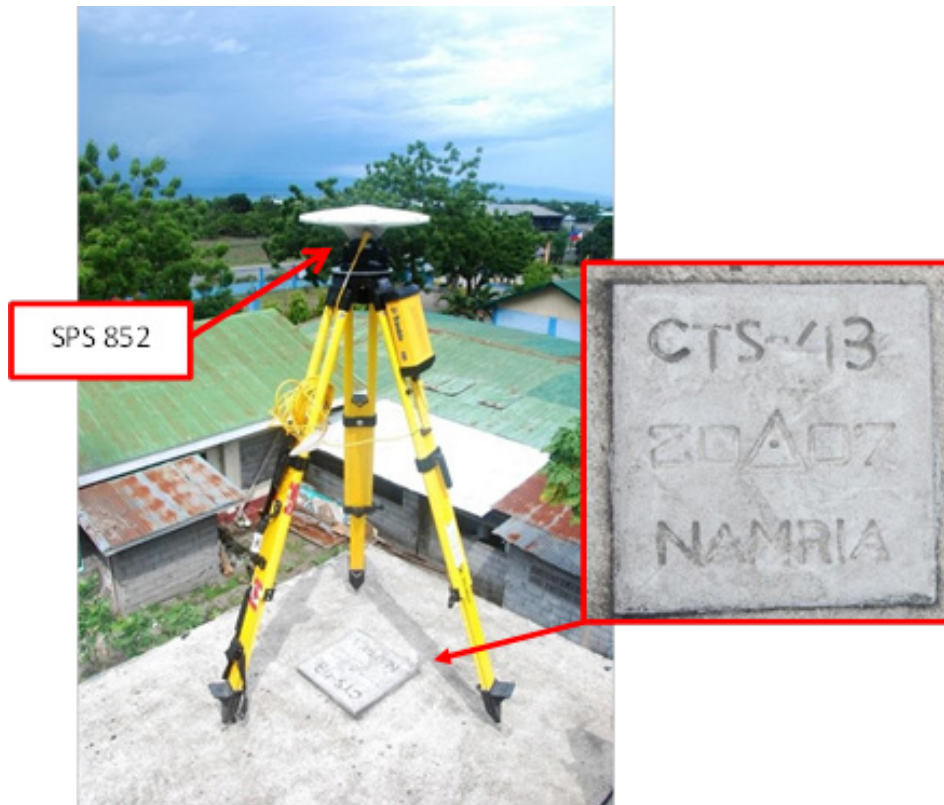
Figure 13. GNSS base station at CTS-43 in Brgy. Tambler, General Santos City
