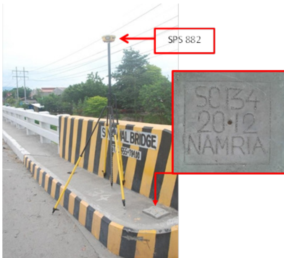
Figure 12. GNSS base station at SC-134 Brgy. Sinawal, General Santos City
