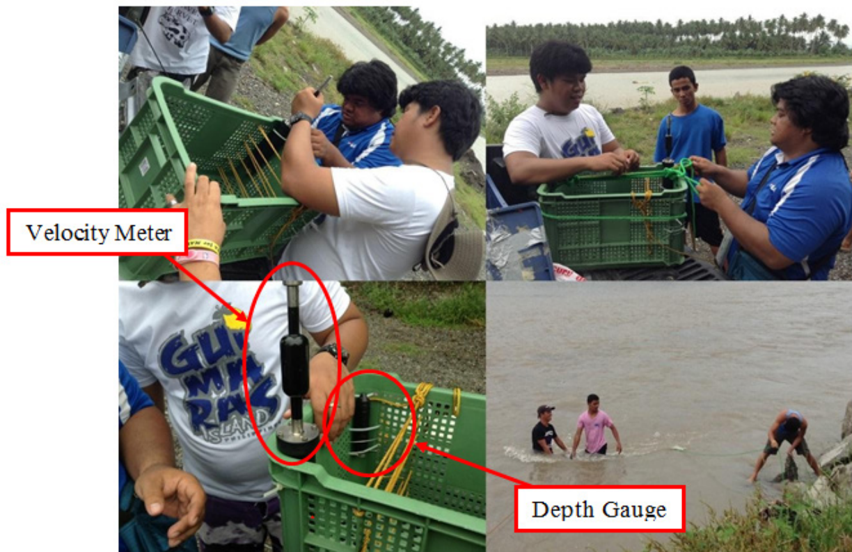
Figure 28. Deployment of velocity meter and depth gauge in Brgy. Ligaya, and temporary rain gauge installation at Brgy. Tinagacan, Buayan River
