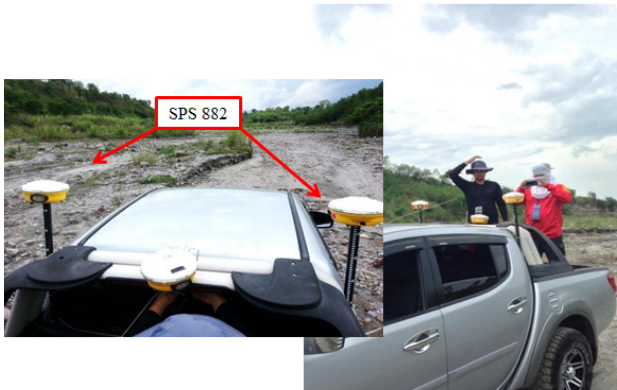
Figure 16. Setup of instruments for bathymetric survey using Trimble SPS 882 installed on a vehicle in Makar River.
