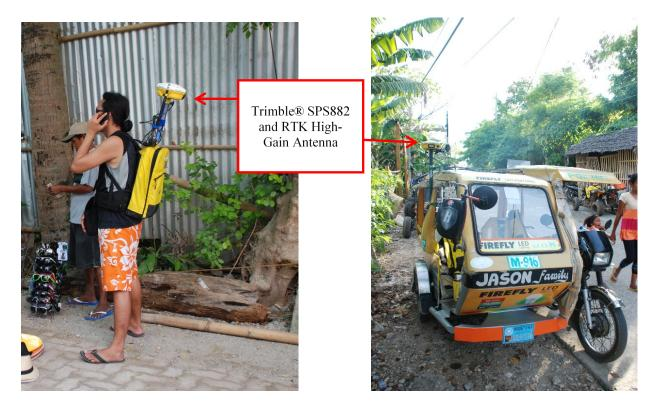
**Figure 18.** Validation Points Acquistion Survey using GNSS RTK technique by traversing the length of roads (a) by foot (b) as installed on a motorized vehicle
