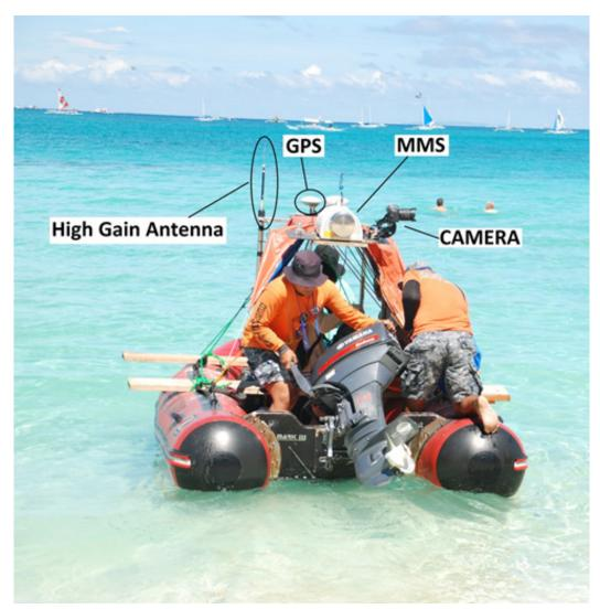
Figure 15. The MMS setup for the Boracay terrestrial LiDAR survey with PCG Boracay
