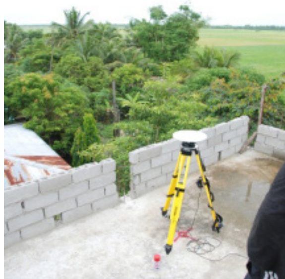
Figure 16. Static GNSS observation at Mangayawan
