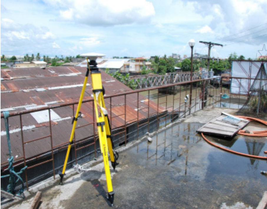
Figure 14. Static GNSS observation on top of Mabolo Barangay Hall
