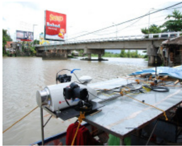
Figure 19. MDL Dynascan™ installed on one end of the boat for the river bank profile surveys of Bicol River
