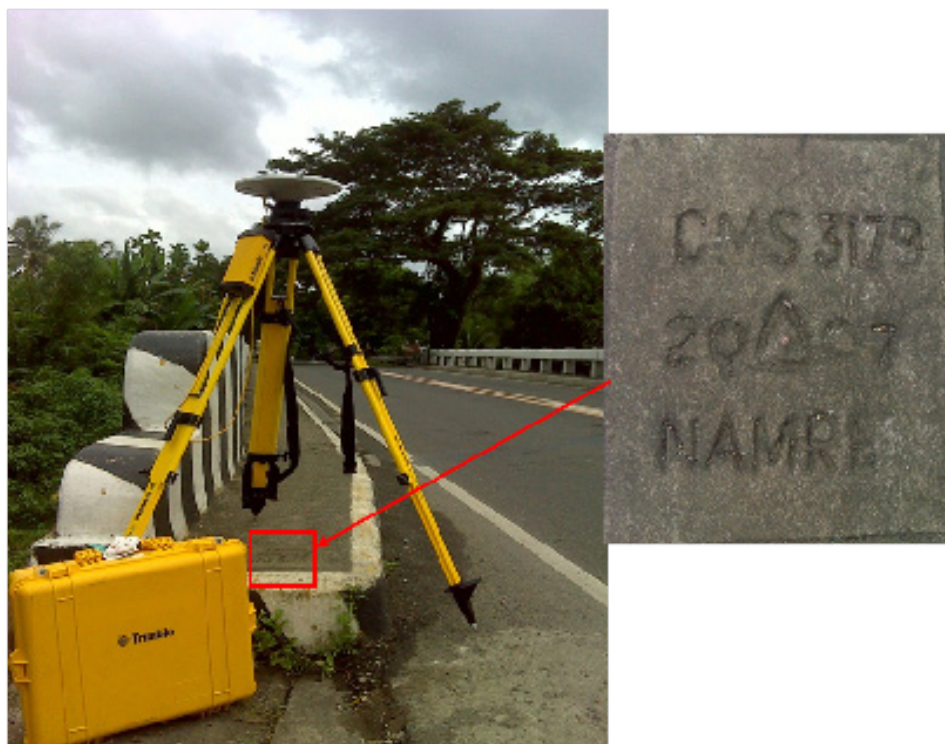
Figure 12. Static GNSS observation at CMS-3179
