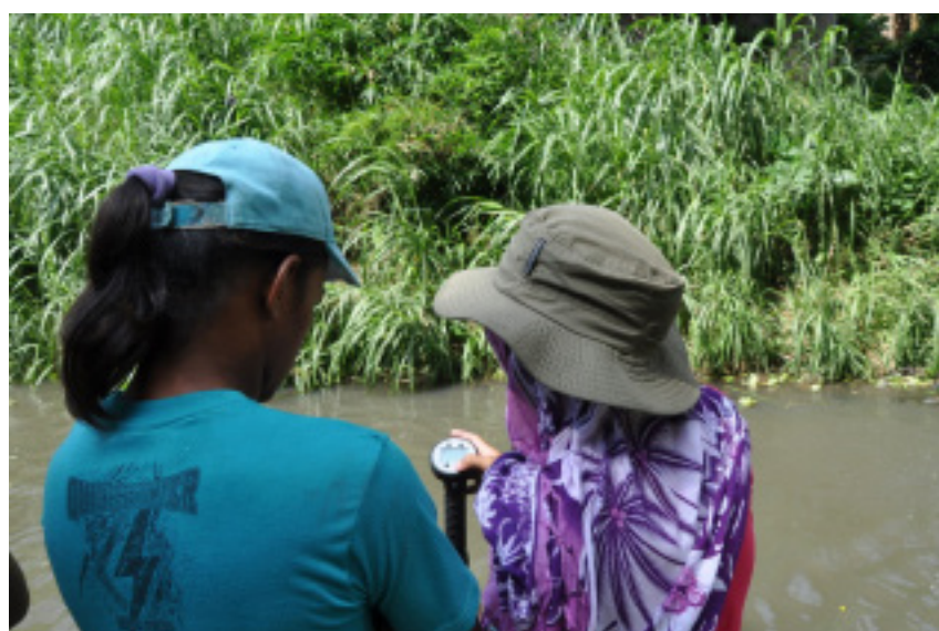
Figure 47. Flow measurements in Padre Garcia Bridge using Flow Probe FP111
