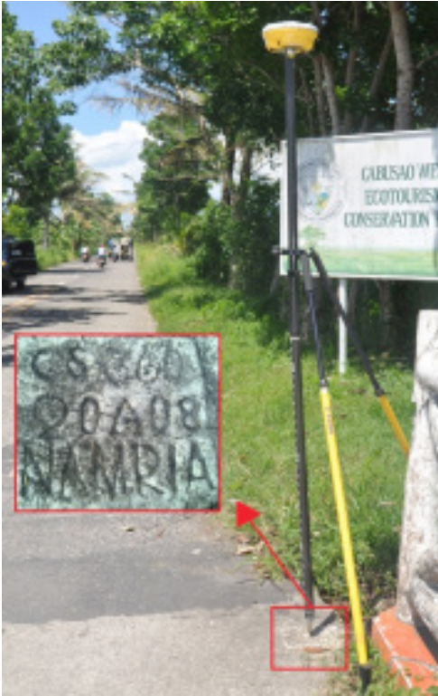
Figure 13. Static GNSS observation at CS-360
