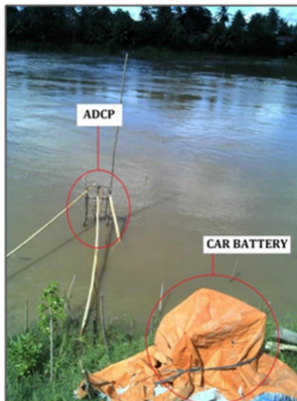
Figure 24. 3rd deployment of ADCP with depth gauge at Brgy. Mat-I, Las Nieves
