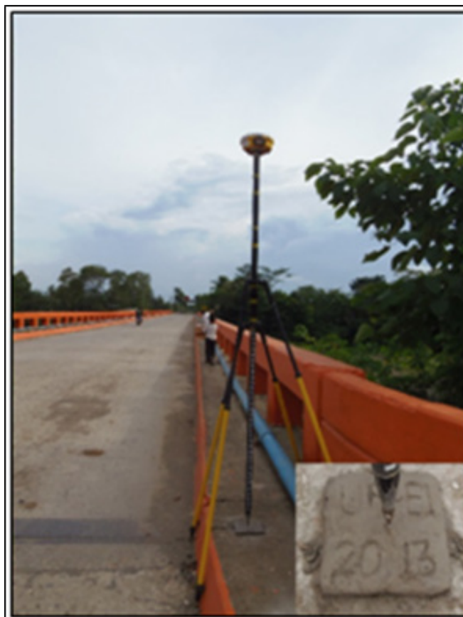
Figure 15. Static observation at UP E-1 at Esperanza Bridge, Municipality of Esperanza
