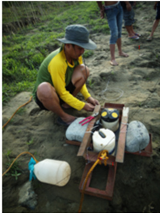
Figure 23. 2nd deployment of ADCP with depth gauge at Brgy. Mat-I, Las Nieves
