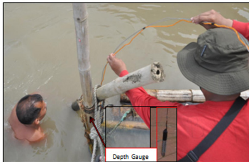
Figure 21. Deployment of depth gauge at Brgy. Pagatpatan, Butuan City
