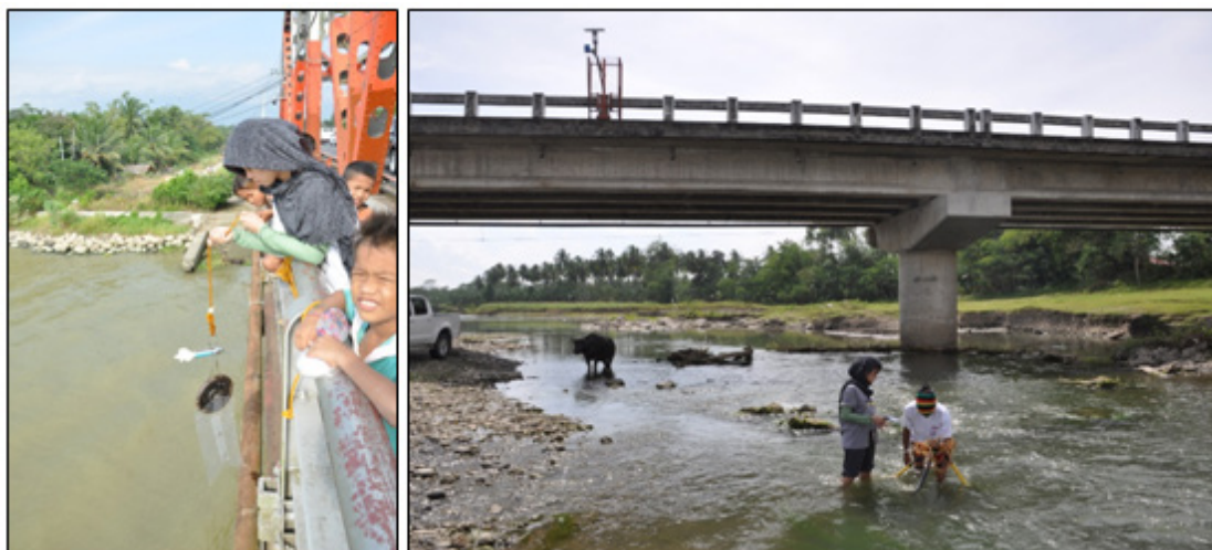
Figure 42. Flow measurements using a rotor-type flow meter at Butuan Bridge for DRRM River Base Leon Kilat AWLS and Adanan Bridge
