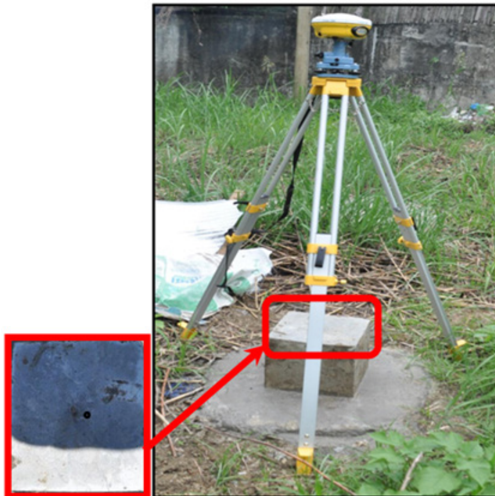
Figure 14. Static observation at the established control at Brgy. Ordoja, Butuan City near Magsaysay Bridge
