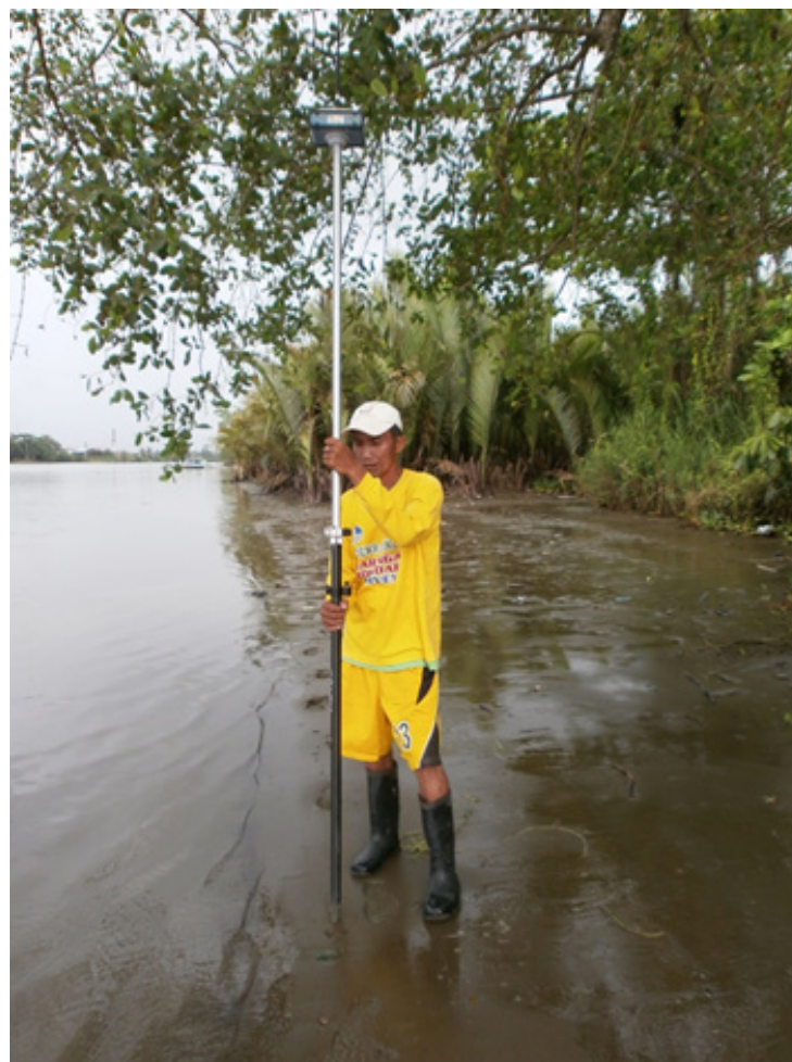
Figure 55. Profile team conducting a profile survey of Agusan River
