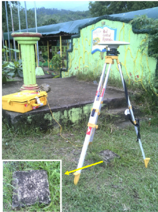
Figure 12. Static GNSS observation at QZN-5 at Real Central Elementary School
