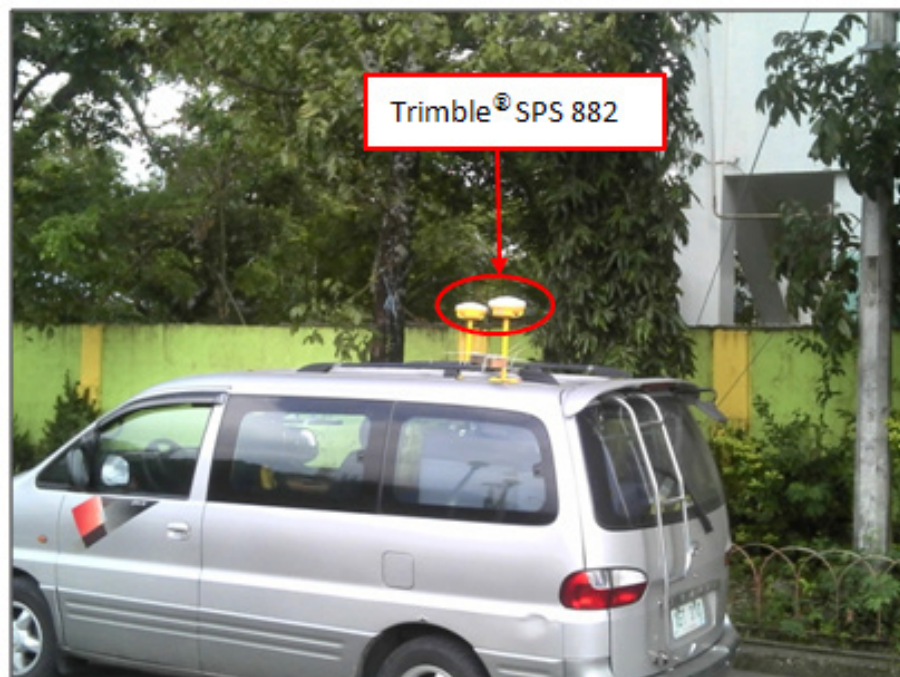
Figure 19. Validation points acquisition survey setup
