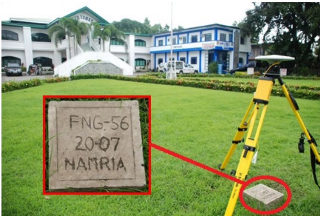
Figure 12. Static GNSS Network Observation Set-up at PNG-56 in Sto.Tomas, Pangasinan
