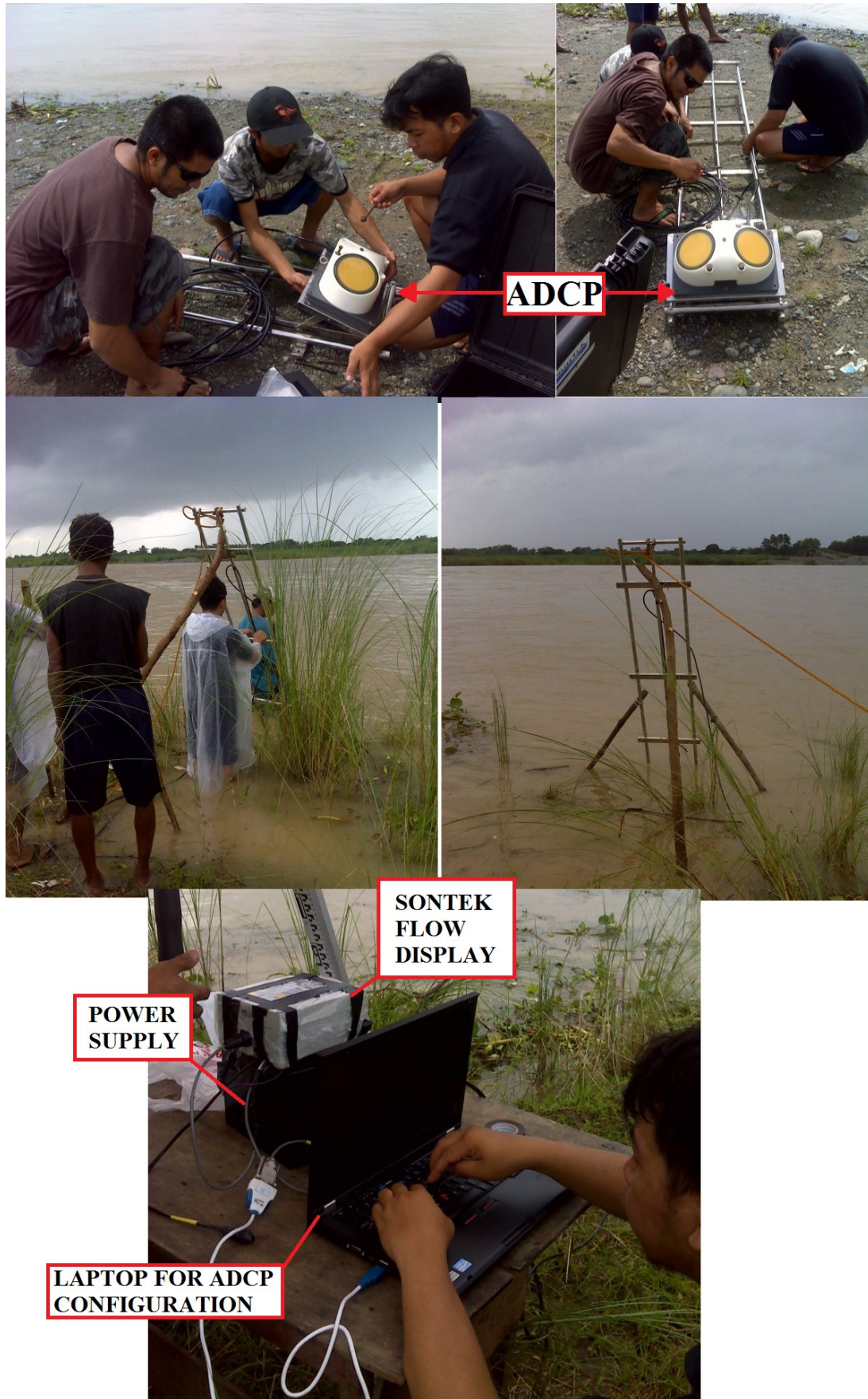
Figure 39. Series of pictures displaying the components and the deployment of ADCP on the bank of Agno River in Barangay Paitan, Sta. Maria
