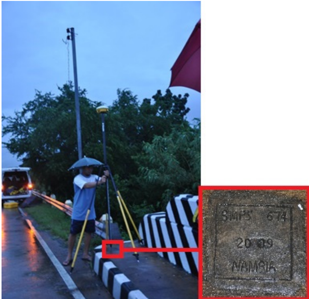
Figure 13. Trimble SPS 882 Rover Set-up at PS-674 at Ramos Bridge in Asingan, Pangasinan
