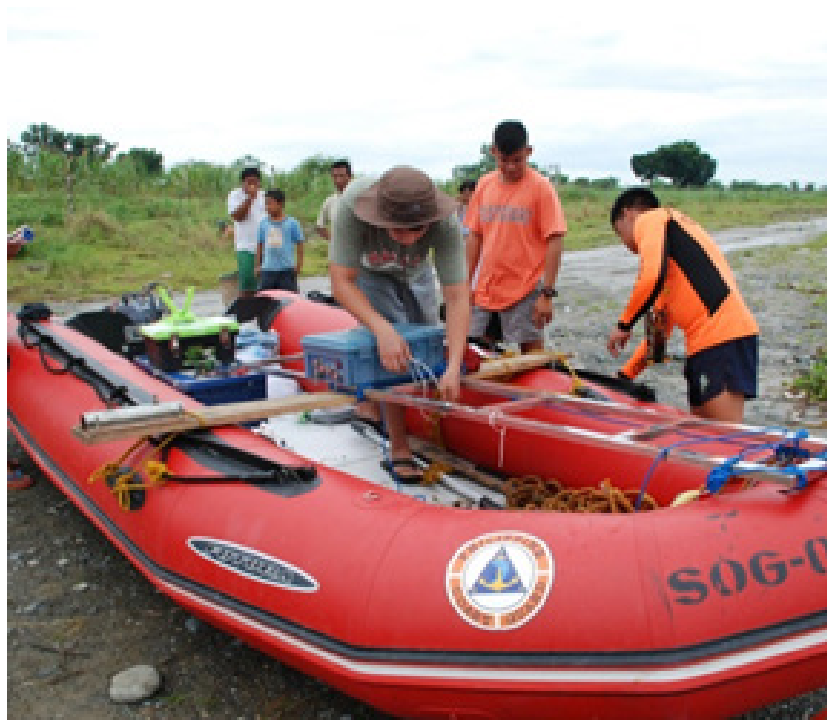
Figure 34. Securing the Hi-Target™ HD-370 Digital VF Single Beam Echo Sounder on top of the rubber boat with a metal frame and wooden plank
