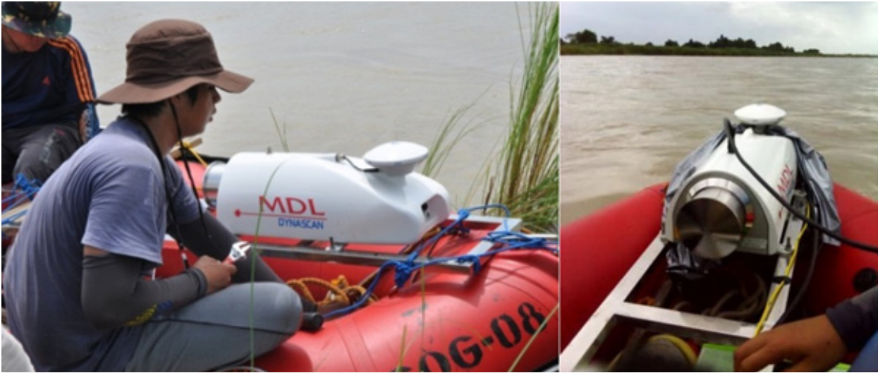
Figure 23. The MDL Dynascan installed on one end of the rubber boat was used to profile the lower banks of Agno River
