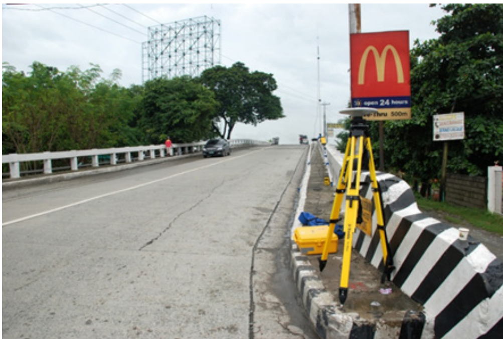
Figure 14. Control Point established at Villasis Bridge in Villasis, Pangasinan
