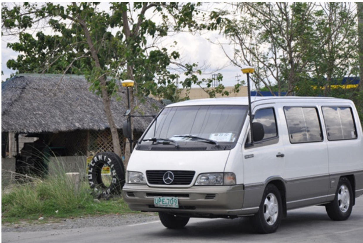
Figure 32. Manual ground LiDAR Validation using Trimble SPS882 Rover
