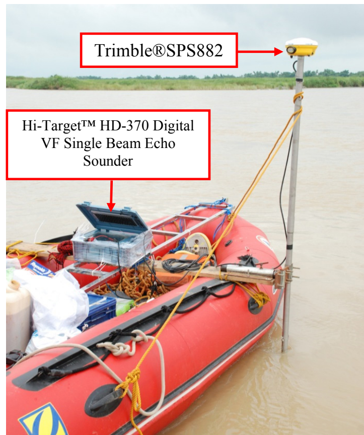
Figure 36. The set-up of instruments for the bathymetric survey with the Trimble®SPS882 mounted on top of the Hi-Target™ Transducer
