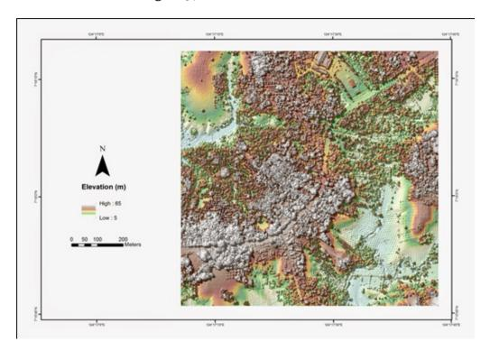
Figure 36. Sample 1x1 square kilometer DSM
