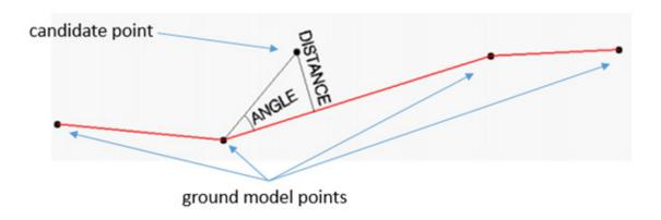
Figure 14. Ground classification technique employed in Terrascan
