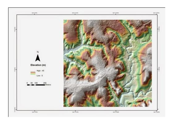
Figure 37. Sample 1x1 square kilometer DTM
