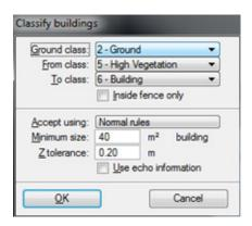
Figure 16. Default TerraScan building classification parameters
