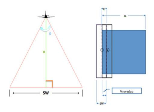
Figure 6. Concept of LiDAR data acquisition parameters
