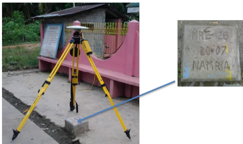
Figure 18. NAMRIA Control Station MRE-26, Located in San Teodoro, Calapan City
