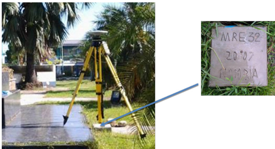
Figure 19. NAMRIA Control Station MRE-32, Located in Victoria, Calapan City
