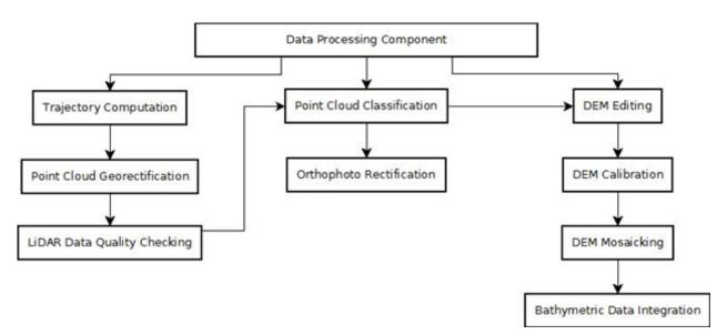
Figure 9. Schematic diagram of the data processing
