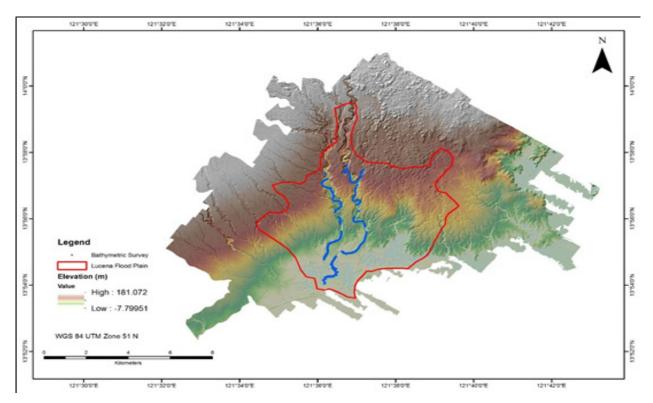
Figure 33. Final DTM of Lucena with validation survey shown in blue
