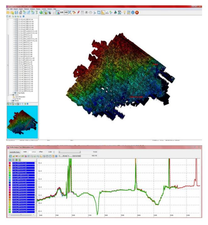
Figure 27. Quality checking with the profile tool of QT Modeler
