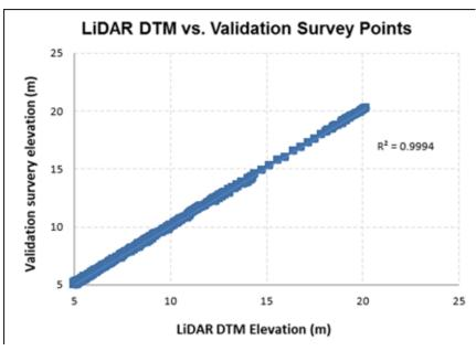
Figure 30. One-one Correlation plot between topographic and LiDAR data
