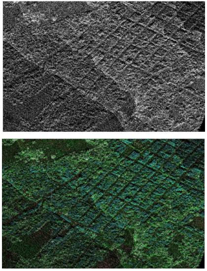
Figure 27. Point cloud (a) before and (b) after classification.
