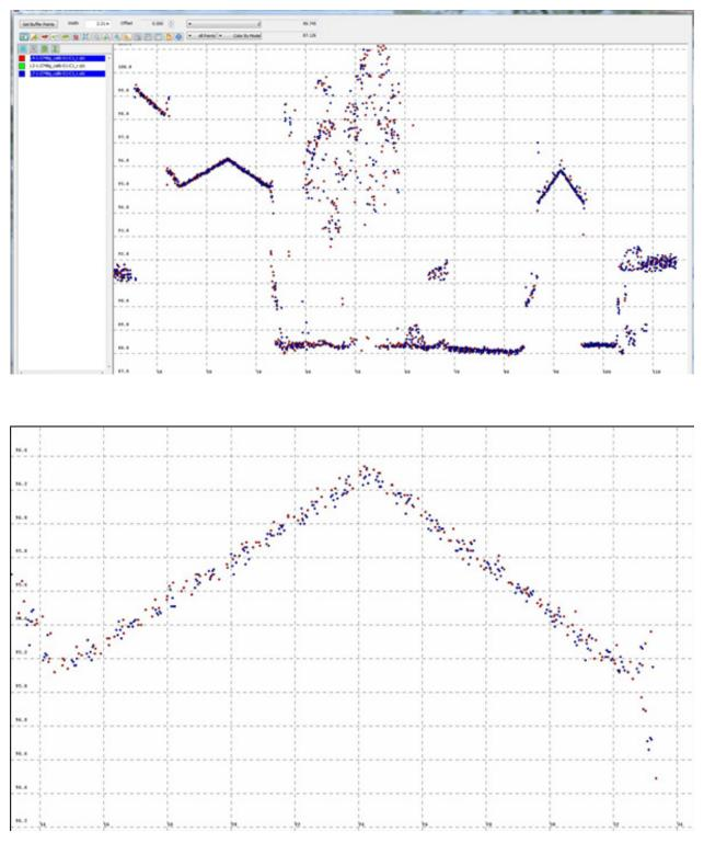
Figure 12. Profile over roof planes (a) and a zoomed-in profile on the area encircled in yellow (b)
