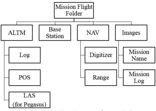
Figure 7. LiDAR Data Management for transmittal
