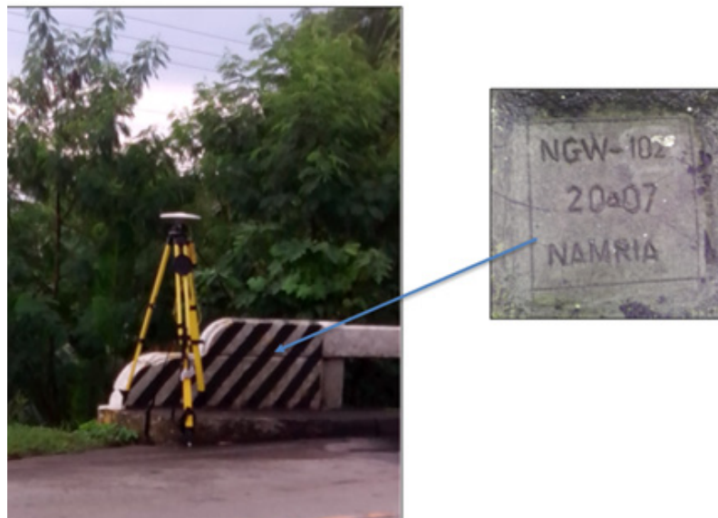
Figure 18. NGW-102 located in Toyuman Bridge in Himamaylan City, Negros Occidental
