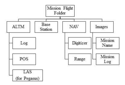
Figure 7. LiDAR Data Management for transmittal
