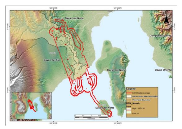
Figure 23. Coverage of LiDAR data for the Davao mission
