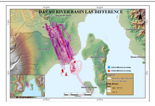
Figure 26. Elevation difference map between flight lines
