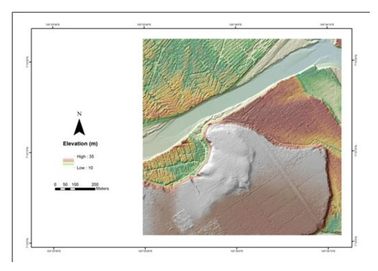
Figure 36. Sample 1x1 square kilometer DTM
