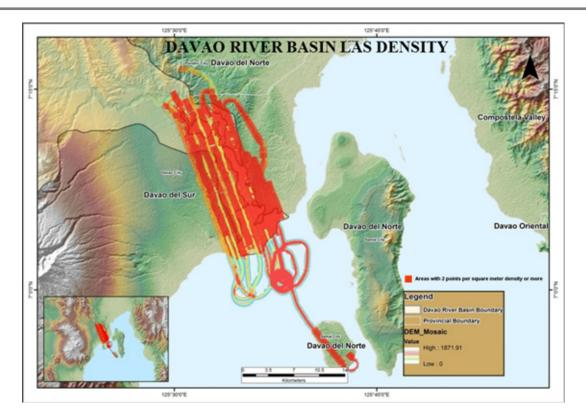
Figure 25. Density map of merged LiDAR data for the Davao mission
