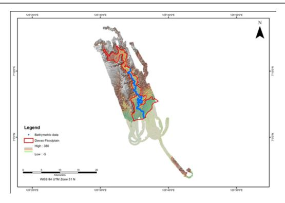
Figure 33. Final DTM of Davao with validation survey shown in blue
