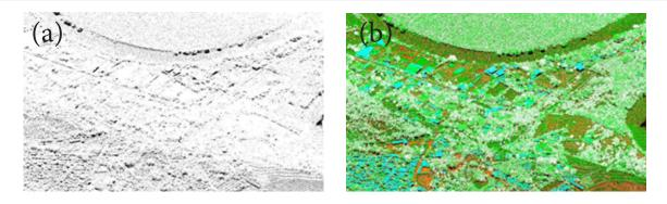
Figure 29. Point cloud (a) before and (b) after classification
