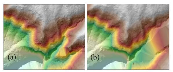
Figure 14. Resulting DTM of ground classification using the default parameters (a) and adjusted parameters (b)
