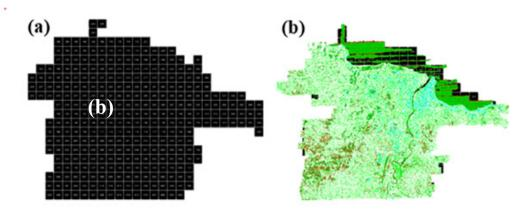
Figure 33. (a) Cagayan de Oro and Iponan blocks and (b) Cagayan de Oro and Iponan classification results in TerraScan
