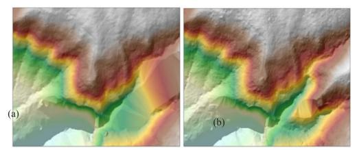
Figure 17. Resulting DTM of ground classification using the default parameters (a) and adjusted parameters (b)
