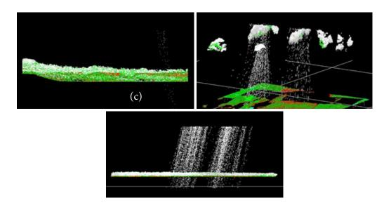
Figure 19. Different examples of air points manually deleted in the TerraScan window
