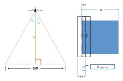
Figure 9. Concept of LiDAR data acquisition parameters
