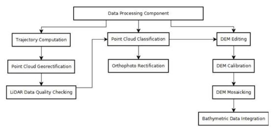
Figure 12. Schematic diagram of the data processing
