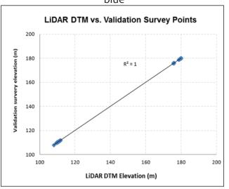
Figure 37. One-one Correlation plot between topographic and LiDAR data for Cagayan de Oro
