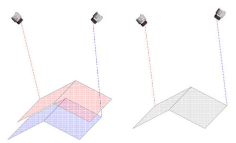
Figure 13. Misalignment of a single roof plane from two adjacent flight lines, before rectification (left). Least squares adjusted roof plane, after rectification (right).
