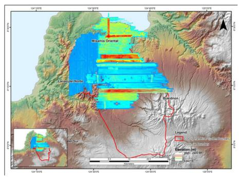
Figure 29. Image of data overlap for the Cagayan de Oro and Iponan mission
