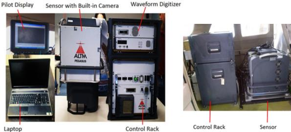
LaptopControl RackControl RackSensorFigure 8. The ALTM Pegasus System: a) parts of the Pegasus system, b) the system as in-<br/>stalled in Cessna T206H
