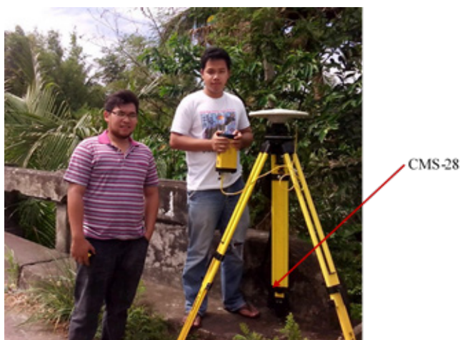
Figure 19. NAMRIA control station CMS-28 is located along the road going to Brgy. Fundado, Canaman
