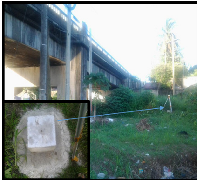
Figure 18. The DVC established control point Butuan BM under Marcos Bridge in Butuan City.
