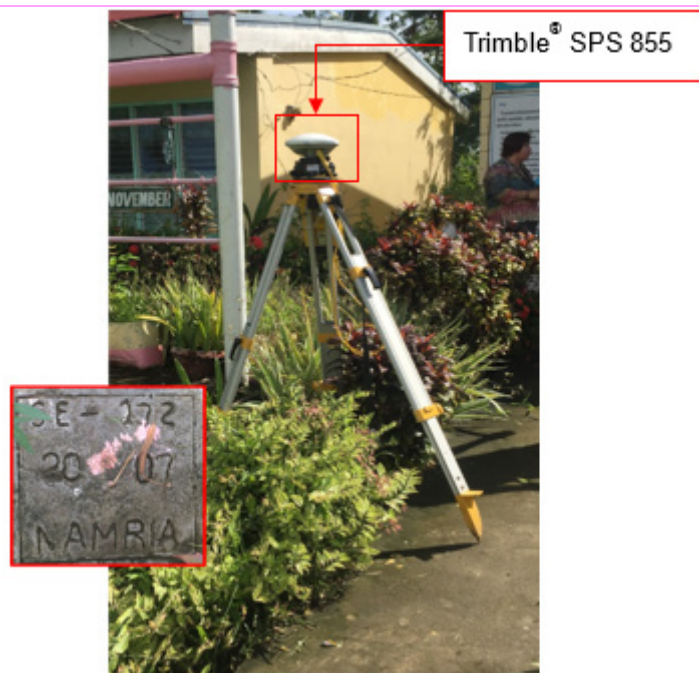
Figure 31. GNSS receiver set up, Trimble® SPS 855, at SE-172, located inside Nato Elementary School in Brgy. Nato, Taft, Eastern Samar
