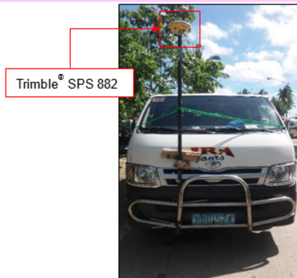
Figure 41. Validation points acquisition survey set-up for Ulot River
