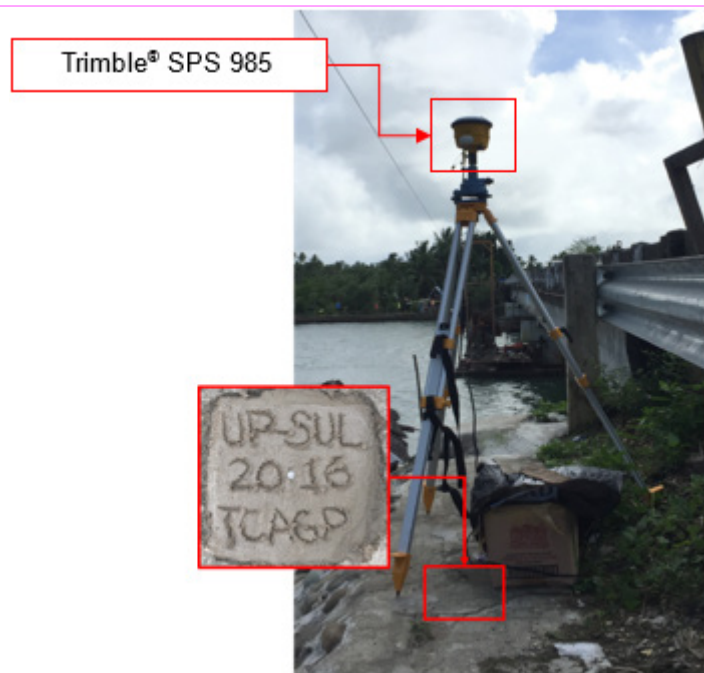
Figure 33. GNSS receiver setup, Trimble® SPS 985, at UP-SUL, located at the approach of Sulat Bridge in Brgy. Maramara, Sulat, Eastern Samar
