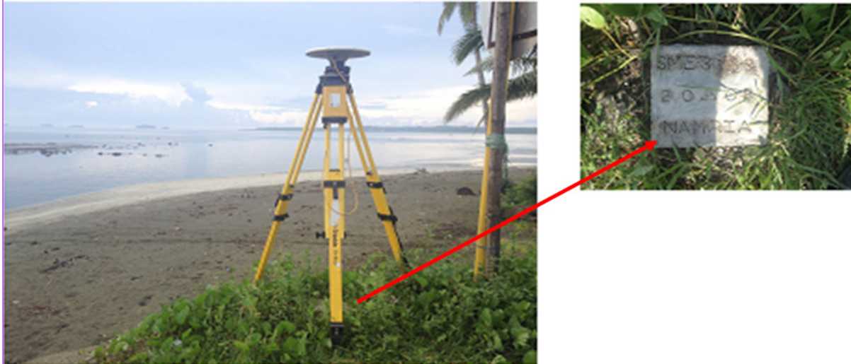
Figure 3. GPS set-up over SME-3139 located along the highway in Brgy. Sto. Nino, Ulot, Eastern Samar (a) and NAMRIA reference point SME-3139 (b) as recovered by the field team.
