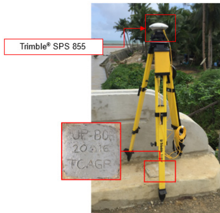
Figure 34. GNSS receiver setup, Trimble® SPS 855, at UP-BOR, located at the approach of Can-Obing Bridge in Brgy. Can-Abong, Borongan City, Eastern Samar
