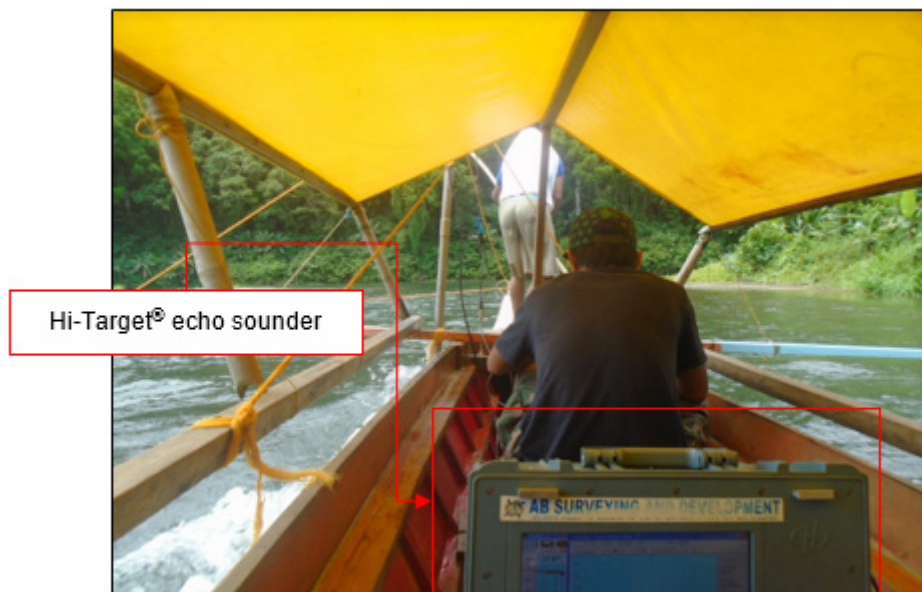
Figure 43. Bathymetric survey of ABSD at Ulot River using Hi-Target® echo sounder
