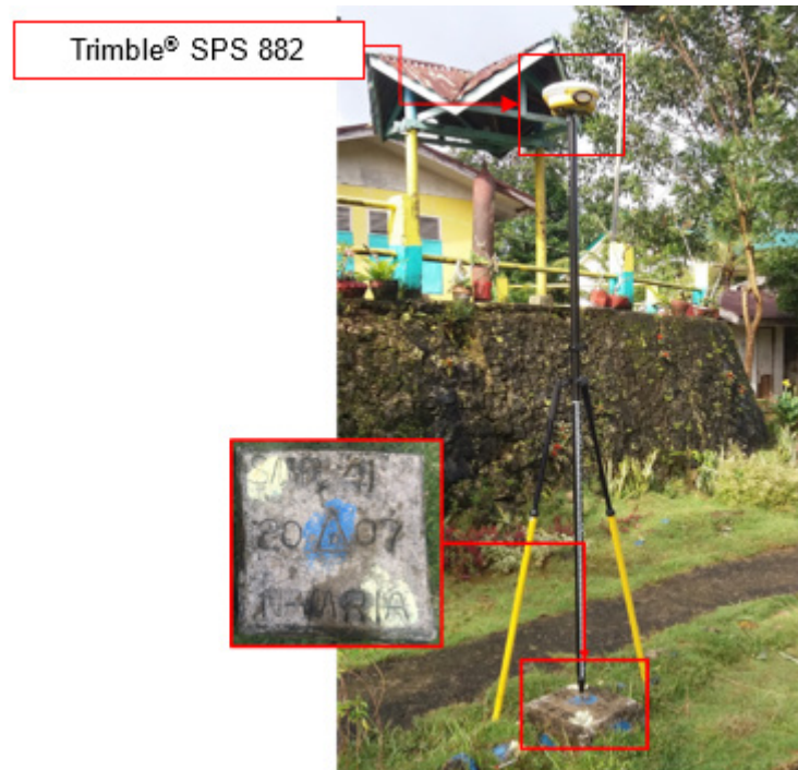
Figure 29. GNSS receiver setup, Trimble® SPS 882 at SMR-41, located at Bagacay Elementary School in Brgy. Bagacay, Hinabangan, Eastern Samar
