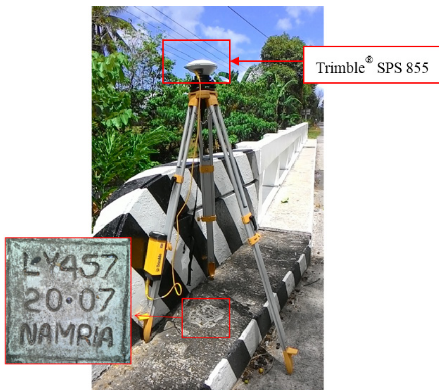
Figure 33. GNSS base set-up, Trimble® SPS 855, at LY-457, located at the approach of the Tigbao-Cib Bridge 2 in Barangay Tigbao, Sogod, Southern Leyte
