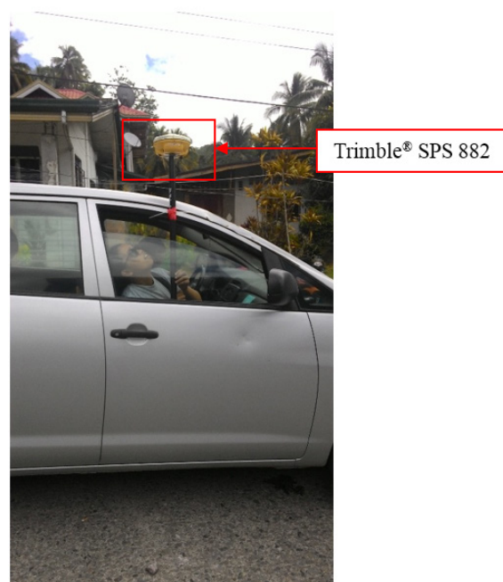
Figure 41. Validation points acquisition survey set-up
