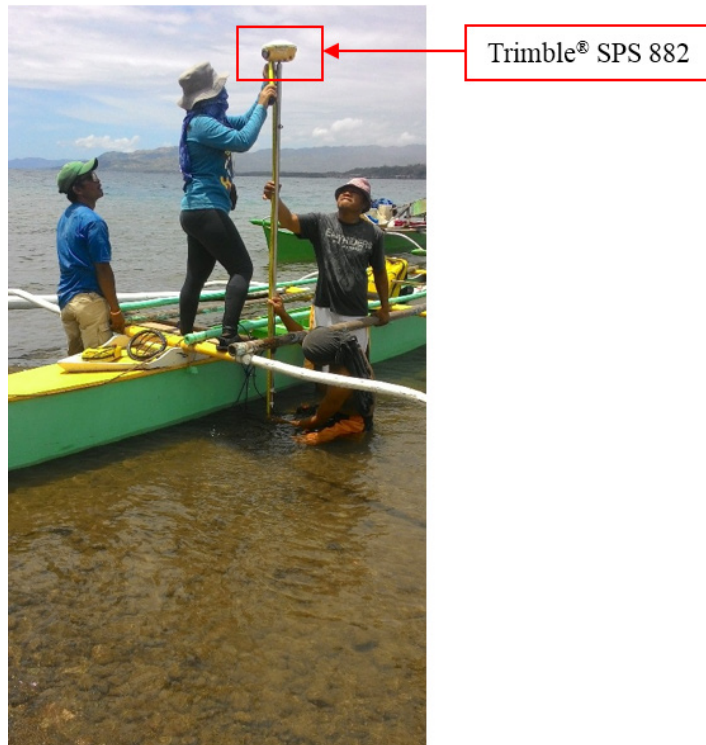
Figure 43. Bathymetry by boat set-up for the Subangdaku River survey
