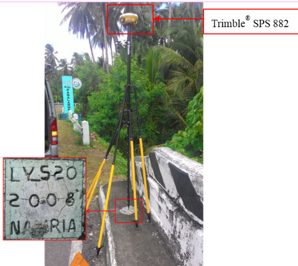
Figure 34. GNSS base set-up, Trimble® SPS 882, at LY-520, located along the approach of the Das-ay Bridge in Barangay Bisangon, Hinunangan, Southern Leyte
