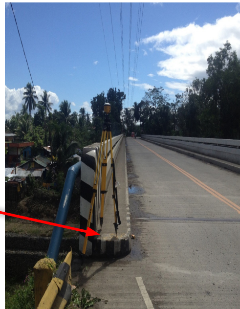
Figure 7. (a) GPS set-up over LY-439A; and (b) NAMRIA reference point LY-439A, as recovered by the field team
