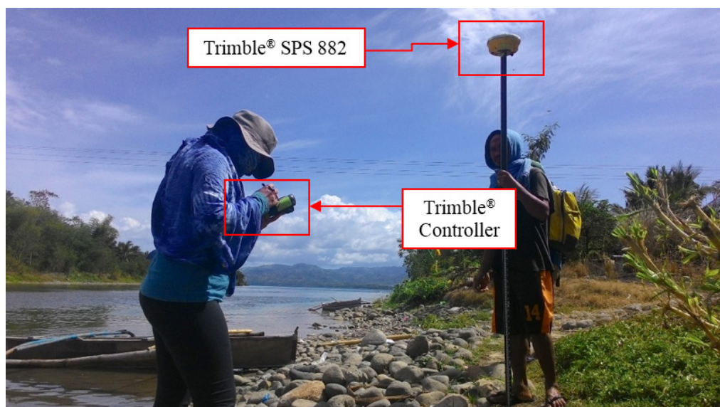
Figure 44. Manual bathymetry set-up for the Subangdaku River survey
