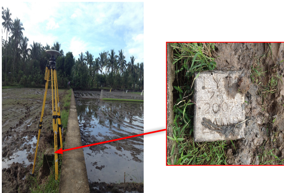
Figure 4. (a) GPS set-up over LYT-731, located in Barangay Kansungka, Baybay City, Leyte; and (b) NAMRIA reference point LYT-731, as recovered by the field team
