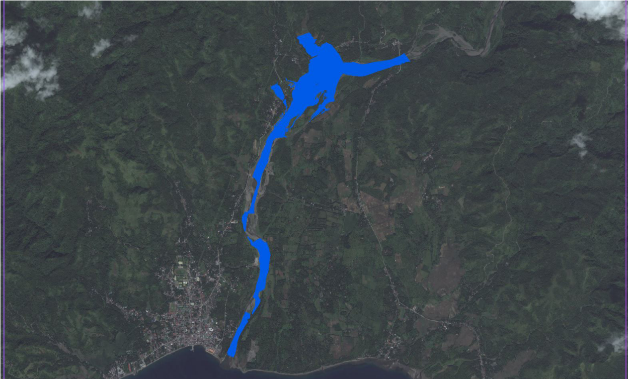
Figure 63. Sample output map of the Subangdaku RAS model
