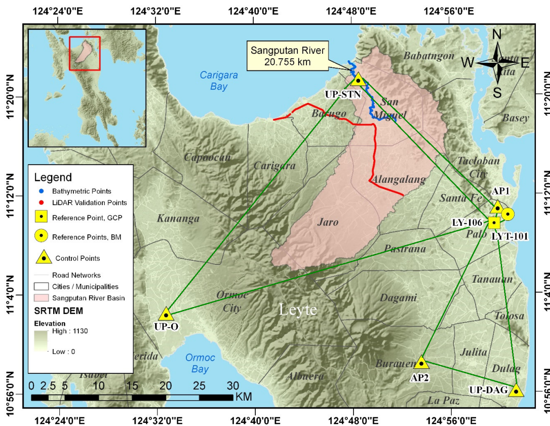
Figure 33. Extent of the bathymetric survey (in blue line) in the Sangputan River and the LiDAR data validation survey (in red)
