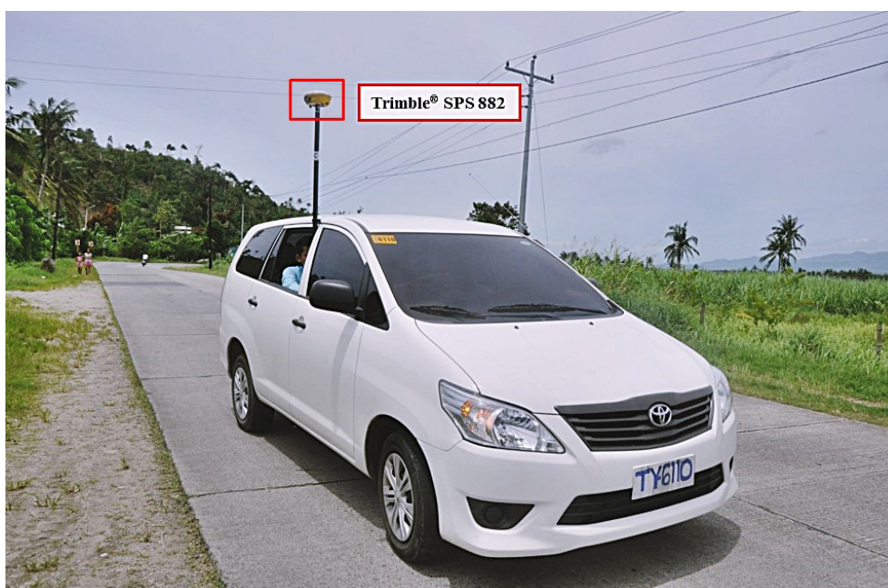
Figure 45. Validation points acquisition survey set-up
