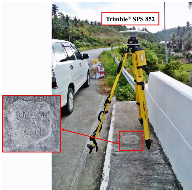
Figure 39. GNSS base set-up, Trimble® SPS 852, at UP-STN, an established control point, located at the Pagbanganan Bridge approach in Barangay Poblacion Zone 12, City of Baybay, Leyte
