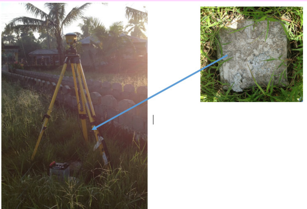
Figure 7. (a) GPS set-up over SMR-56 at Cabacungan Elementary School in Barangay Cabacungan, Sta. Rita, Samar; and (b) NAMRIA reference point SMR-56, as recovered by the field team
