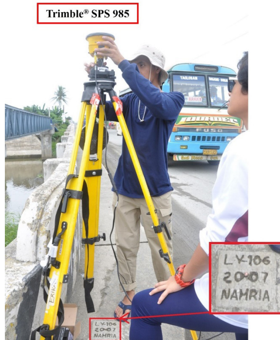
Figure 36. GNSS base set-up, Trimble® SPS 985, at LY-106, located at the approach of the Bernard Reed Bridge along Maharlika Highway in Barangay Luntad, Municipality of Palo, Leyte
