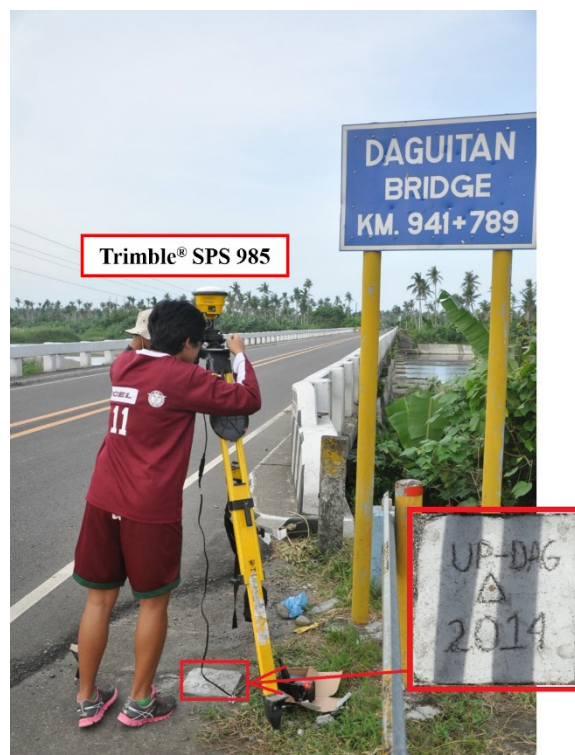
Figure 37. GNSS receiver set-up, Trimble® SPS 985, at UP-DAG, an established control point, located at the bridge approach of the Daguitan Bridge along Maharlika Highway in Barangay Fatima, Municipality of Dulag, Leyte
