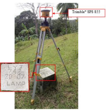
Figure 32. GNSS base set up, Trimble SPS 855, at LYT-742, located near a chapel and basketball court in Brgy. Tambis, Municipality of Hilongos, Leyte
