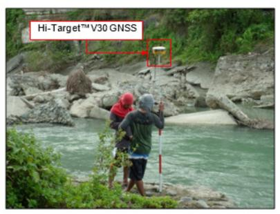
Figure 43. Manual bathymetric survey using a Hi-Target™ V30 GNSS in Salug River
