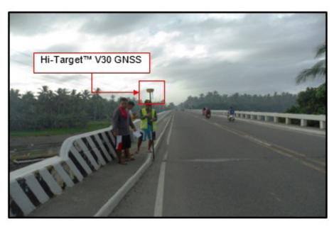
Figure 36. As-built survey of Salug Bridge
