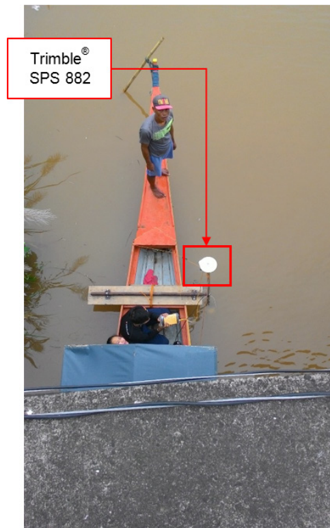
Figure 44. Set up of the bathymetric survey at Pambujan River using Trimble® SPS 882 in GNSS PPK survey technique.
