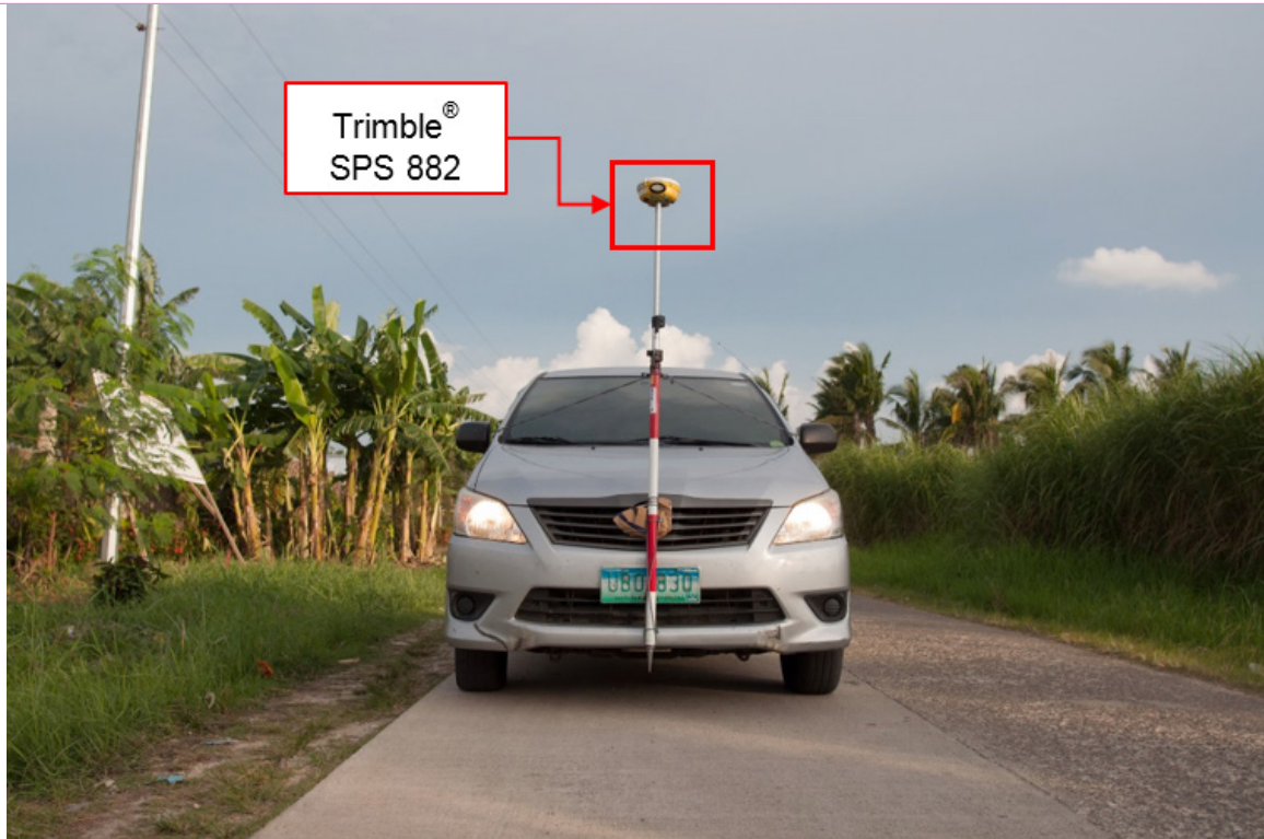
Figure 42. GNSS Receiver Trimble® SPS 882 installed on a vehicle for Ground Validation Survey.
