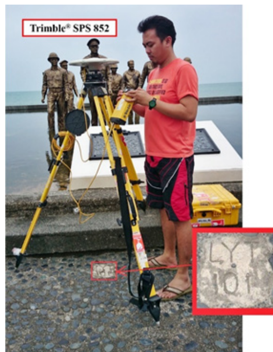
Figure 35. GNSS base set-up, Trimble® SPS 852, at LYT-101, located at the General McArthur Shrine in Brgy. Candahog, Municipality of Palo, Leyte
