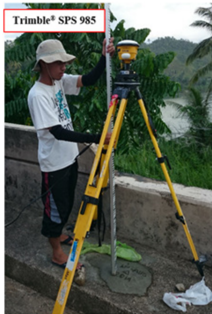
Figure 37. Trimble® SPS 985 GNSS set-up at UP-ABG in Cadacan Bridge, Abuyog, Leyte
