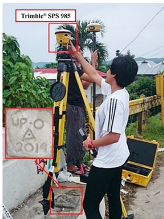
Figure 39. GNSS receiver set-up, Trimble® SPS 985, at UP-O, an established control point, located at the bridge approach of the Ormoc Merida Bridge along Ormoc-Merida-Isabel-Palompon Road in Brgy. Liloan, City of Ormoc, Province of Leyte
