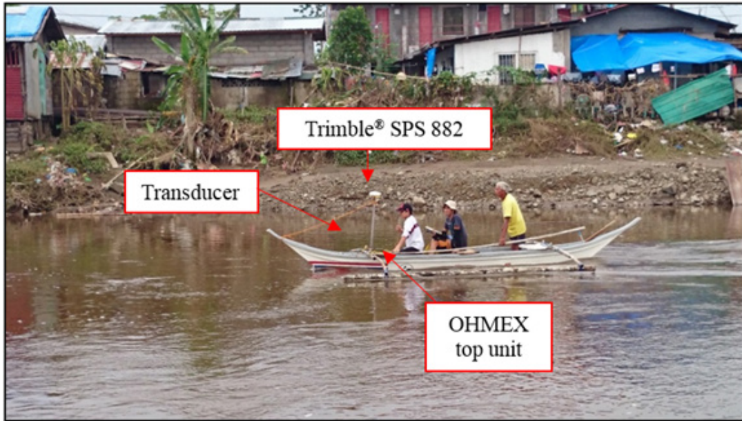
Figure 49. Bathymetric survey using an OHMEX™ Single Beam Echo Sounder with a mounted Trimble® SPS 882
