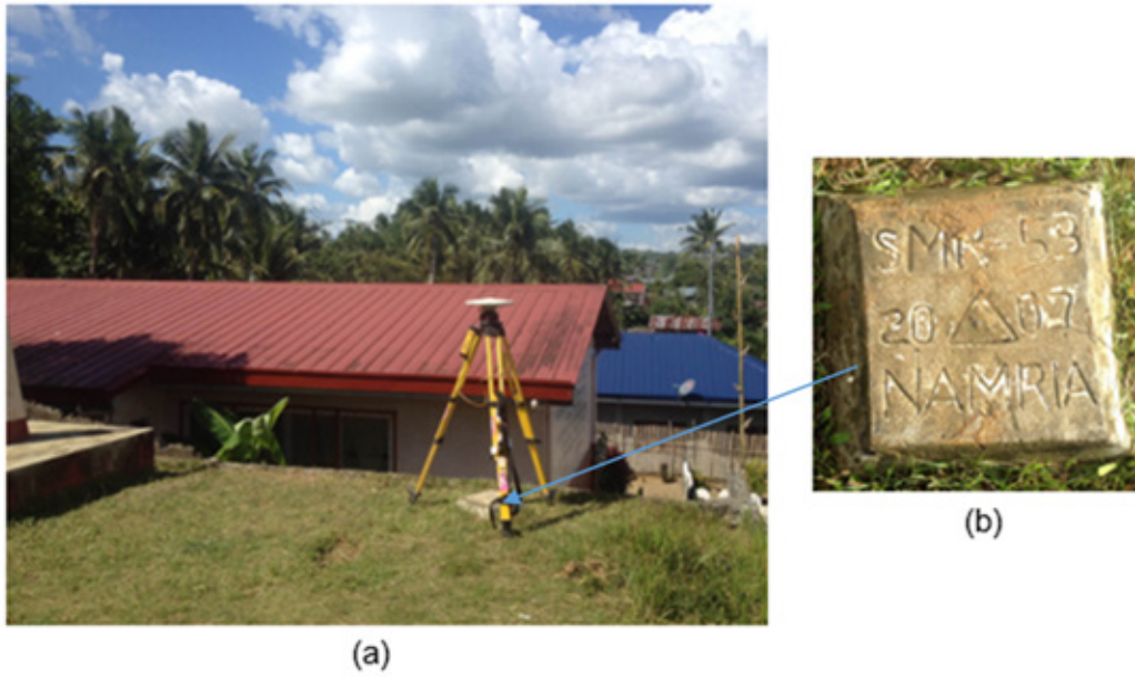
Figure 8. GPS set-up over SMR-56 located inside Cabacungan Elementary School in Brgy. Cabacungan, Sta. Rita, Samar (a) and NAMRIA reference point SMR-56 (b) as recovered by the field team.
