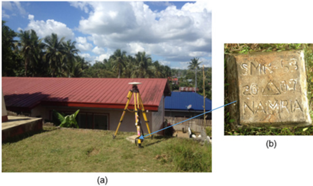
Figure 6. GPS set-up over SMR-53 located near the school building flag pole of San Isidro Elementary, Brgy. San Isidro, Santa Rita (a) and NAMRIA reference point SMR-53 (b) as recovered by the field team.
