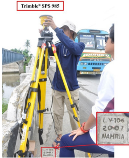
Figure 36. GNSS base set-up, Trimble® SPS 985, at LY-106, located at the approach of Bernard Reed Bridge along Maharlika Highway, Brgy. Luntad, Municipality of Palo, Leyte
