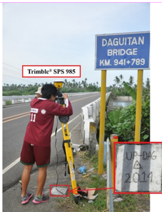
Figure 38. GNSS receiver set-up, Trimble® SPS 985, at UP-DAG, an established control point, located at the bridge approach of the Daguitan Bridge along Maharlika Highway in Brgy. Fatima, Municipality of Dulag, Province of Leyte
