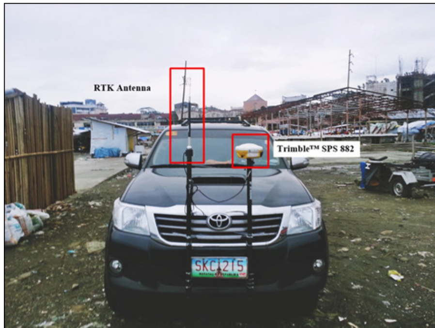
Figure 45. Trimble® SPS 882 and RTK antenna set-up in a van for LiDAR validation survey
