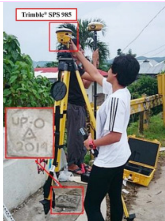
Figure 34. GNSS receiver set-up, Trimble® SPS 985, at UP-O, an established control point, located at the bridge approach of the Ormoc Merida Bridge along Ormoc-Merida-Isabel-Palompon Road in Barangay Liloan, City of Ormoc, Leyte
