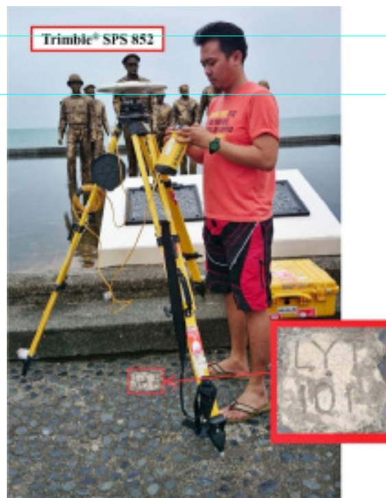
Figure 31. GNSS base set-up, Trimble® SPS 852, at LYT-101, located at the General McArthur Shrine in Barangay. Candahog, Municipality of Palo, Leyte
