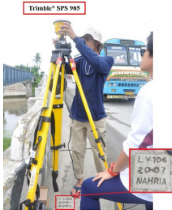
Figure 32. GNSS base set-up, Trimble® SPS 985, at LY-106, located at the approach of the Bernard Reed Bridge along Maharlika Highway, Barangay Luntad, Municipality of Palo, Leyte
