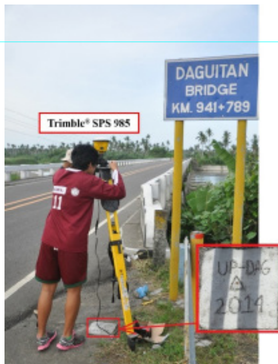
Figure 33. GNSS receiver set-up, Trimble® SPS 985, at UP DAG, an established control point, located at the bridge approach of the Daguitan Bridge along Maharlika Highway in Barangay Fatima, Municipality of Dulag, Leyte
