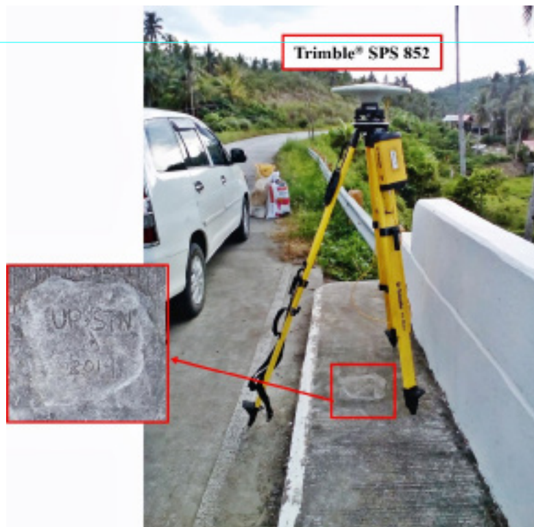
Figure 35. GNSS base set-up, Trimble® SPS 852, at UP-STN, an established control point, located at the Pagbanganan Bridge approach in Barangay Poblacion Zone 12, City of Baybay, Leyte
