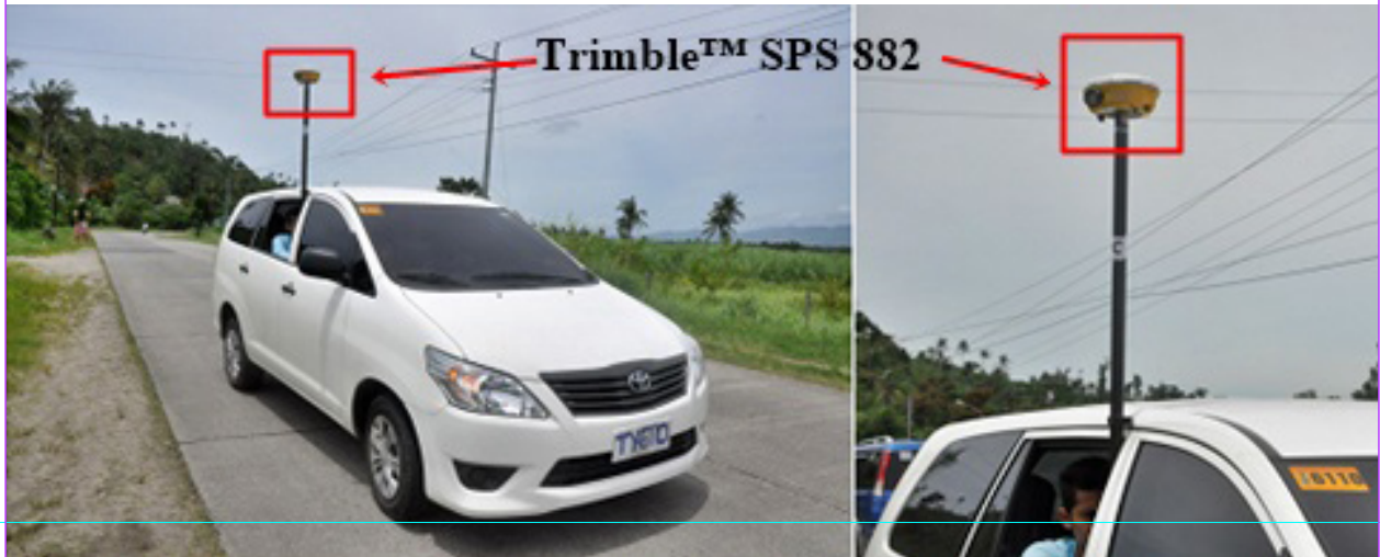
Figure 40. Ground validation set-up: a Trimble® SPS 882, mounted on a 2-meter pole and attached on the side of the vehicle
