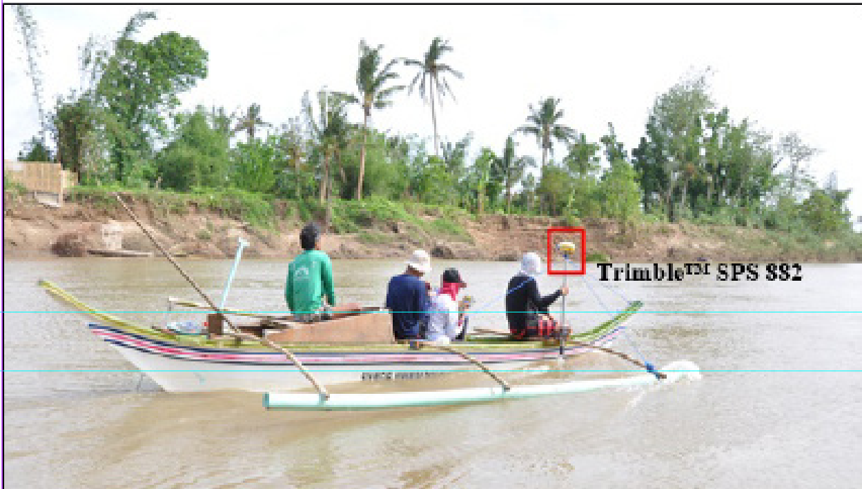
Figure 44. Bathymetry set-up using Ohmex™ Single Beam Echo Sounder with Trimble® SPS 882
