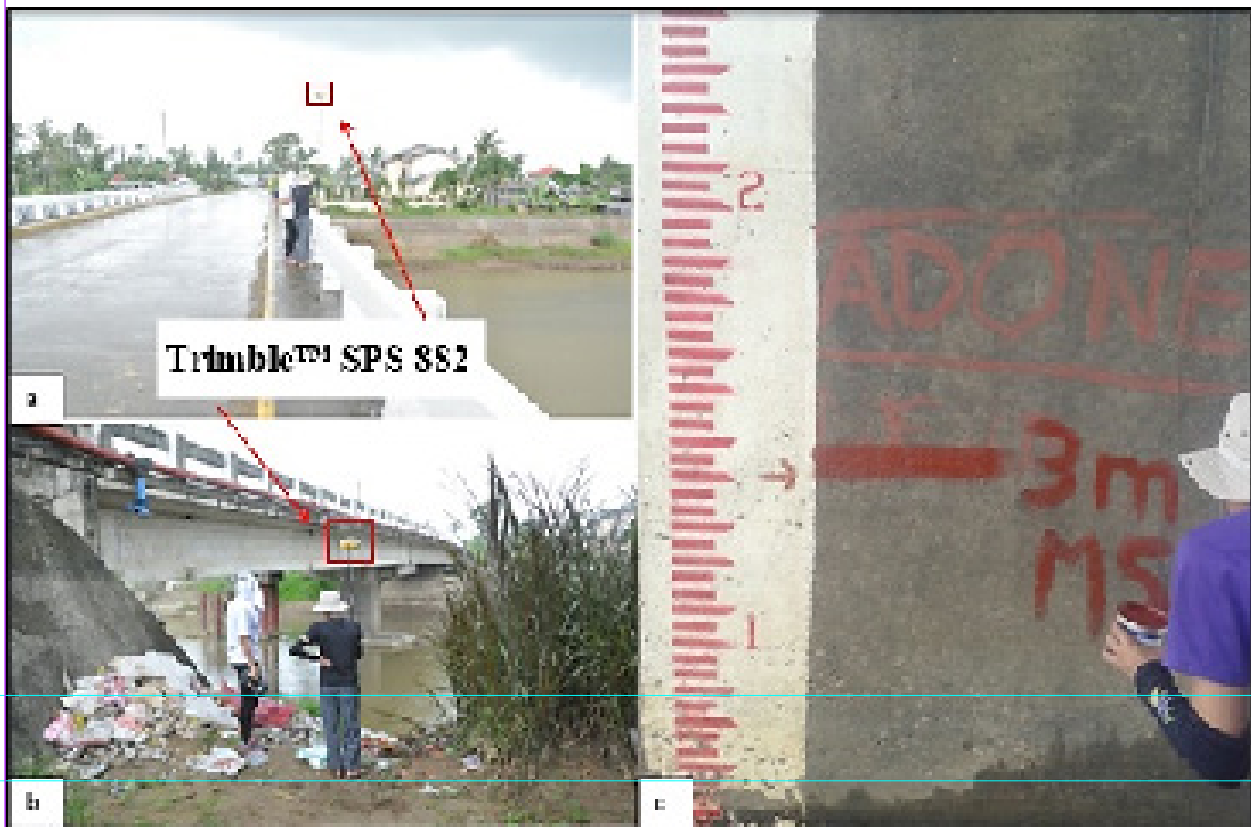
Figure 36. (a) Acquisition of water surface elevation (b) cross Section survey using Trimble® SPS 882 at Pagsangahan Bridge in City of Ormoc and (c) water level marking of bridge pier for Pagsangahan River
