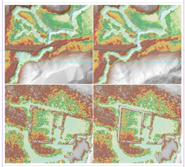
Figure 18. Portions in the DTM of Oras floodplain – a bridge before (a) and after (b) manual editing; a paddy field before (c) and after (d) data retrieval; and a building before (a) and after (b) manual editing.
