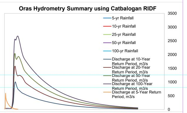
Figure 60. Outflow hydrograph at Oras Station generated using Catbalogan RIDF simulated in HEC-HMS
