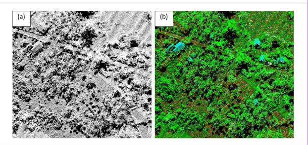
Figure 14. Point cloud before (a) and after (b) classification.
