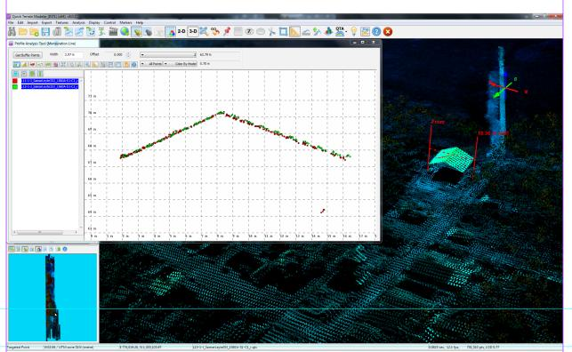
Figure 12. Quality checking for a Oras flight 1560A using the Profile Tool of QT Modeler.
