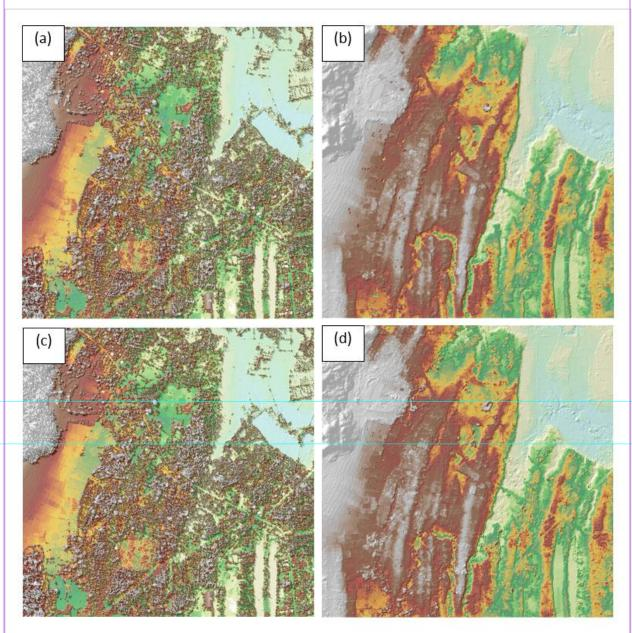
Figure 15. The Production of last return DSM (a) and DTM (b), first return DSM (c) and secondary DTM (d) in some portion near Oras floodplain.
