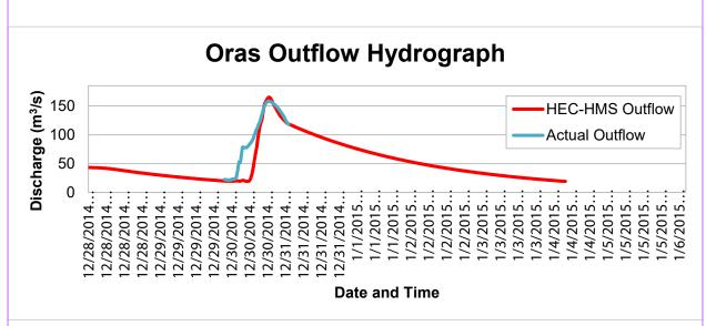
Figure 59. Outflow Hydrograph of Oras Bridge generated in HEC-HMS model compared with observed outflow
