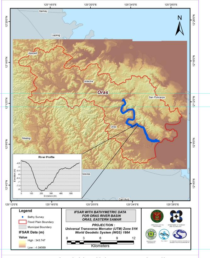
Figure 23. Map of Oras Flood Plain with bathymetric survey points shown in blue.
