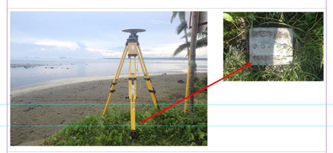
Figure 2. GPS set-up over SME-3139 located along the highway in Brgy. Sto. Nino, Oras, Eastern Samar (a) and NAMRIA reference point SME-3139 (b) as recovered by the field team.
