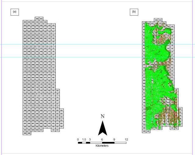
Figure 13. Tiles for Oras floodplain (a) and classification results (b) in TerraScan.
