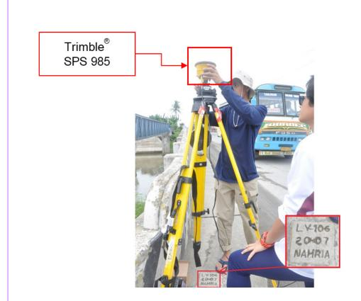
Figure 37. GNSS receiver setup, Trimble® SPS 985 at LY-106, located at the approach of Bernard Reed Bridge in Brgy. San Miguel, Municipality of Palo, Leyte
