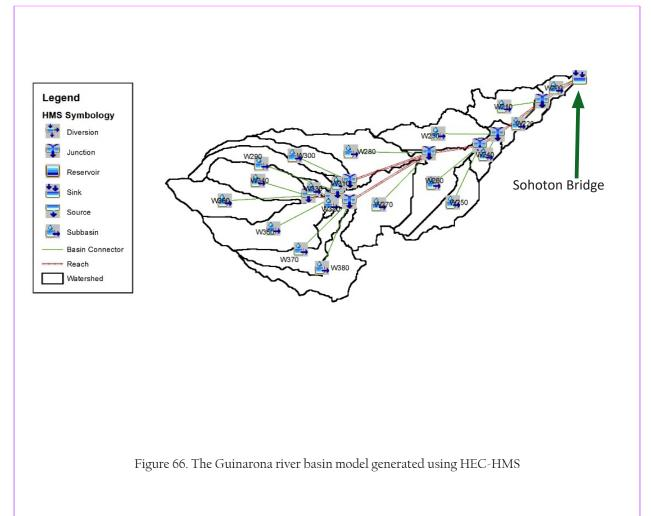
Using the SAR-based DEM, the Guinarona basin was delineated and further subdivided into subbasins. The model consists of 19 sub basins, 9 reaches, and 9 junctions as shown in Figure 66. The main outlet is at Sohoton Bridge.
