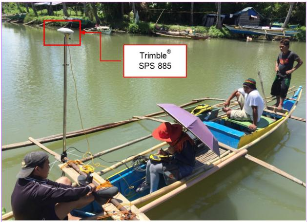
Figure 53. Bathymetric survey using a Trimble® SPS 855 in GNSS RTK survey technique in Guinarona River
