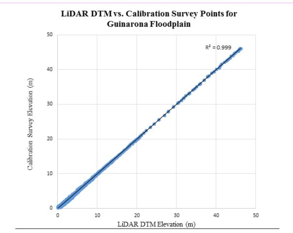
Figure 28. Correlation plot between calibration survey points and LiDAR data
