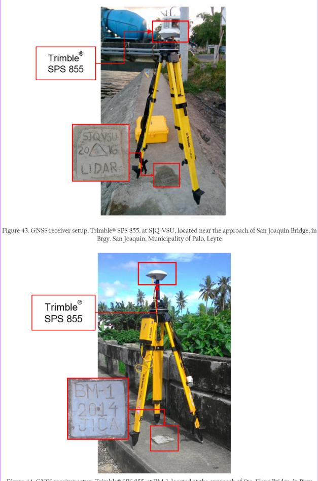
Figure 44. GNSS receiver setup, Trimble® SPS 855, at BM-1, located at the approach of Sta. Elena Bridge, in Brgy. Binongtoan, Municipality of Tanauan, Leyte
