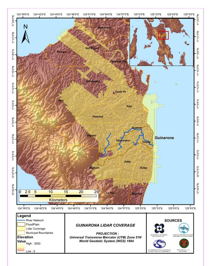
Figure 10. Actual LiDAR survey coverage for Guinarona floodplain
