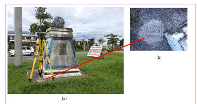
Figure 9. (a) GPS set-up over LY-881 located at the concrete foundation of Governor Center Welcome sign at the junction of the road going to Ormoc, Samar, Tacloban and MacArthur Landing Memorial Park in Brgy. Pawing, Palo, Leyte and (b) NAMRIA reference point L
