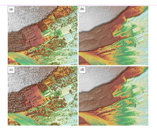
Figure 22. The production of last return DSM (a) and DTM (b), first return DSM (c) and secondary DTM (d) in some portion of Guinarona floodplain
