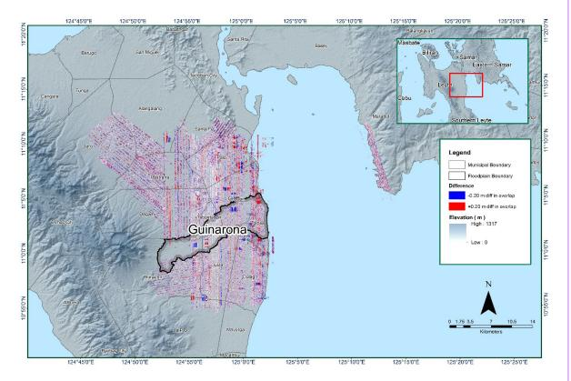
Figure 18. Elevation difference map between flight lines for Guinarona floodplain
