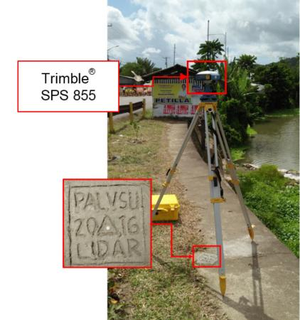
Figure 42. GNSS receiver setup, Trimble® SPS 855, at PAL-VSU, located on top of revetment along Bangon River in Brgy. Arado, Municipality of Palo, Leyte
