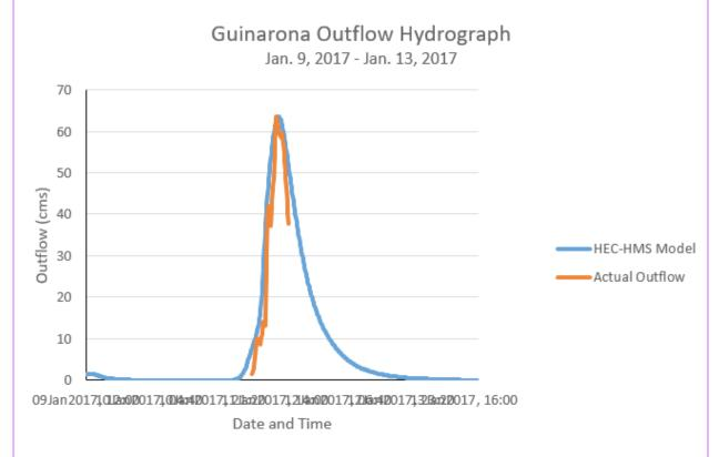
Figure 69. Outflow Hydrograph of Guinarona produced by the HEC-HMS model compared with observed outflow
