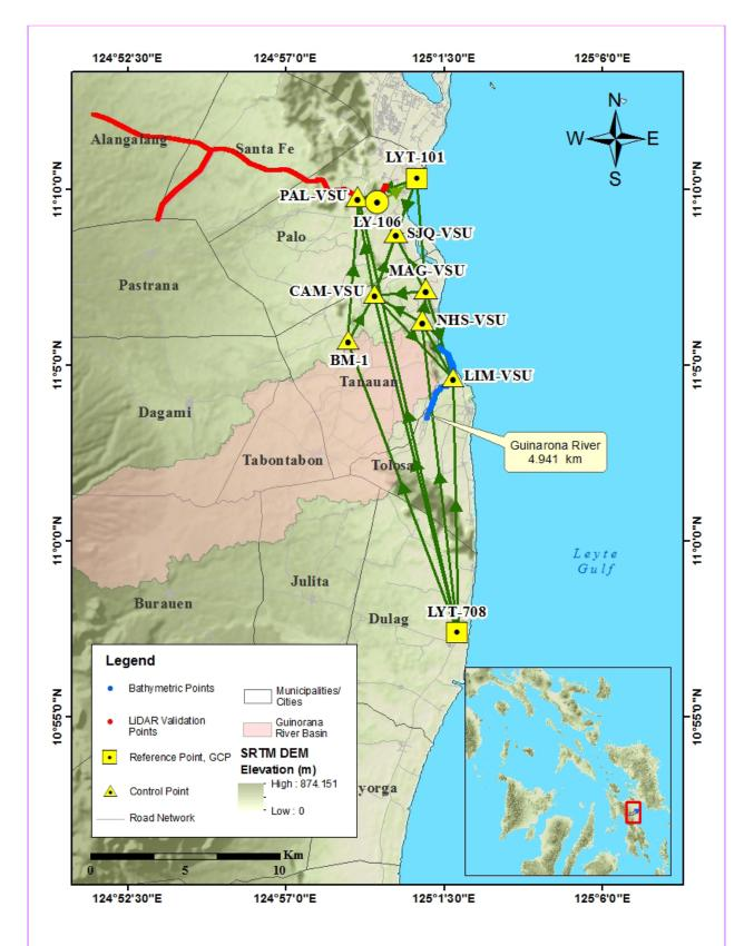
Figure 33. Extent of the bathymetric survey (in blue line) in Guinarona River and the LiDAR validation survey (red)
