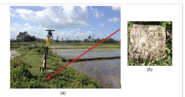
Figure 5. (a) GPS set-up over LYT-104 located and re-established along rice paddy trail, approximately 90 meters from the centerline, east side of Pastrana-Santa Fe Road, District IV, Pastrana, Leyte and (b) NAMRIA reference point LYT-104 as recovered by the field team
