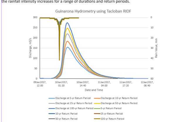
Administration (PAG-ASA) data. The simulation results reveal significant increase in outflow magnitude as the rainfall intensity increases for a range of durations and return periods.
