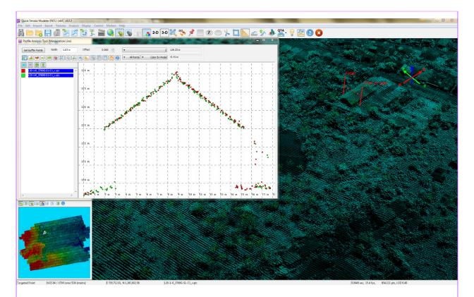
Figure 19. Quality checking for a Guinarona flight 3769G using the Profile Tool of QT Modeler
