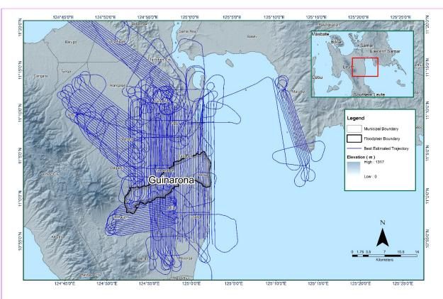
Figure 14. The best estimated trajectory of the LiDAR missions conducted over the Guinarona floodplain
