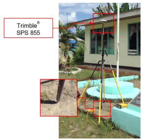
Figure 38. GNSS receiver setup, Trimble® SPS 885, at CAM-VSU, located in front of Camire Elementary School in Brgy. Balud, Municipality of Tanauan, Leyte
