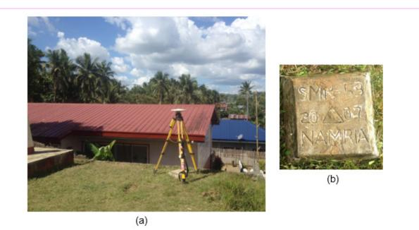
Figure 6. (a) GPS set-up over SMR-53 located near the school building flag pole of San Isidro Elementary, Brgy. San Isidro, Santa Rita and (b) NAMRIA reference point SMR-53 as recovered by the field team
