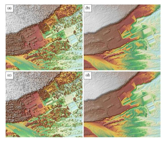
Figure 25. Portions in the DTM of Guinarona floodplain – a bridge before (a) and after (b) manual editing and a road before (c) and after (d) data retrieval
