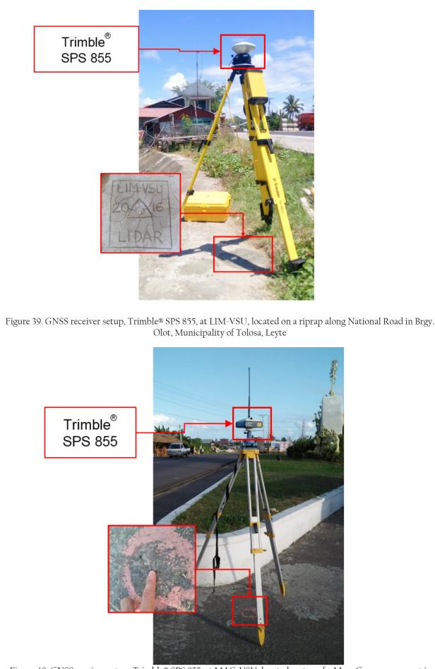
Figure 40. GNSS receiver setup, Trimble® SPS 855, at MAG-VSU, located on top of a Mass Grave monument in Brgy. Solano, Municipality of Tanauan, Leyte
