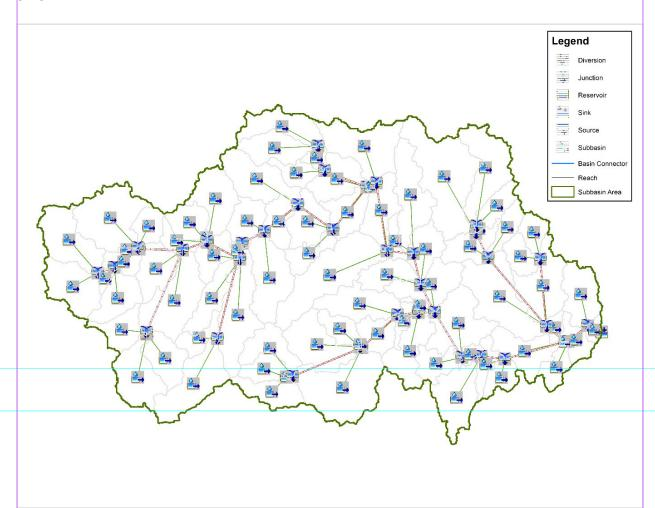
Figure 55. The Dolore river basin model generated using HEC-HMS
