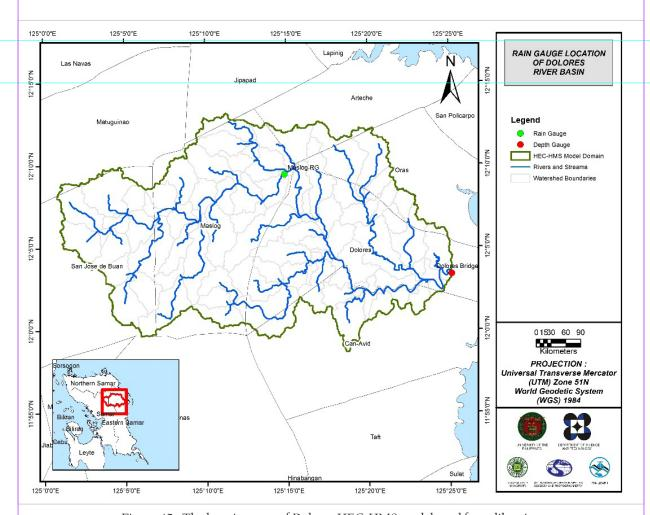
Figure 45. The location map of Dolores HEC-HMS model used for calibration
