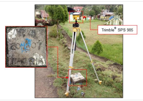
Figure 27. GNSS base set up, Trimble® SPS 985, at SMR-41, located 20 m SW from the flagpole in Bagacay Elementary School playground in Brgy. Bagacay, Hinabangan, Eastern Samar
