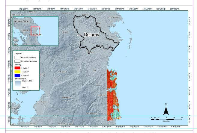
Figure 11. Pulse density map of merged LiDAR data for Dolores Floodplain.
