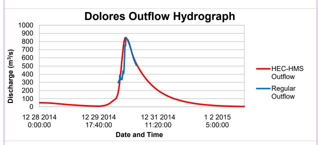
Figure 58. Outflow Hydrograph of Dolores Bridge generated in HEC-HMS model compared with observed outflow
