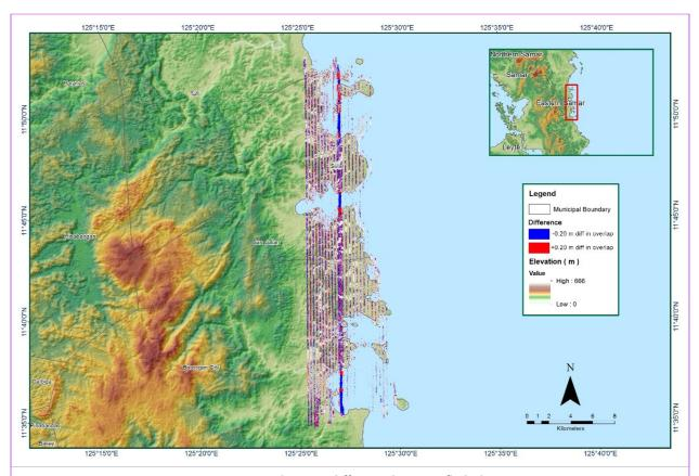
Figure A-8.7 Elevation difference between flight lines
