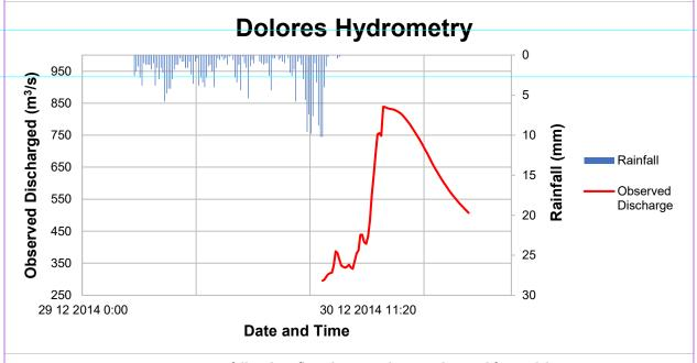
Figure 48. Rainfall and outflow data at Dolores Bridge used for modelng
