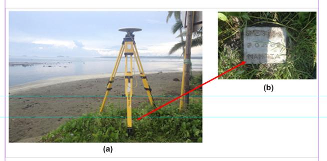
Figure 3. GPS set-up over SME-3139 located along the highway in Brgy. Sto. Nino, Dolores, Eastern Samar (a) and NAMRIA reference point SME-3139 (b) as recovered by the field team.
