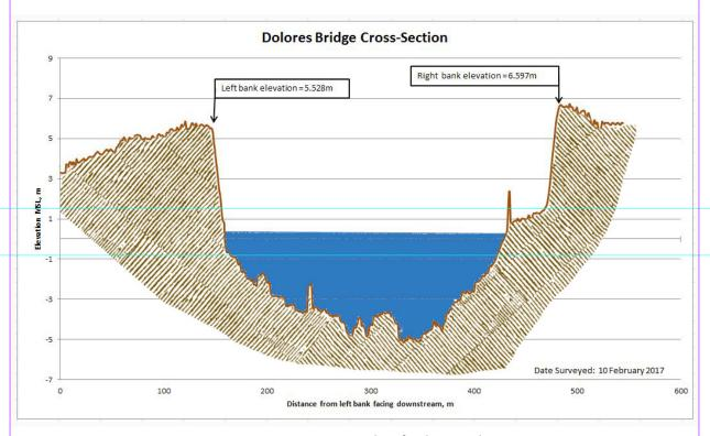
Figure 46. Cross-Section Plot of Dolores Bridge
