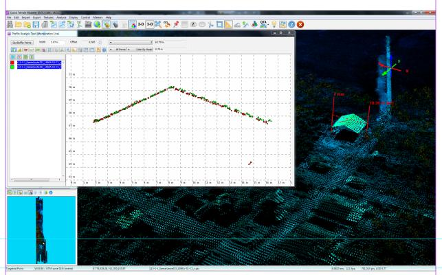
Figure 13. Quality checking for a Dolores flight 1560A using the Profile Tool of QT Modeler.
