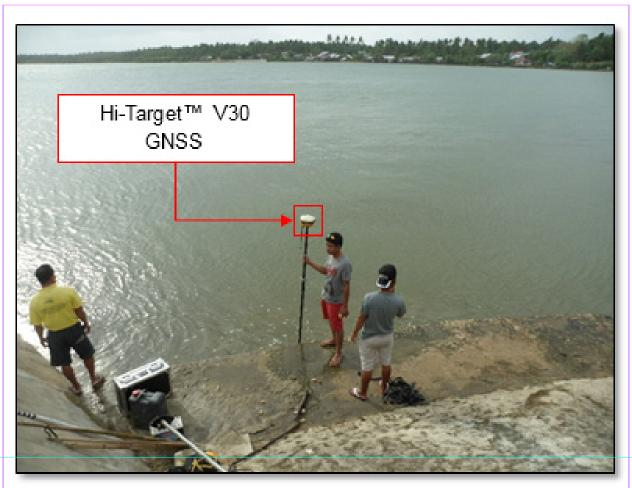
Figure 31. As-built survey of Dolores Bridge
