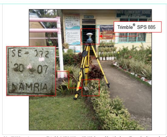
Figure 28. GNSS receiver set up, Trimble® SPS 885, at SE-172, located beside the walkway leading to the office of Nato Elementary School in Brgy. Nato, Taft, Eastern Samar
