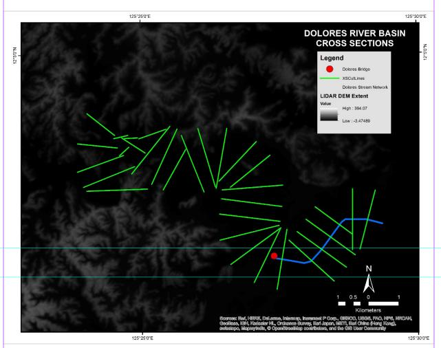
Figure 56. River cross-section of Dolores River generated through ArcMap HEC GeoRAS tool
