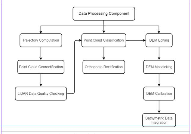
Figure 5. Schematic diagram for the Data Pre-Processing Component
