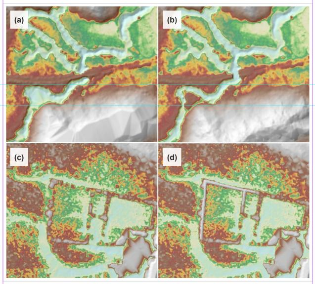
Figure 19. Portions in the DTM of Dolores Floodplain – a bridge before (a) and after (b) manual editing; and a paddy field before (c) and after (d) data retrieval.
