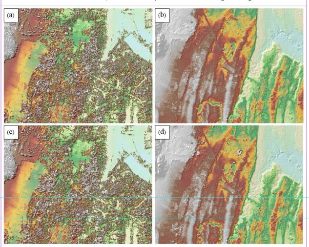
Figure 16. The Production of last return DSM (a) and DTM (b), first return DSM (c) and secondary DTM (d) in some portion near Dolores Floodplain.
