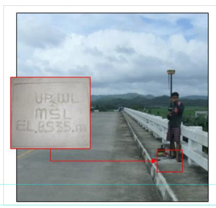
Figure 36. Water surface elevation marking on Dolores Bridge sidewalk
