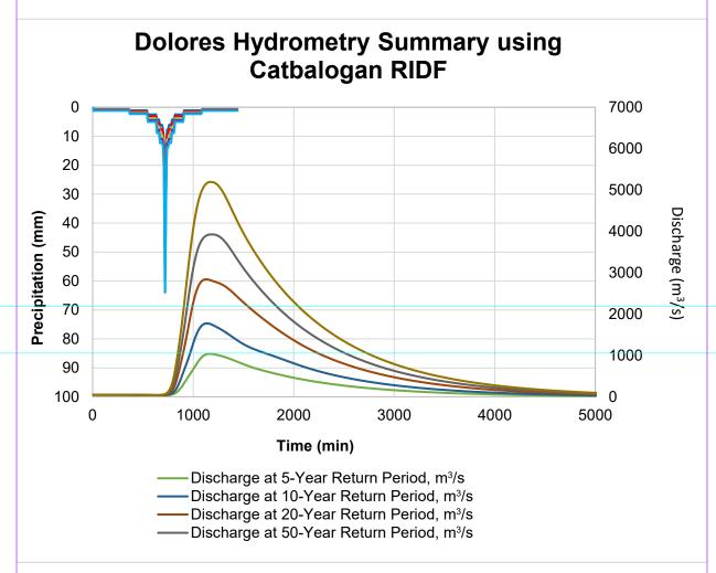
Figure 59. Outflow hydrograph at Dolores Station generated using Catbalogan RIDF simulated in HEC-HMS
