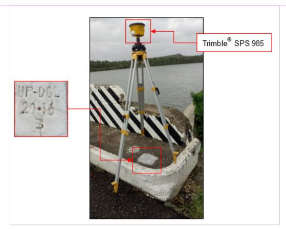
Figure 29. GNSS receiver set up, Trimble® SPS 985, at UP-DOL-3, located at the approach of Dolores Bridge in Brgy. 1 (Poblacion), Dolores, Eastern Samar
