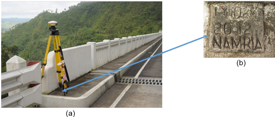
Figure 4. GPS set-up over LY-1024 located at the SE end of the sidewalk of Agas-agas Bridge at KM post 1006 + 972.6 and 4 meters from the road centerline (a); and NAMRIA reference point LY-1024 (b) as recovered by the field team.
