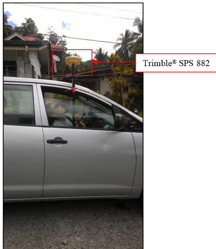
Figure 39. GNSS Receiver Trimble® SPS 882 installed on a vehicle for Ground Validation Survey.
