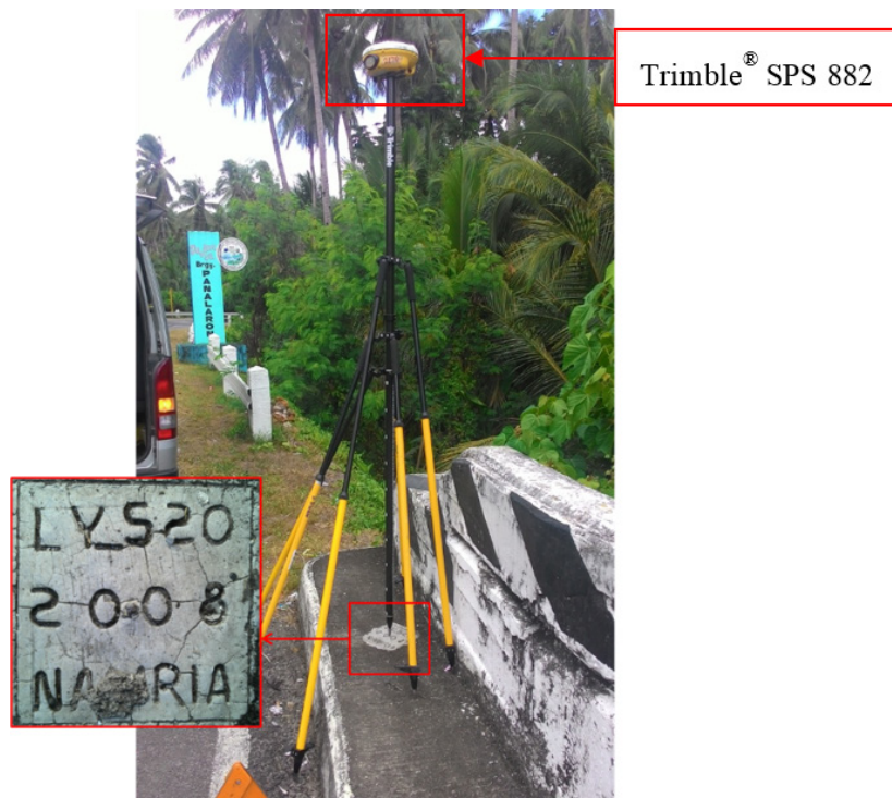
Figure 34. GNSS base set up, Trimble® SPS 882, at LY-520, located along the approach of Das-Ay Bridge in Brgy. Labrador, Hinunangan, Southern Leyte.
