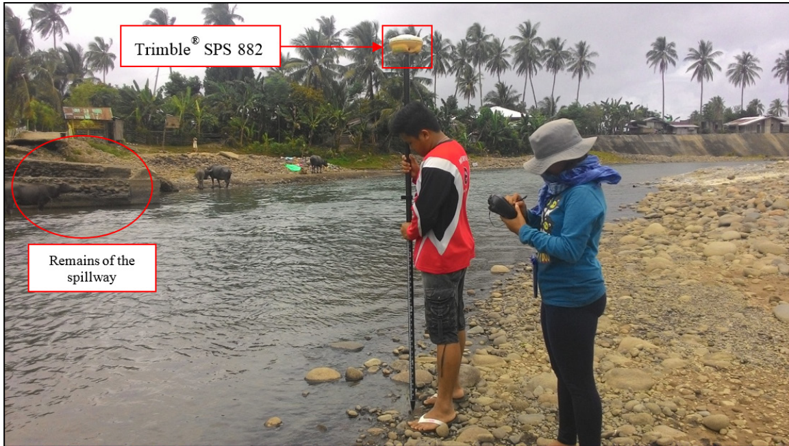
Figure 36. Cross-section survey conducted at Das-ay Bridge.
