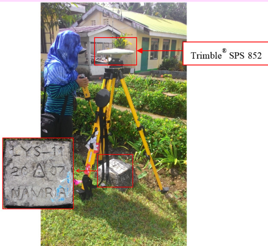
Figure 35. GNSS base set up, Trimble® SPS 852, at LYS-11, located at the St. Bernard Elementary School Grounds, Brgy. Cabagawan, St. Bernard, Southern Leyte.
