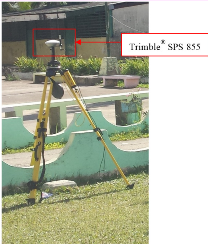
Figure 31. GNSS base set up, Trimble® SPS 855, at SMR-3024A, located at the approach of the entrance gate of Canticum Elementary School in Brgy. Canticum, Municipality of Calbiga, Samar
