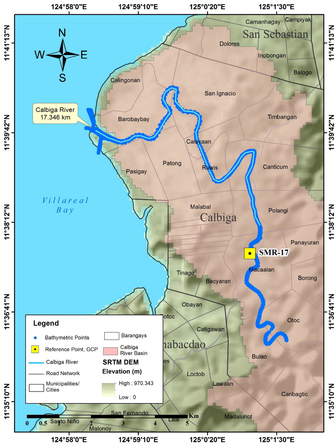
Figure 39. Bathymetric survey of Calbiga River
