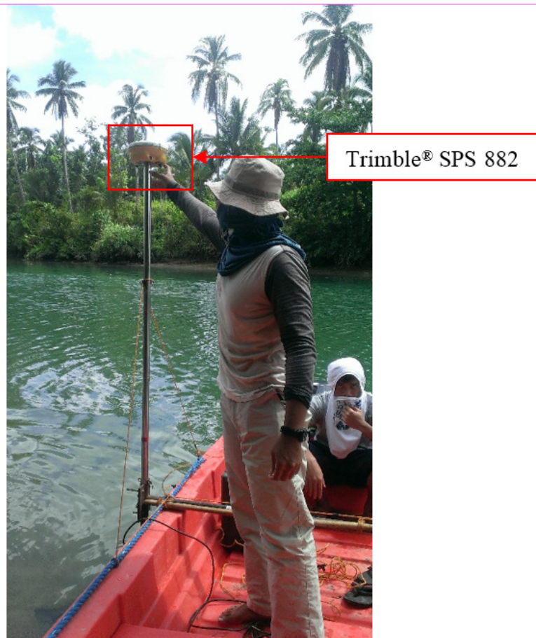
Figure 38. Bathymetry by boat set up for Calbiga River survey
