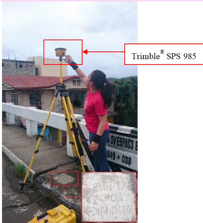
Figure 29. GNSS base set up, Trimble® SPS 985, at SMR-17, located in Brgy. Macaalan, Municipality of Calbiga, Samar
