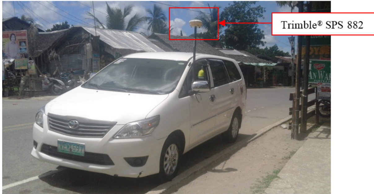
Figure 36. Validation points acquisition survey set up
