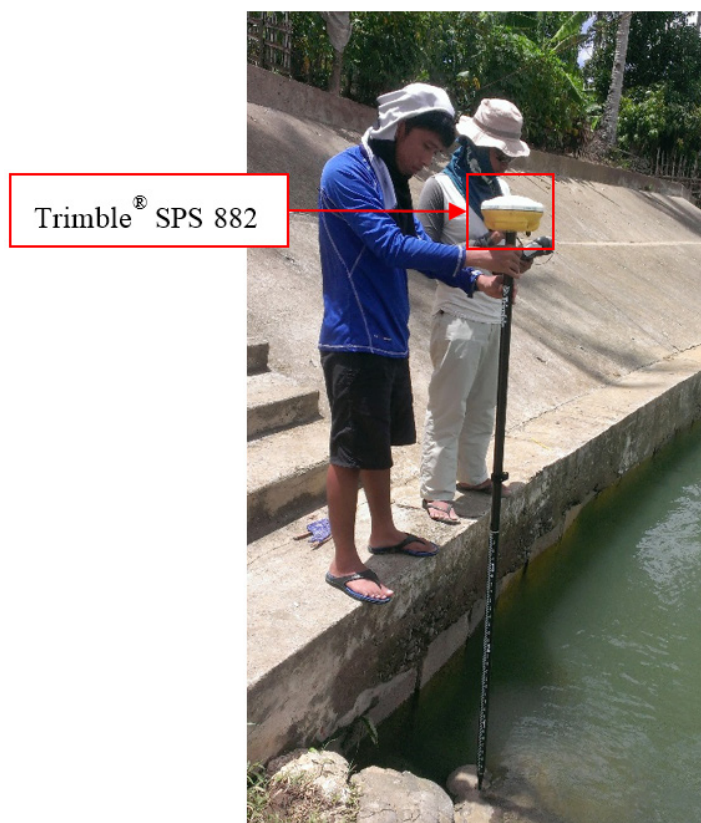
Figure 33. Cross-Section Survey for Calbiga River
