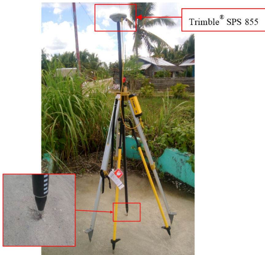
Figure 32. GNSS base set up, Trimble® SPS 855, at BARVSU, located at one of the corners of the Barangay Basketball Court in Brgy. Barobaybay, Municipality of Calbiga, Samar
