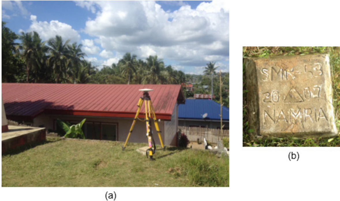
Figure 3. GPS set-up over SMR-53 located near the school building flag pole of San Isidro Elementary, Brgy. San Isidro, Santa Rita (a) and NAMRIA reference point SMR-53 (b) as recovered by the field team.
