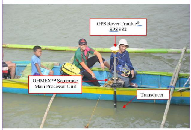
Figure 47. Bathymetric survey along Cadacan River
