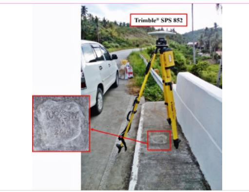
Figure 38. GNSS base set up, Trimble® SPS 852, at UP-STN, an established control point, located at Calaycalay Bridge approach in Brgy. Brgy. Poblacion Zone 12, City of Baybay, Leyte
