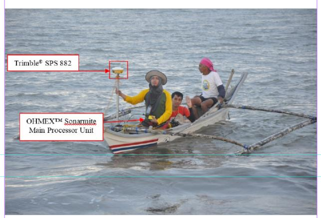
Figure 45. Bathymetric Survey for LiDAR Aquarius validation
