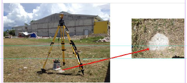
Figure 3. GPS set-up over LYT-93 as recovered within the premises of Abuyog Municipal Hall, Brgy. Sto. Abuyog, Leyte (a) and NAMRIA reference point LYT-93 (b) as recovered by the field team
