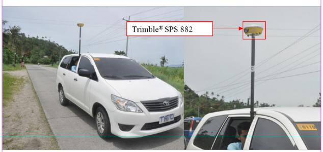
Figure 43. Validation points acquisition survey using Trimble® SPS 882 in Leyte
