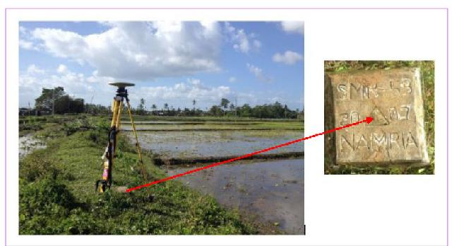
Figure 4. GPS set-up over LYT-104 as recovered and re-established along rice paddy trail, approximately 90 meters from the centerline, east side of Pastrana-Santa Fe Road, District IV, Pastrana, Leyte (a) and NAMRIA reference point LYT-104 (b) as recovered by the field team
