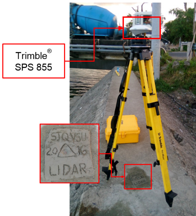
Figure 43. GNSS receiver setup, Trimble® SPS 855, at SJQ-VSU, located near the approach of San Joaquin Bridge, in Brgy. San Joaquin, Municipality of Palo, Leyte
