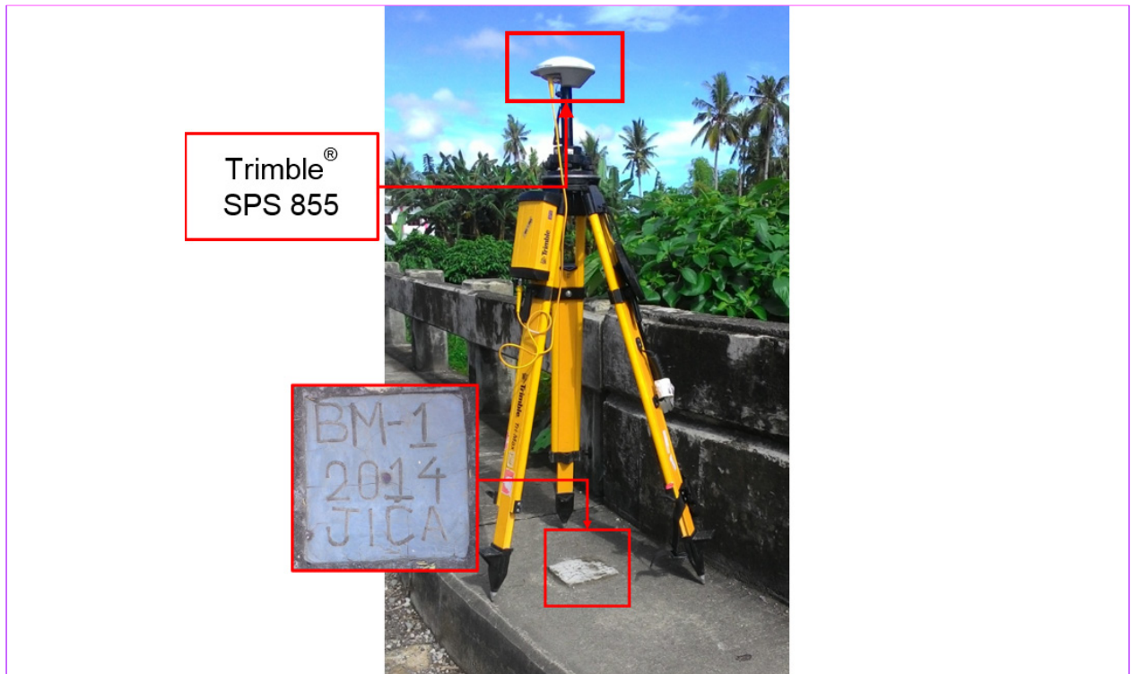
Figure 44. GNSS receiver setup, Trimble® SPS 855, at BM-1, located at the approach of Sta. Elena Bridge, in Brgy. Binongtoan, Municipality of Tanauan, Leyte
