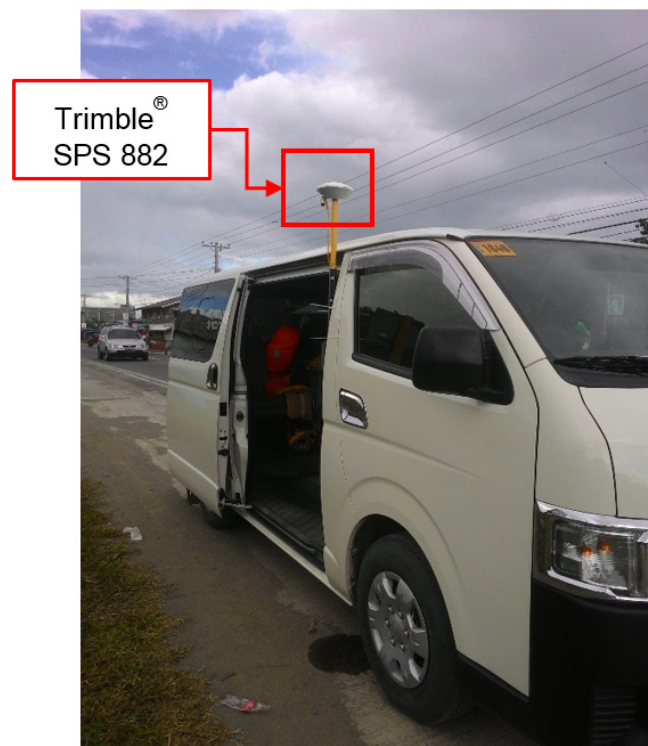
Figure 51. Validation points acquisition survey set up along Binahaan River Basin
