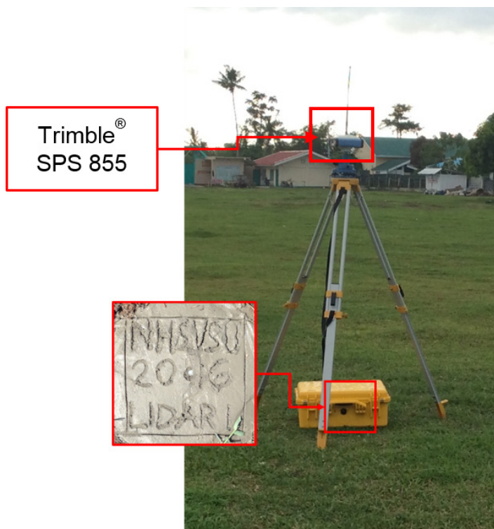
Figure 41. GNSS receiver setup, Trimble® SPS 855, at NHS-VSU, located inside Tanauan National High School, in Brgy. Sto. Niño Poblacion, Municipality of Tanauan, Leyte
