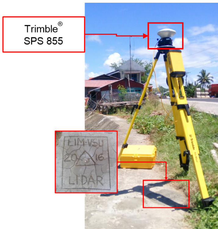
Figure 39. GNSS receiver setup, Trimble® SPS 855, at LIM-VSU, located on ariprap along National Road in Brgy. Olot, Municipality of Tolosa, Leyte
