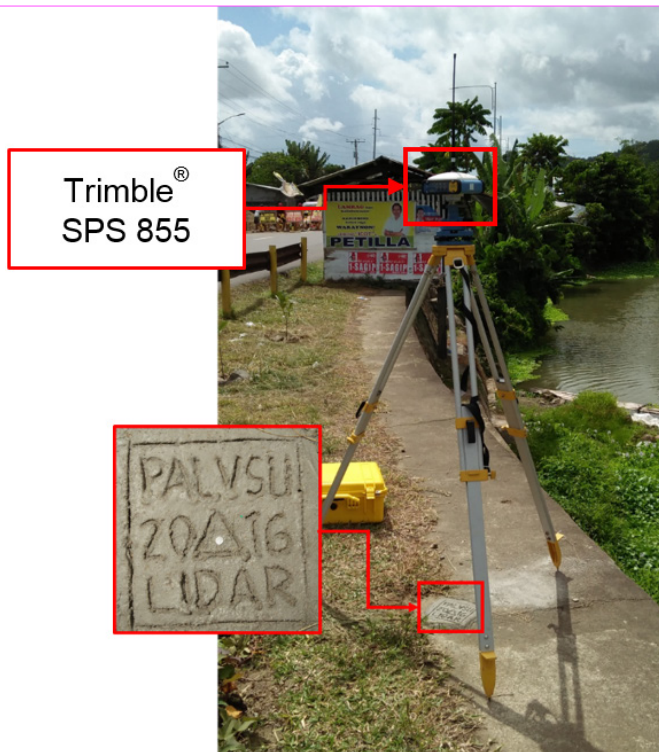
Figure 42. GNSS receiver setup, Trimble® SPS 855, at PAL-VSU, located on top of revetment along Bangon River in Brgy. Arado, Municipality of Palo, Leyte
