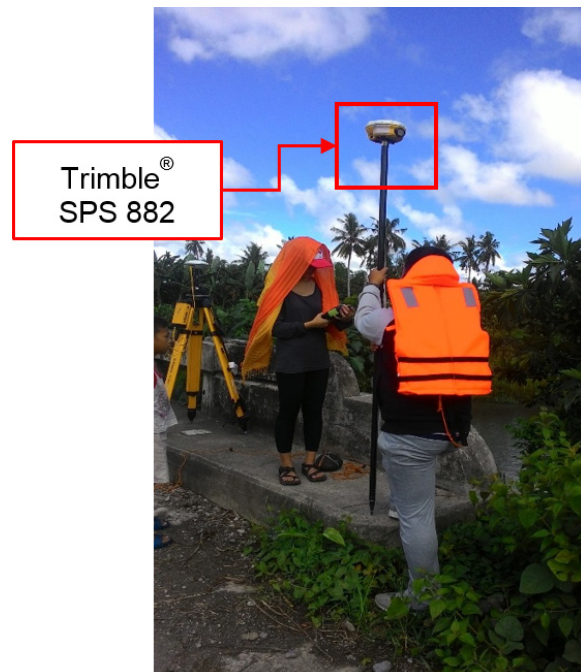
Figure 46. As-Built Survey of Sta. Elena Bridge
