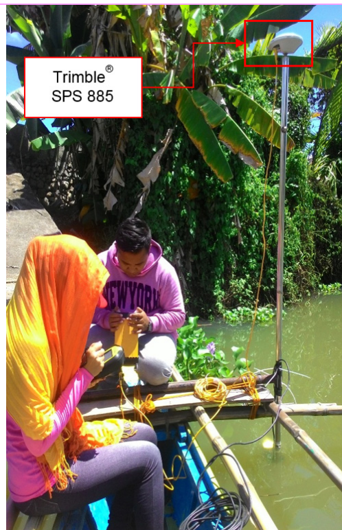
Figure 53. Bathymetric survey using a Trimble® SPS 855 in GNSS RTK survey technique in Binahaan River
