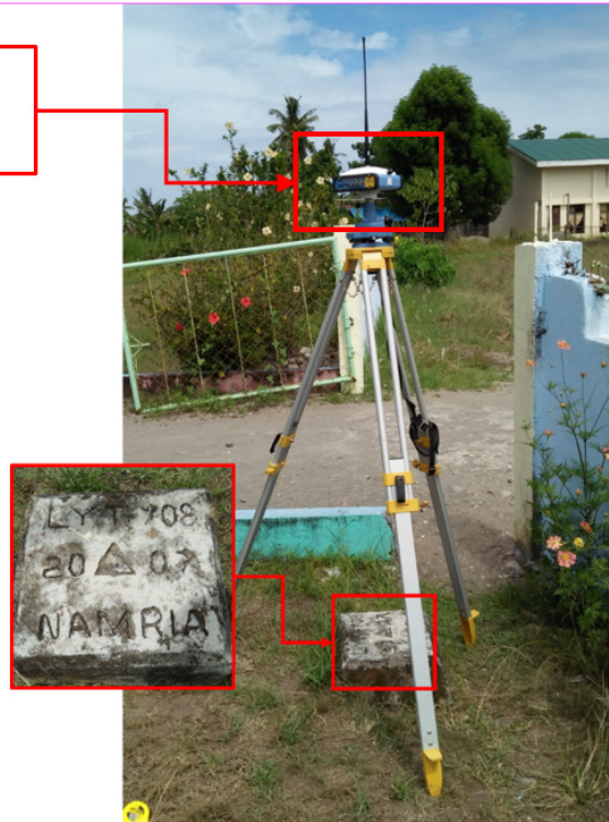
Figure 36. GNSS base set up, Trimble® SPS 855, at LYT-708, located in front of Dulag Elementary School, in Brgy. Buntay, Mun. of Dulag, Leyte
