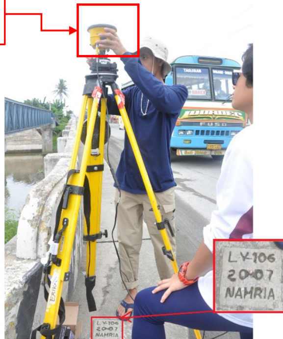
Figure 37. GNSS receiver setup, Trimble® SPS 985 at LY-106, located at the approach of Bernard Reed Bridge in Brgy. San Miguel, Municipality of Palo, Leyte
