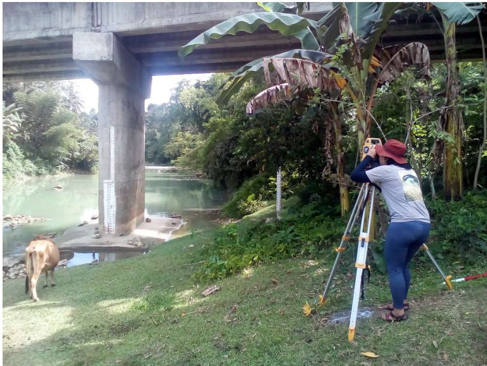
Figure 39. Cross-section survey at the downstream side of Cambanog Bridge
