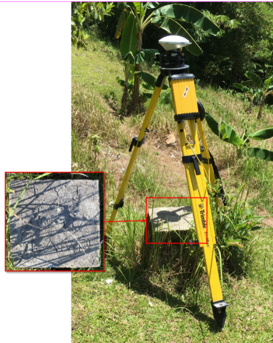
Figure 34. GNSS base set up, Trimble® SPS 852, at LYT-742, located near a chapel and basketball court in Brgy. Tambis, Municipality of Hilongos, Leyte
