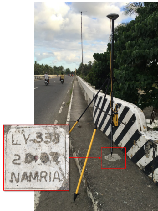
Figure 35. GNSS receiver set up, Trimble® SPS 855, at LY-338, a first-order BM, located at the approach of Salug Birdge along Sta. Indang-Hilongos Road in Brgy. San Juan, Municipality of Hilongos, Leyte
