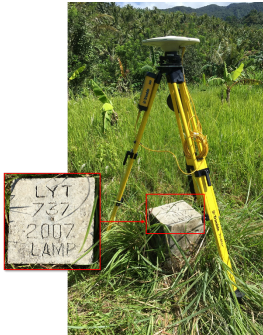
Figure 33. GNSS base set up, Trimble® SPS 852, at LYT-737, located at the back of Cabulisan Elementary School in Brgy. Cabulisan, Municipality of Inopacan, Leyte
