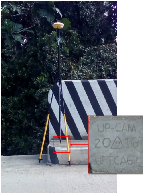
Figure 36. GNSS receiver set up, Trimble® SPS 882, at UP-CAM, an established control point, located at the approach of Cambanog Bridge in Brgy. Naga, Municipality of Bato, Leyte
