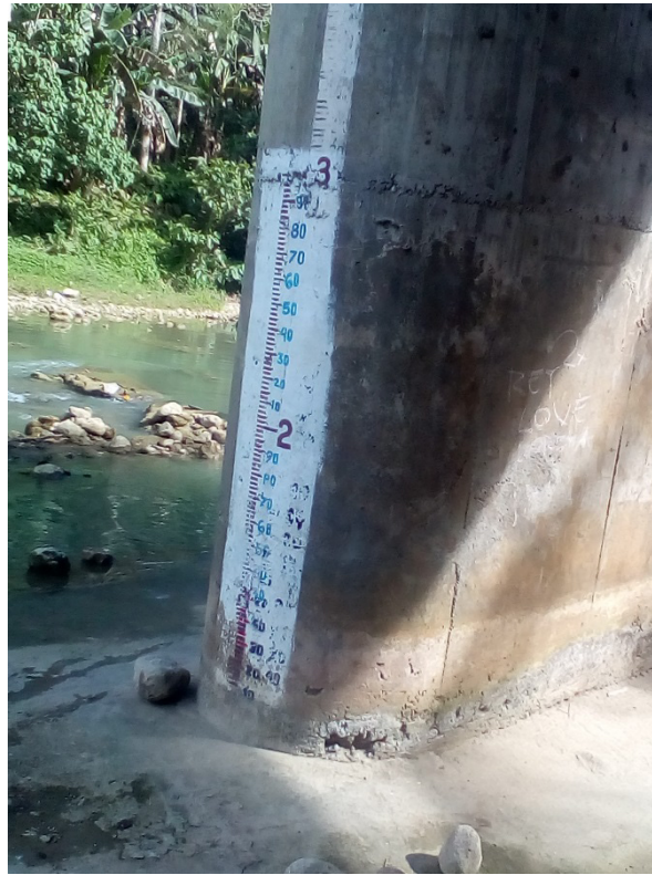
Figure 43. a) Getting the MSL elevation of the markings written on the pier and b) Water-level markings for Bangkerohan River
