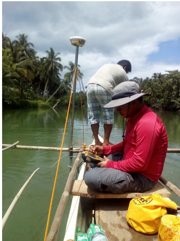
Figure 46. Bathymetry by boat set up for Bangkerohan River survey
