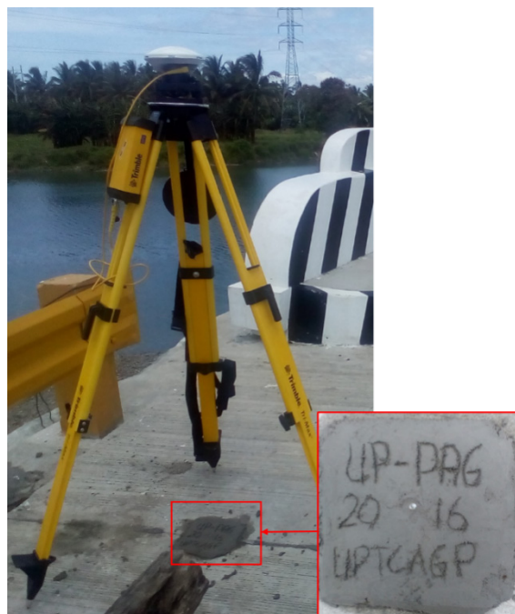
Figure 37. GNSS receiver set up, Trimble® SPS 855, at UP-PAG, an established control point, located at Pagbanganan Bridge approach in Brgy. Brgy. Poblacion Zone 12, City of Baybay, Leyte
