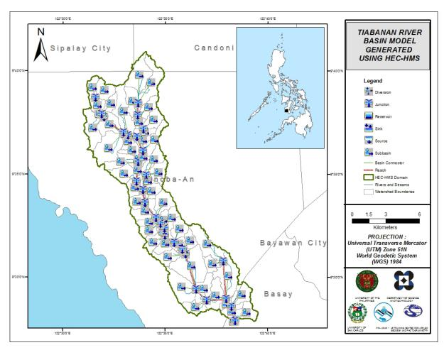
Figure 53. HEC-HMS generated Tiabanan River Basin Model.
