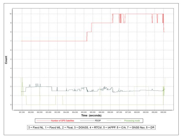
Figure 8. Solution Status Parameters of Tiabanan Flight 7578G.
