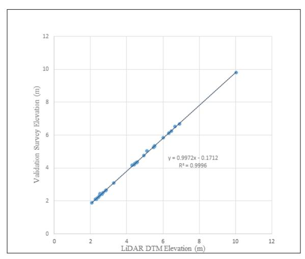
Figure 22. Correlation plot between validation survey points and LiDAR data.
