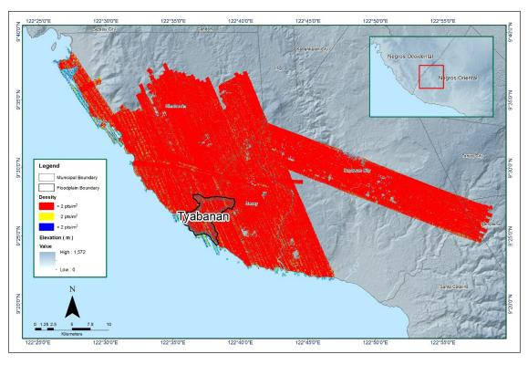
Figure 12. Pulse density map of merged LiDAR data for Tiabanan Floodplain.
