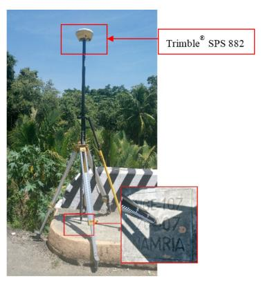
Figure 29. GNSS base set up, Trimble® SPS 882, at NE-107, a second-order GCP located at the approach of Manalongon Bridge in Brgy. Manalongon, Sta. Catalina, Negros Oriental
