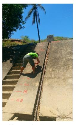
Figure 36. Water-level marking on Tiabanan River
