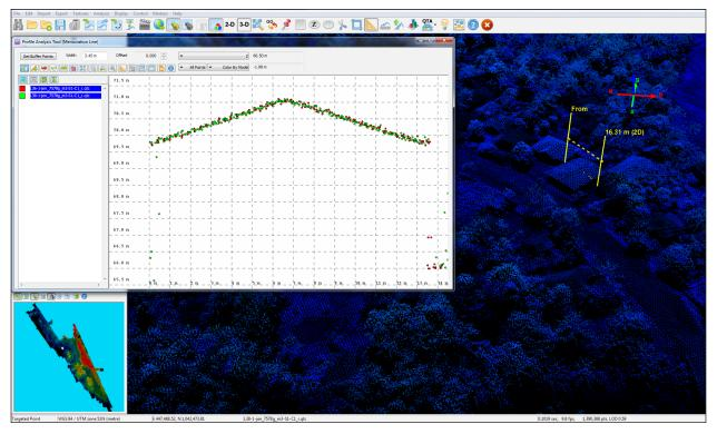
Figure 14. Quality checking for Tiabanan Flight 7578G using the Profile Tool of QT Modeler.
