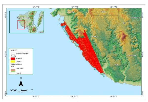
Figure A-8.13. Density of merged LiDAR data
