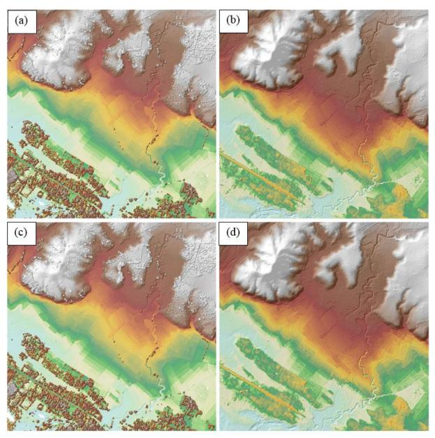
Figure 17. The production of last return DSM (a) and DTM (b), first return DSM (c) and secondary DTM (d) in some portion of Tiabanan Floodplain.
