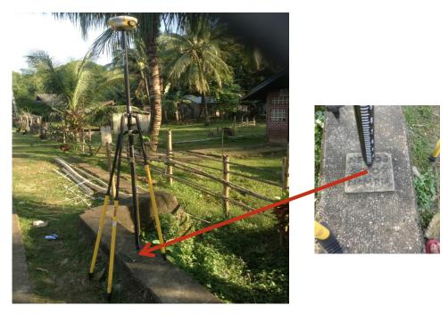
Figure 4. GPS set-up over NE-08 on top center of reinforced concrete pipe culvert about 7 meters from the roadline located in the municipality of Basay, Barangay Nagbualao along the national road going to Hinoba-An (a) and NAMRIA reference point NE-08 (b) as recovered by the field team.
