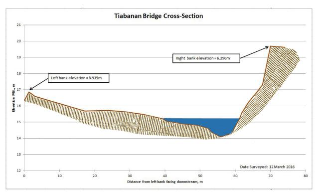
Figure 44. Cross-Section Plot of Tiabanan Bridge
