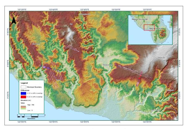
Figure A-8.7. Elevation difference between flight lines
