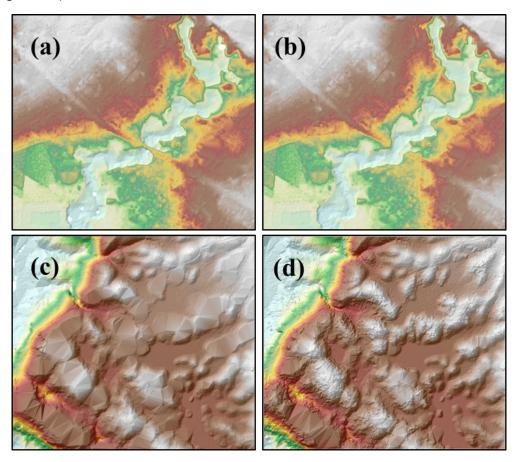
Figure 18. Portions in the DTM of Tiabanan Floodplain – a bridge before (a) and after (b) manual editing; hills before (c) and after (d) data retrieval
