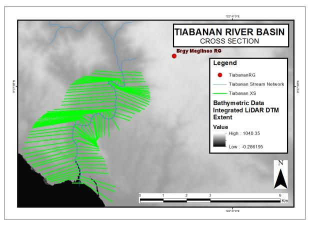
Figure 54. River cross-section of Tiabanan River generated through Arcmap HEC GeoRAS tool
