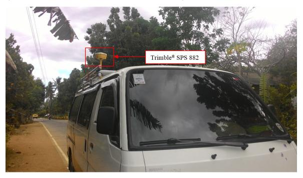
Figure 37. Validation points acquisition survey set-up
