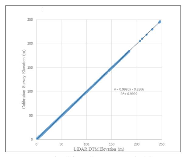
Figure 21. Correlation plot between calibration survey points and LiDAR data.
