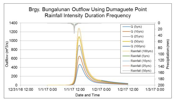
Figure 57. Outflow hydrograph at Brgy. Bungalunan, Basay generated using Dumaguete Point RIDF simulated in HEC-HMS
