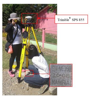
Figure 30. GNSS base set up, Trimble® SPS 855, at NE-358, a first-order BM, located on a culvert along Sta. Caalina-Bayawan Road in Brgy. Ubos, Bayawn City, Negros Oriental
