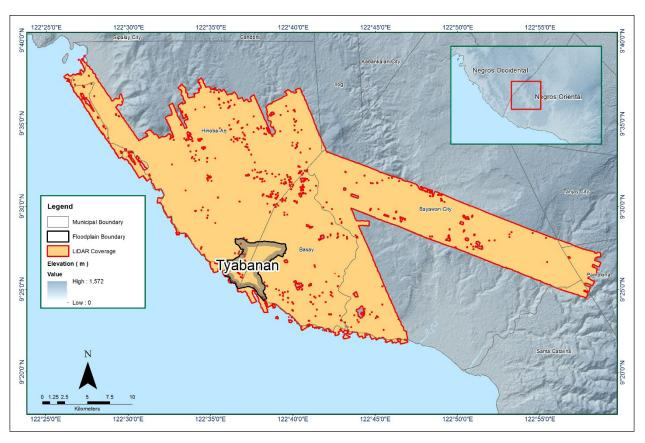
Figure 10. Figure 10. Boundary of the processed LiDAR data over Tiabanan Floodplain
