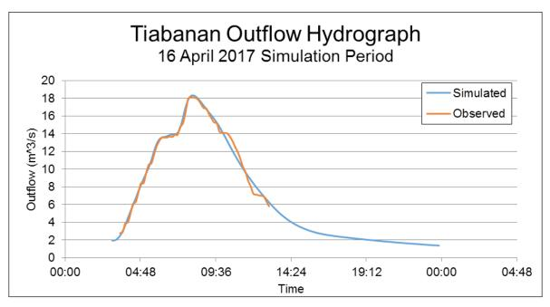
Figure 56. Outflow Hydrograph of Tiabanan produced by the HEC-HMS model compared with observed outflow.
