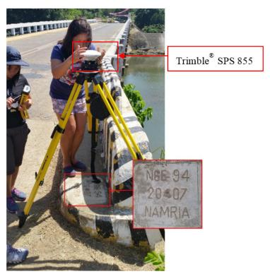
Figure 31. GNSS base set up, Trimble® SPS 855, at NGE-94, a GCP used as marker, located at the approach of Tiabanan Bridge in Brgy. Bongalonan, Basay, Negros Oriental
