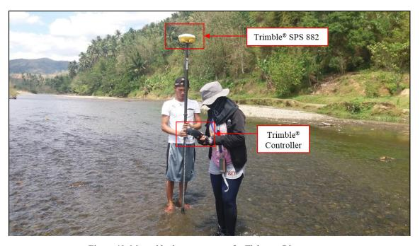
Figure 40. Manual bathymetry set-up for Tiabanan River survey
