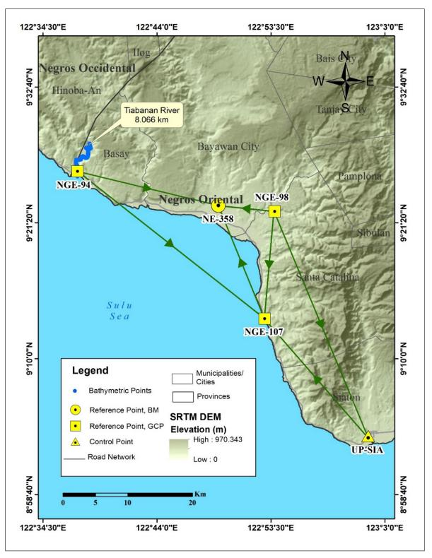
Figure 27. GNSS Network of Tiabanan River field survey
