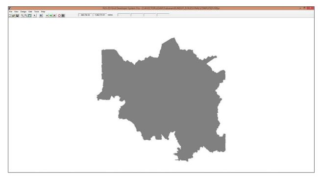
Figure 55. Screenshot of subcatchment with the computational area to be modeled in FLO-2D GDS Pro
