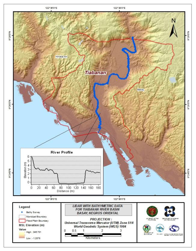
Figure 23. Map of Tiabanan Floodplain with bathymetric survey points shown in blue.
