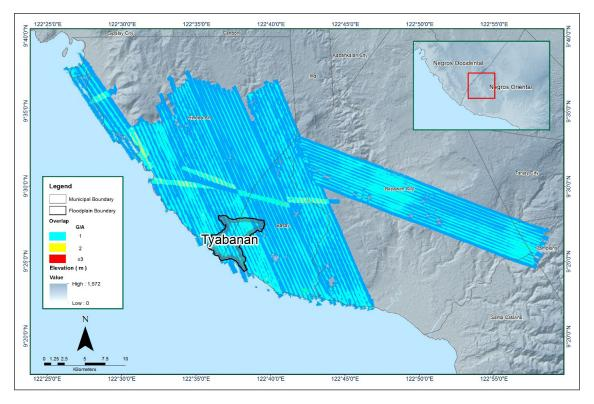
Figure 11. Image of data overlap for Tiabanan Floodplain.
