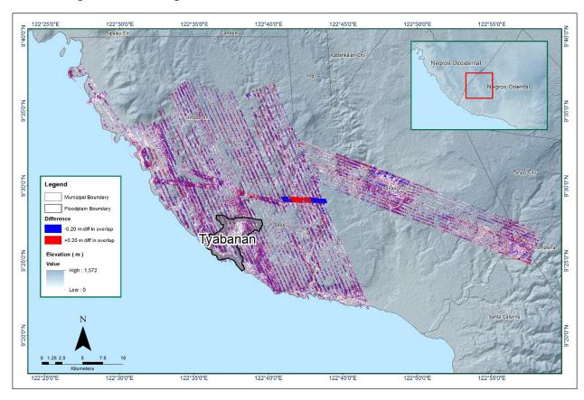
Figure 13. Elevation difference map between flight lines for Tiabanan Floodplain.
