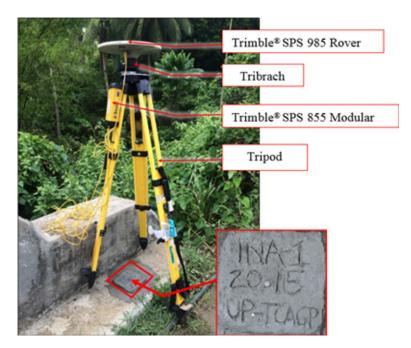
Figure 33. Trimble® SPS 985 GNSS receiver setup at INA-1 at the Inabanga Bridge approach, Brgy. Baguhan, Inabanga, Bohol
