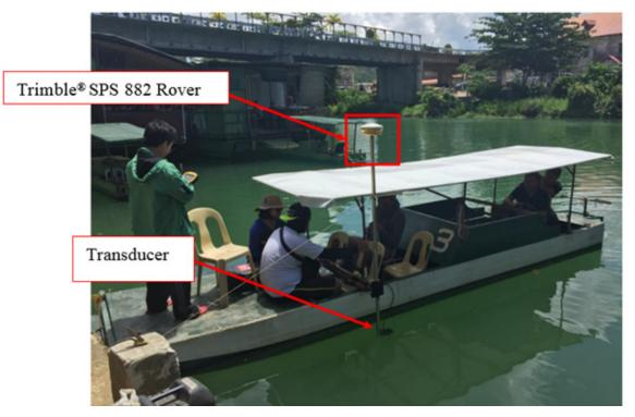
Figure 42. Bathymetric survey in Loboc River
