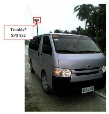
Figure 40. Trimble® SPS8 82 set-up for validation points acquisition survey for Loboc River
