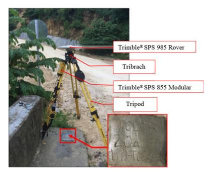
Figure 32. Trimble® SPS 985 GNSS receiver setup at control point DOLOR, located at the left most (facing downstream) Baguhan Bridge approach, across Inabanga River located in Brgy. Dorol, Municipality of Angilan, Bohol
