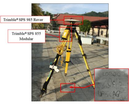
Figure 34. GPS setup of Trimble® SPS 852 on LOBOC, located on the incomplete bridge across the Loboc River near the municipality town plaza of Loboc in Brgy. Poblacion
