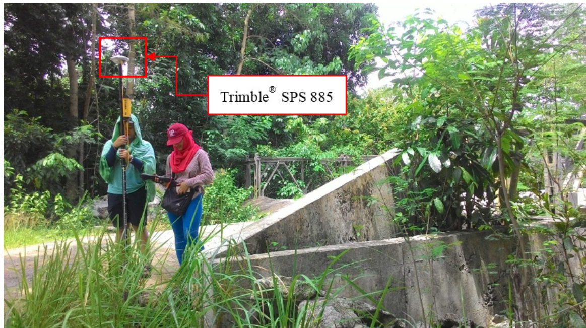
Figure 37. Bridge As-Built Survey using PPK Technique in Tugas Bridge
