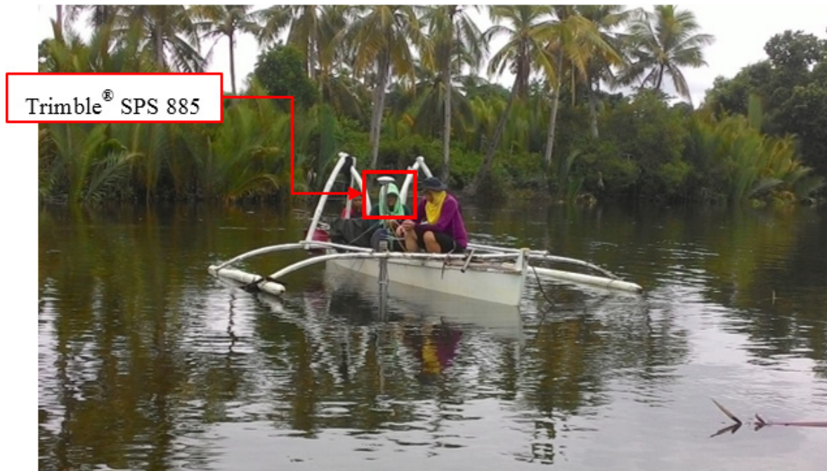
Figure 50. Bathymetric survey using OHMEX™ single beam echo sounder in Ipil River
