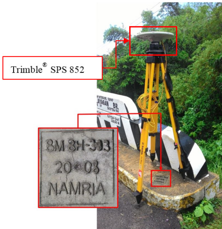
Figure 35. GNSS receiver setup, Trimble® SPS 852, at BH-393 located at the approach of Hinlayagan Bridge, Brgy. Hinlayagan Ilaya, Municipality of Trinidad, Bohol
