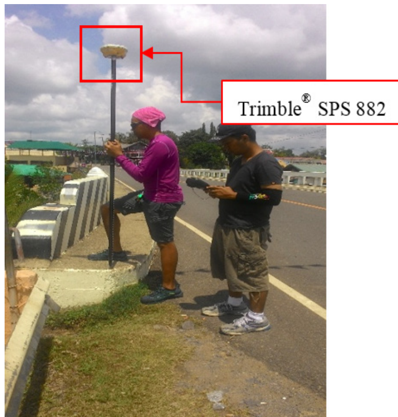
Figure 39. Bridge As-Built Survey using PPK Technique in Trinidad Bridge
