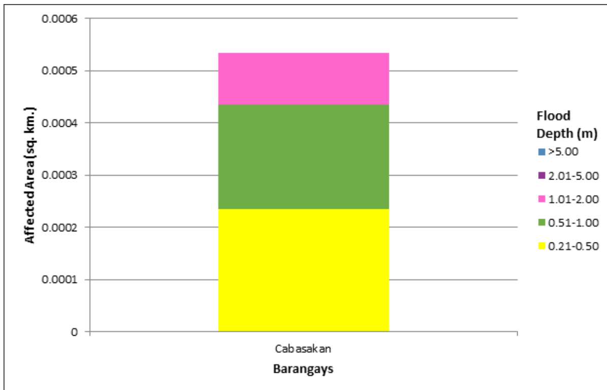
Figure 99. Affected Areas in Jetafe, Bohol during 100-Year Rainfall Return Period
