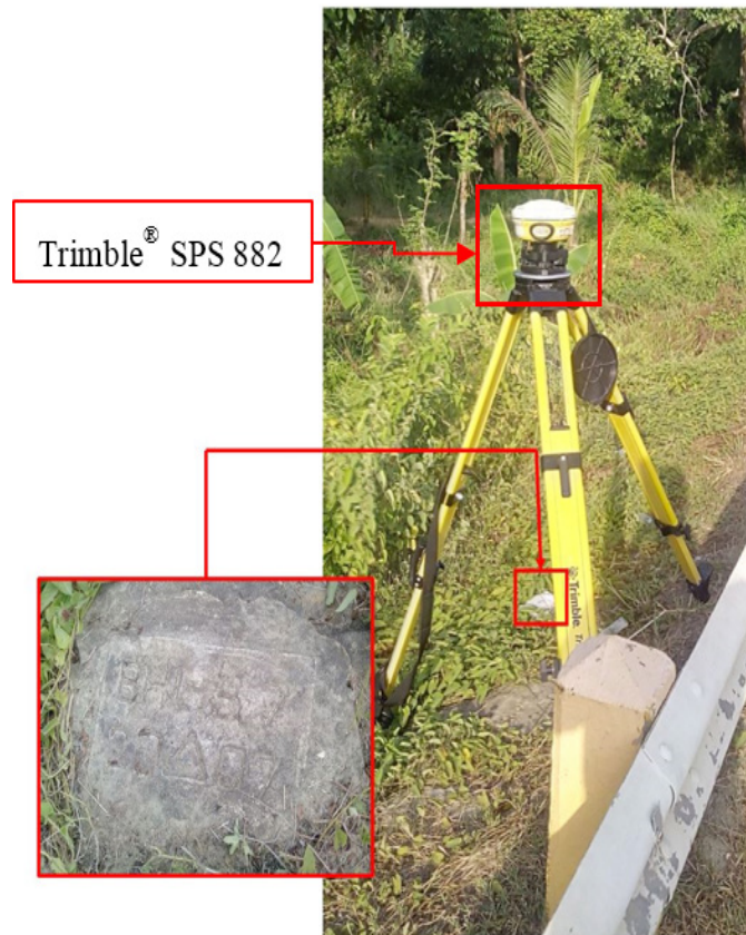
Figure 33. GNSS base set up, Trimble® SPS 882, at BHL-57 located along Ubay-Talibon Road, Brgy. Tanghaligue, Municipality of Talibon, Bohol
