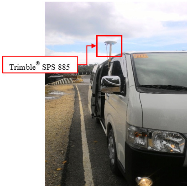
Figure 48. Validation points acquisition survey set up along Ipil River Basin
