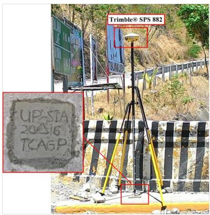
Figure 39 GNSS receiver set up, Trimble® SPS 882, at UP-SIA, an established control point, located at the approach of Siaton Bridge in Brgy. Caticugan, Siaton, Negros Oriental
