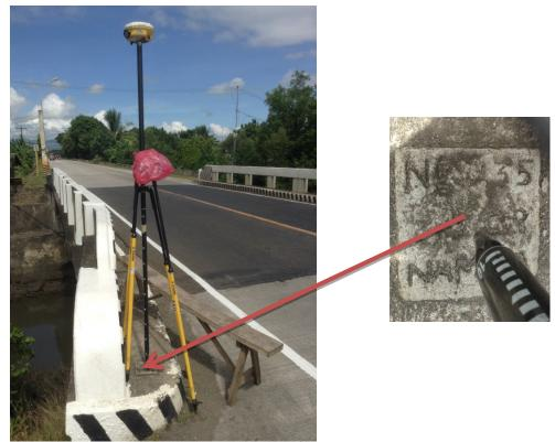
Figure 9 GPS set-up over NE-135 in Busuang Bridge on top of concrete sidewalk in Barangay Bio-os under the Municipality of Amlan (a) and NAMRIA benchmark NE-135 (b) as recovered by the field team.
