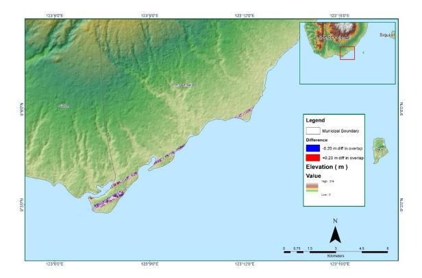
Figure A-8.28 Elevation Difference Between flight lines
