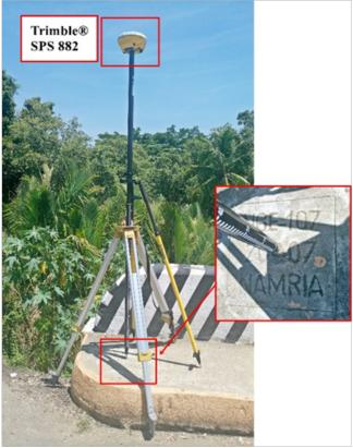
Figure 36 GNSS receiver set up, Trimble® SPS 882, at NGE-107, a second order GCP located at the approach of Manalongon Bridge, in Brgy. Manalongon, Sta. Catalina, Negros Oriental
