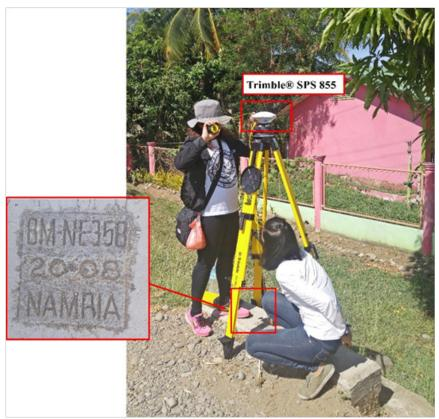
Figure 37 GNSS base set up, Trimble® SPS 855, at NE-358, a first-order BM, located on a culvert along Sta. Caalina-Bayawan Road in Brgy. Ubos, Bayawn City, Negros Oriental
