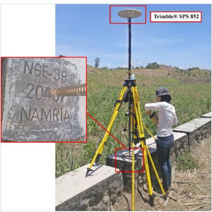
Figure 35 GNSS base set up, Trimble® SPS 852, at NGE-98 a second-order GCP located on top of a concrete block along Sta. Catalia-Pamplona Provincial Road, in Brgy. Caranoche, Sta. Catalina, Negros Oriental
