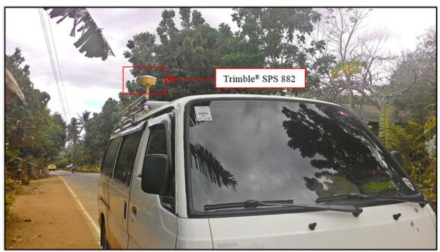
Figure 43 Validation points acquisition survey set-up
