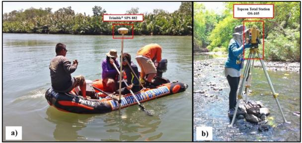
Figure 45 a) Bathymetry by boat set up with mounted Trimble® SPS 882 and b) manual bathymetry using Topcon Total Station OS-105 for Canaway River survey
