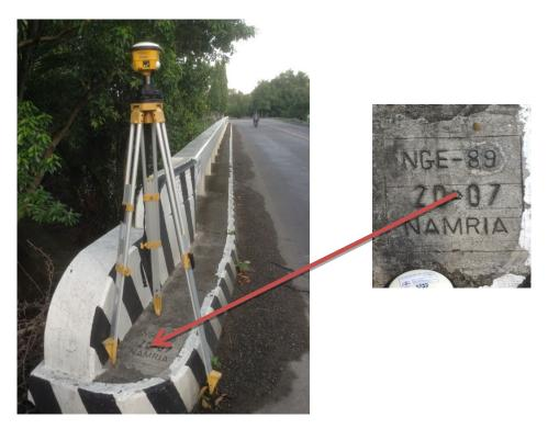
Figure 4 GPS set-up over NGE-89 at the SE corner of Bio-os Bridge in Barangay Bio-os under the Municipality of Amlan (a) and NAMRIA reference point NGE-89 (b) as recovered by the field team
