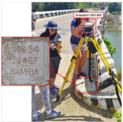
Figure 38 GNSS base set up, Trimble® SPS 855, at NGE-94, a GCP used as marker, located at the approach of Tiabanan's bridge in Brgy. Bongalonan, Basay, Negros Oriental
