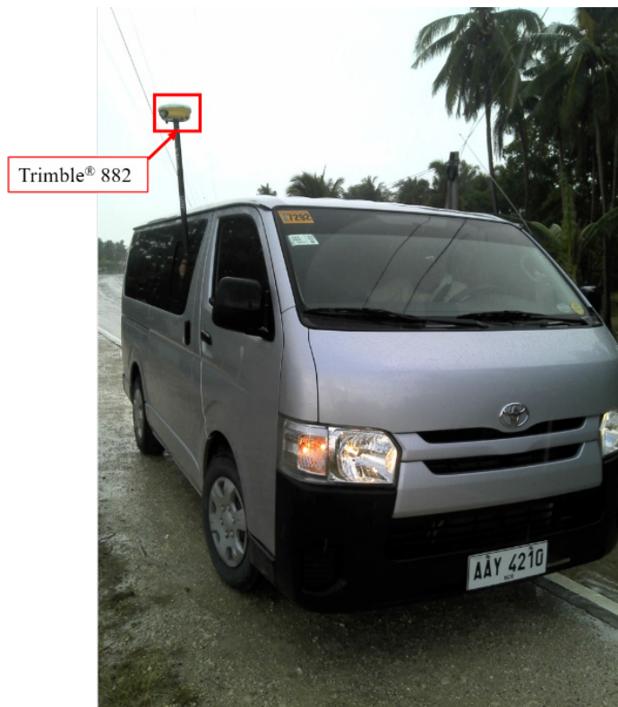
Figure 42. Validation points acquisition survey set-up along the Abatan River Basin
