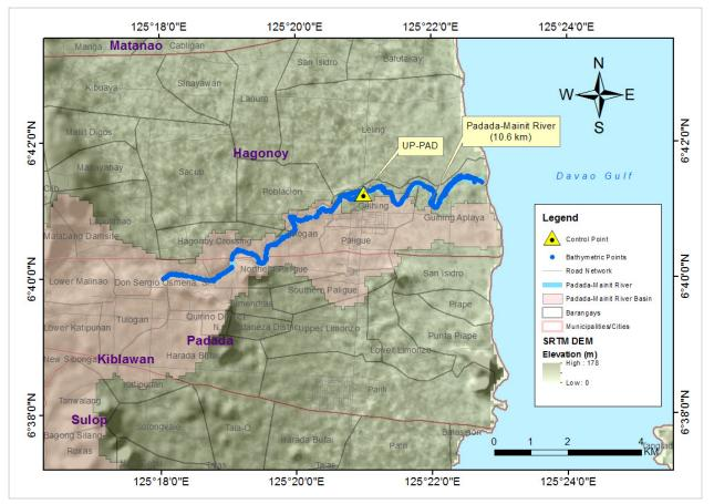
Figure 44. Bathymetric survey of Padada-Mainit River
