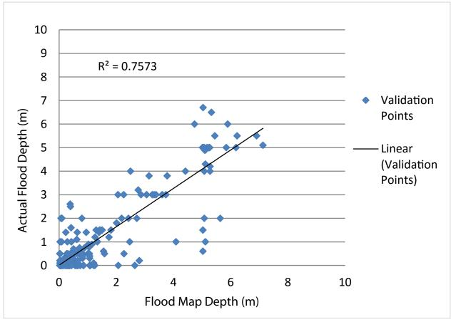
Figure 139. Flood Map Depth vs Actual Flood Depth for Padada
