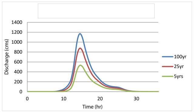
Figure 69. Digos Padada-Mainit river (9) generated discharge using 5-, 25-, and 100-year GenSan rainfall intensity-duration-frequency (RIDF) in HEC-HMS
