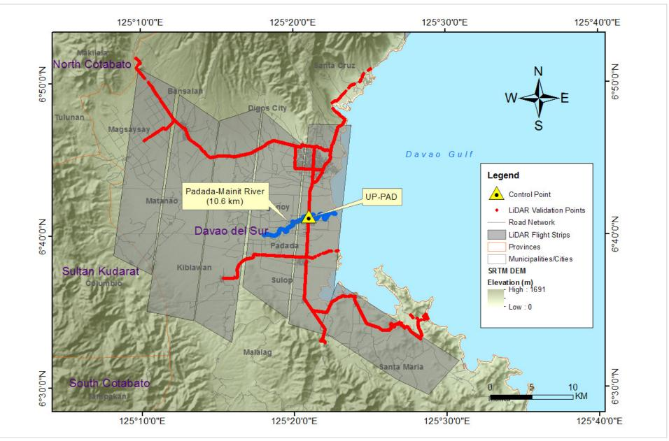
Figure 42. Validation points acquisition survey coverage for Padada-Mainit River
