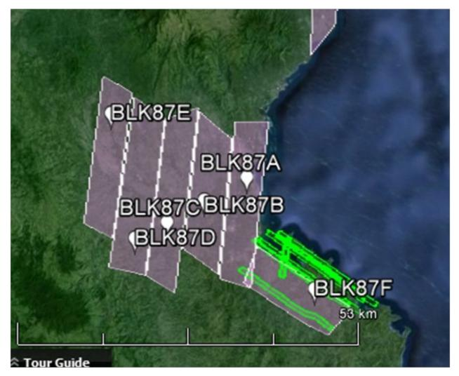
Flight No. : 7216GC Area: BLK87B, BLK87D, BLK87F Mission name: 2BLK87F218A Parameters: Altitude: 1000 m; Scan Frequency: 50 Hz Scan Angle: 20 deg; Overlap: 35 % Area covered: 139.714 km<sup>2</sup>
