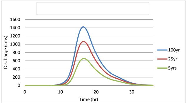
Figure 70. Digos Padada-Mainit river (10) generated discharge using 5-, 25-, and 100-year GenSan rainfall intensity-duration-frequency (RIDF) in HEC-HMS
