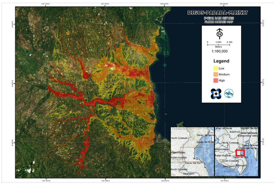
Figure 76. 5-year Flood Hazard Map for Padada Floodplain overlaid on Google Earth imagery
