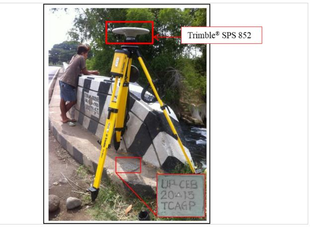
Figure 32. GNSS base receiver setup, Trimble® SPS 852 at UP-CEB on the right approach of Cebulan Bridge in Brgy Darong, Municipality of Santa Cruz, Davao Del Sur
