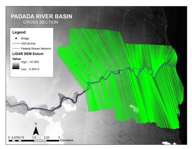
Figure 57. River cross-section of Padada River generated through Arcmap HEC GeoRAS tool
