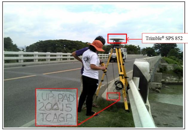
Figure 35. GNSS base receiver setup, Trimble® SPS 882 at UP-PAD, Padada Bridge, Brgy. Guihing, Municipality of Hagonoy, Davao del Sur
