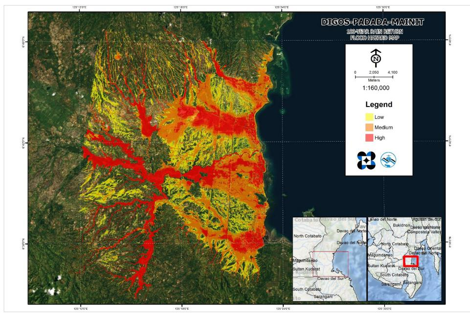
Figure 72. 100-year Flood Hazard Map for Padada Floodplain overlaid on Google Earth imagery
