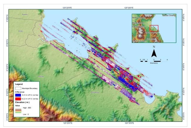
Figure 1.6.7 Elevation difference between flight lines
