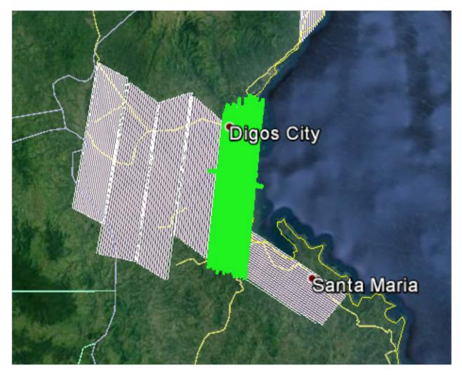
Flight No. : 7406GC Area: BLK87C Mission name: 2BLK87BC213A Parameters: Altitude: 1000 m; Scan Frequency: 50 Hz; Scan Angle: 20 deg; Overlap: 30 % Area covered: 193.272 km²
