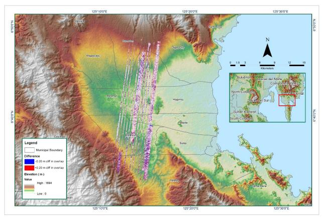
Figure 1.3.7 Elevation difference between flight lines
