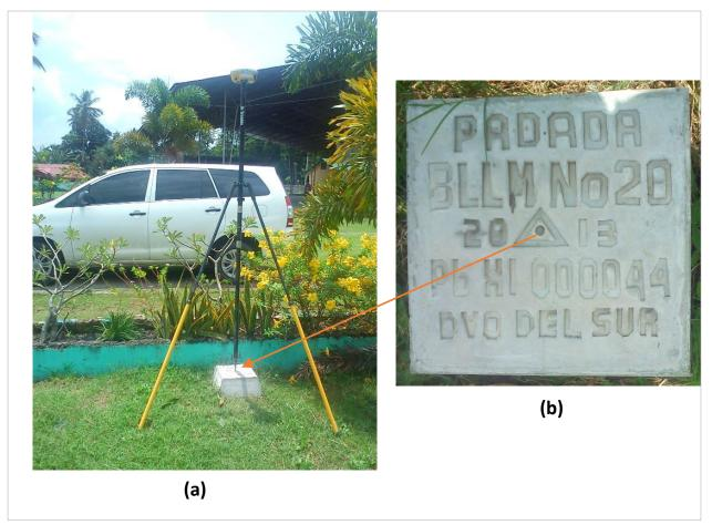
Figure 5. GPS set-up over BLLM-20 located inside Mariano Sarona Elementary School, inside the fence of the flagpole (a) and reference point BLLM-20 (b) as recovered by the field team.
