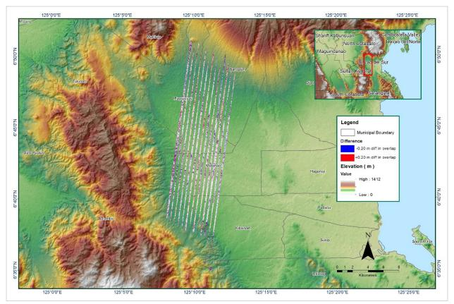
Figure 1.4.7 Elevation difference between flight lines
