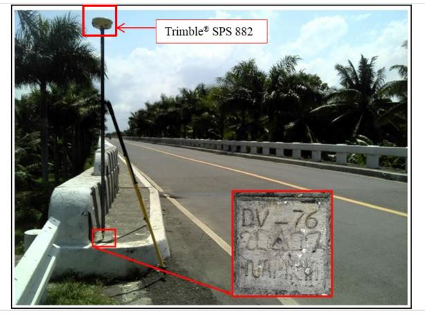
Figure 30. GNSS base receiver setup, Trimble® SPS 882 at DV-76 at the Gov. Miranda Bridge Approach, Brgy. Guadalupe, Municipality of Carmen, Davao Del Norte
