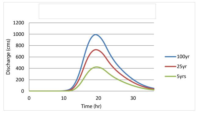
Figure 68. Digos Padada-Mainit river (8) generated discharge using 5-, 25-, and 100-year GenSan rainfall intensity-duration-frequency (RIDF) in HEC-HMS
