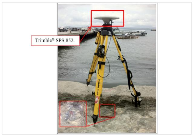
Figure 29. GNSS base receiver setup, Trimble® SPS 852 at DVS-1 at the east side of Pier, in Brgy. Leon Garcia Sr., Davao City, Davao Del Sur
