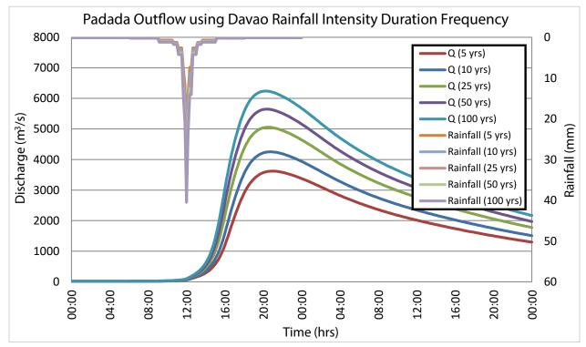
Figure 60. Outflow hydrograph at Padada Station generated using the Davao RIDF simulated in HEC-HMS.
