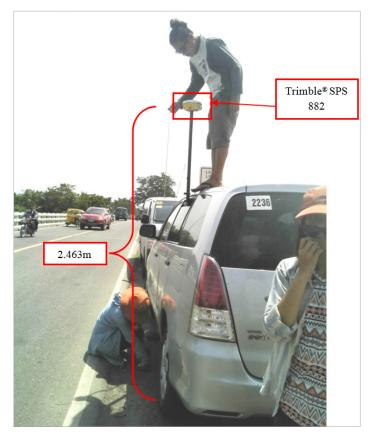
Figure 41. Validation points acquisition survey set-up for Davao del Sur.
