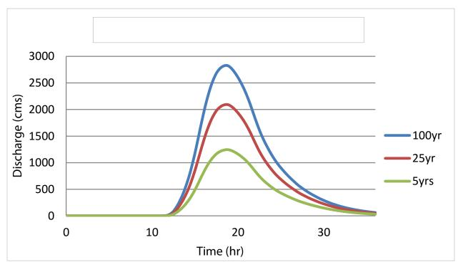
Figure 67. Digos Padada-Mainit river (7) generated discharge using 5-, 25-, and 100-year GenSan rainfall intensity-duration-frequency (RIDF) in HEC-HMS
