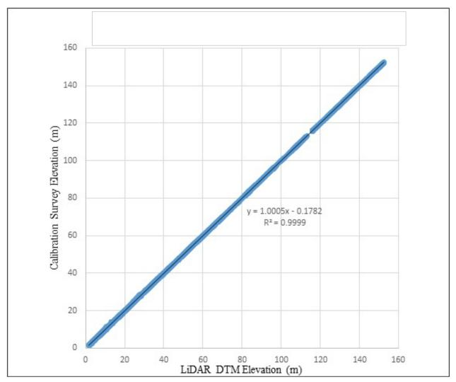
Figure 22. Correlation plot between calibration survey points and LiDAR data
