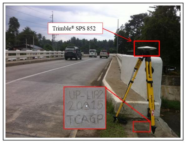
Figure 34. GNSS base receiver setup, Trimble® SPS 852 at UP-LIP2, on the right approach of Lipadas Bridge along National Highway in Brgy. Lizada, Toril District, Davao Del Sur
