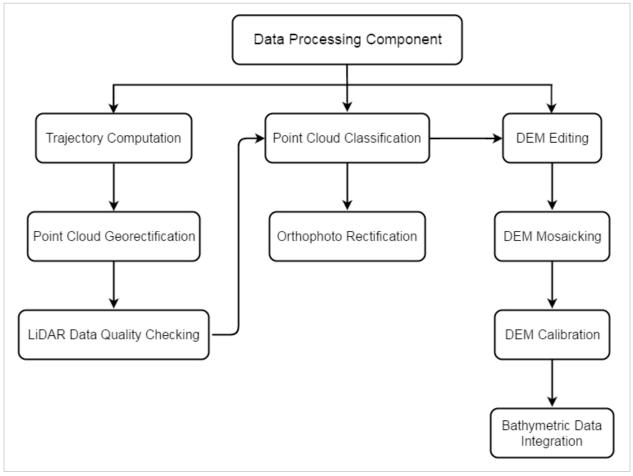
Figure 7. Schematic Diagram for Data Pre-Processing Component
