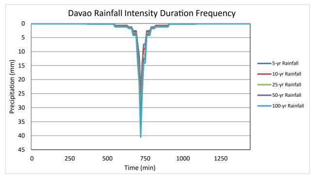
Figure 51. Synthetic storm generated for a 24-hr period rainfall for various return periods
