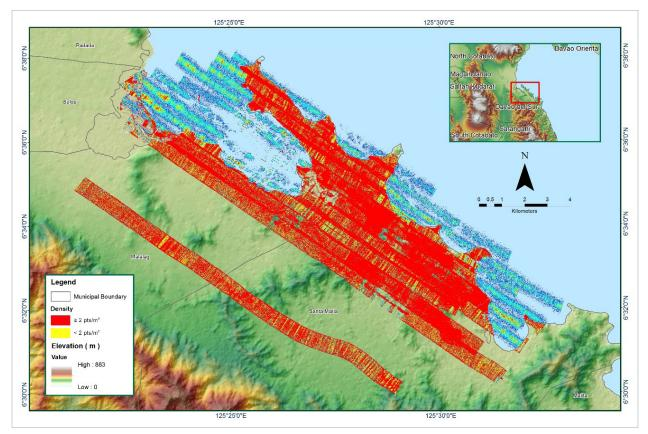
Figure 1.6.6 Density map of merged LiDAR data
