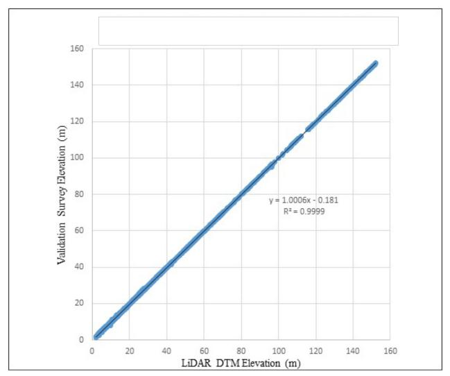
Figure 23. Correlation plot between validation survey points and LiDAR data.
