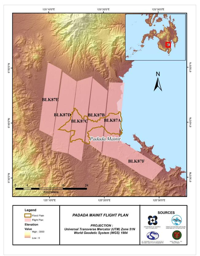
Figure 2. Flight plans used for Padada-Mainit floodplain.
