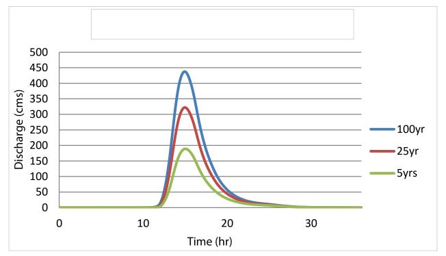
Figure 64. Digos Padada-Mainit river (4) generated discharge using 5-, 25-, and 100-year GenSan rainfall intensity-duration-frequency (RIDF) in HEC-HMS
