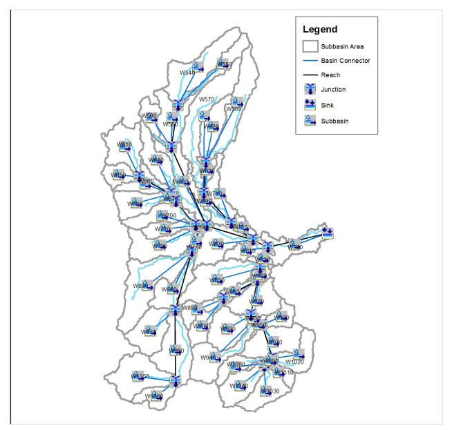
Figure 56. The Padada river basin model generated using HEC-HMS.
