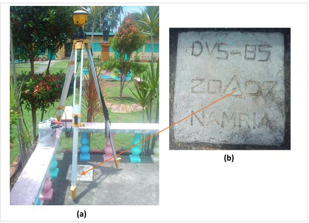
Figure 4. GPS set-up over DVS-85 located inside Mariano Sarona Elementary School, inside the fence of the flagpole (a) and NAMRIA reference point DVS-85 (b) as recovered by the field team.
