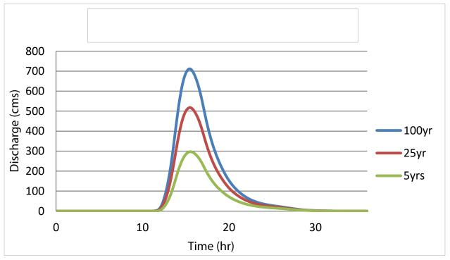
Figure 62. Digos Padada-Mainit river (2) generated discharge using 5-, 25-, and 100-year GenSan rainfall intensity-duration-frequency (RIDF) in HEC-HMS
