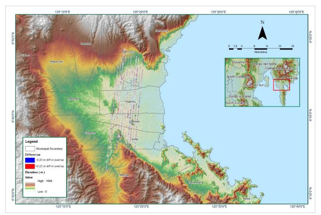
Figure 1.2.7 Elevation difference between flight lines
