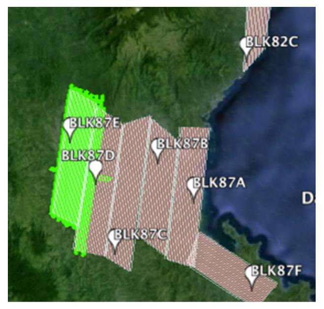
Flight No. : 7412GC Area: BLK87B Mission name: 2BLK87CSD216A Parameters: Altitude: 1000 m; Scan Frequency: 50 Hz Scan Angle: 20 deg; Overlap: 35 % Area covered: 70.780 km<sup>2</sup>
