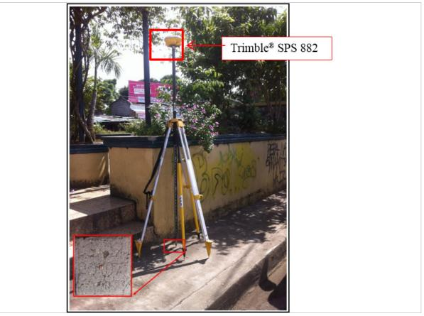
Figure 31. GNSS base receiver setup, Trimble® SPS 882 at DS-09 located at stair of Nograles Park along Mac Arthur Highway, in Brgy. Talomo, Davao City, Davao Del Sur
